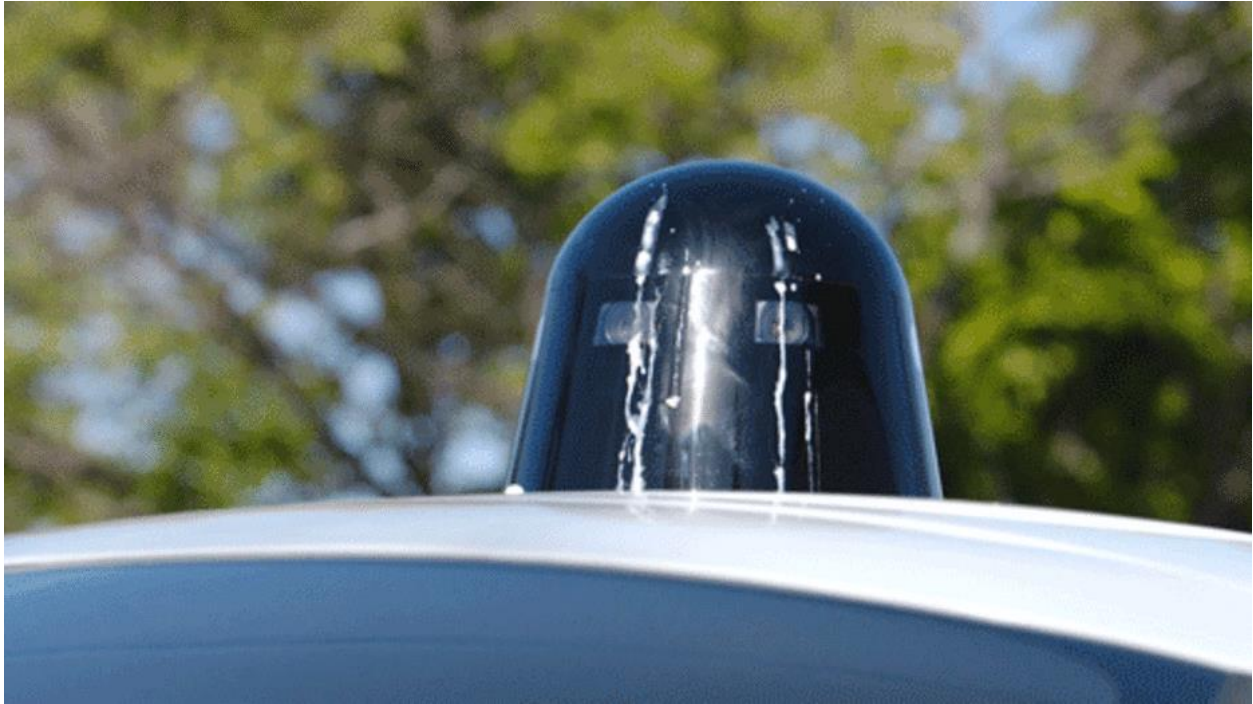
A waymo Lidar unit (during Lidar wiping testing)
