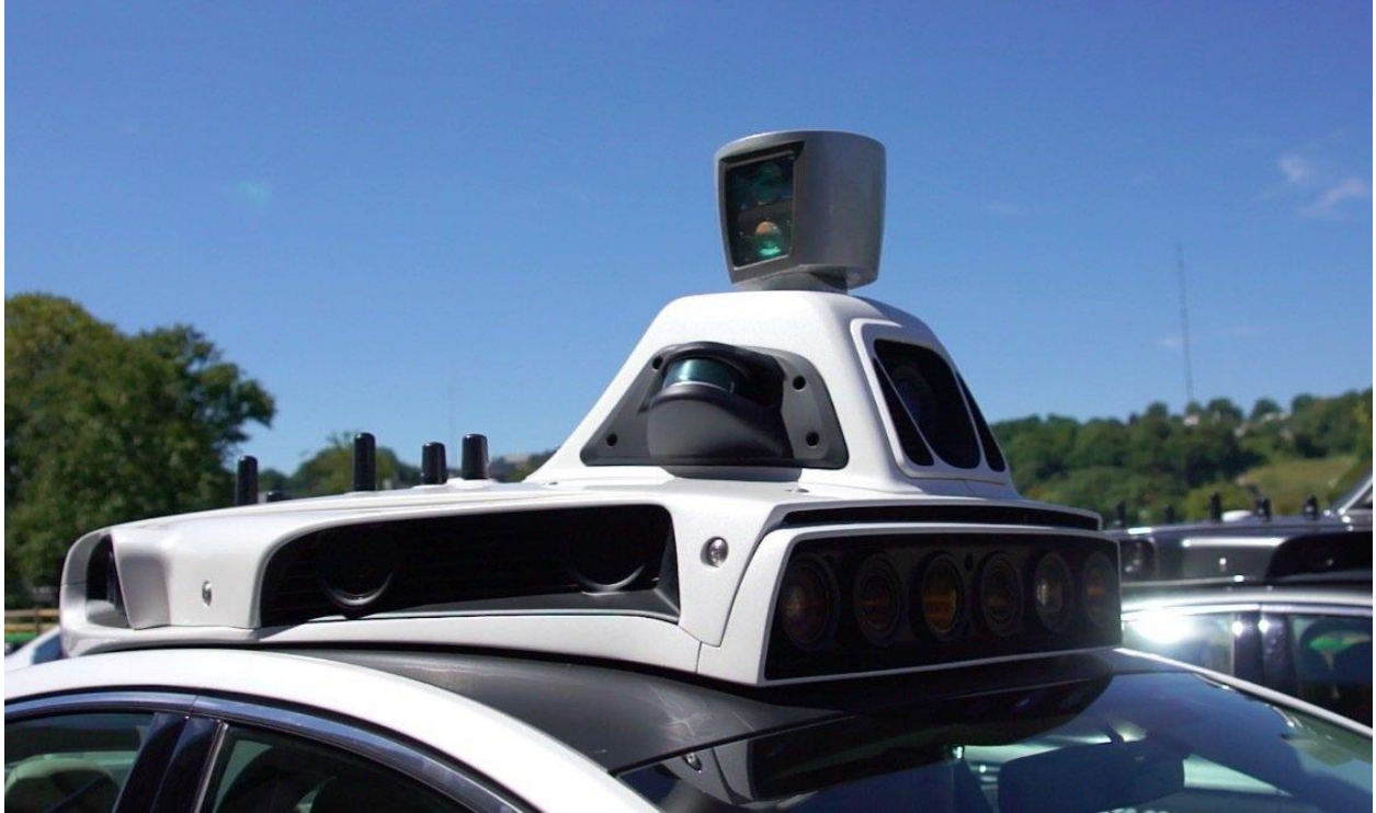
Older Uber Lidar sensor rack (Ford Fusion) [ http://media.pennlive.com/life/photo/self-driving-uber-ff4637c53b737463.jpg ]
