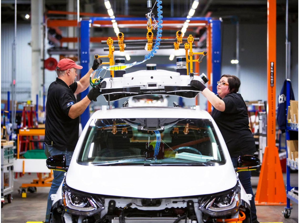
Workers at the Orion assembly plant adding the roof sensors for a Cruise self-driving car [ https://www.wired.com/story/gm-softbank-investment-tesla-braking-news-roundup/ ]
