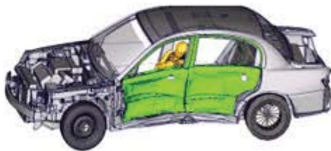
Side frame deformation
