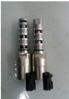
Note: Different OCVs for intake and exhaust (left for intake and right for exhaust)
