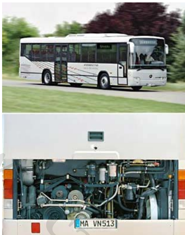
Mercedes-Benz Conecto H with six-cylinder OM ۴۵۷ hLA Euro ۳ diesel engine
