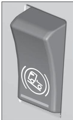
disengaged when the starter key is turned to the 0 position. When the engine is started the function is always disengaged.
