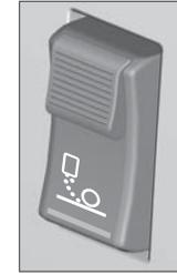
Anti-slip device, sand aggregate
