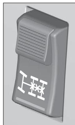
Differential lock between the axles.
