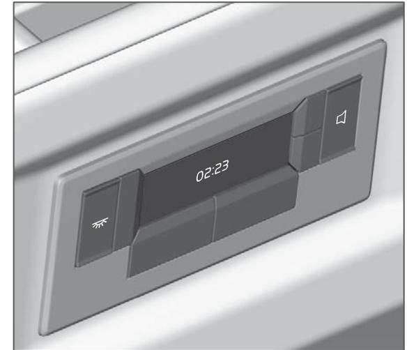
The rear control panel with display is located above the bed area on the rear cab wall.
