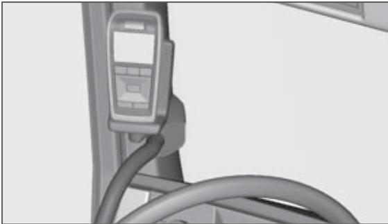
*The work remote control in its charging station*
