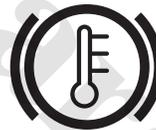
*Warning symbol for high brake temperature.*
