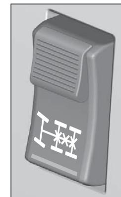
Centre position, the differential lock between the axles is engaged. The symbol in the instrument illuminates.
