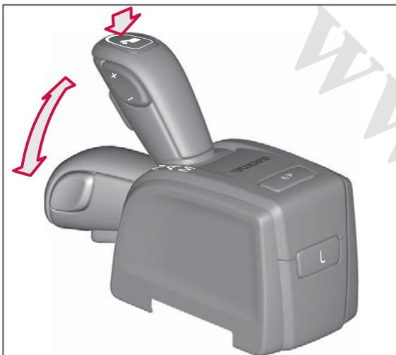
The gear shift lever can be tilted to horizontal position in order to be unobstructive and allow easy movement between the driver seat and other parts of the cab.
