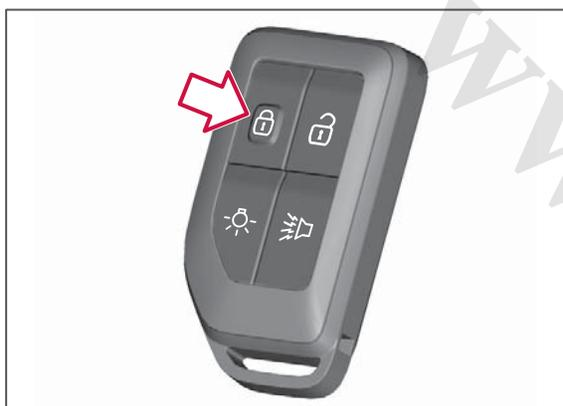
Lock the doors by pressing the LOCK button. The direction indicators illuminate.
