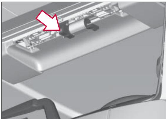
*Emergency operation of the roof hatch*
