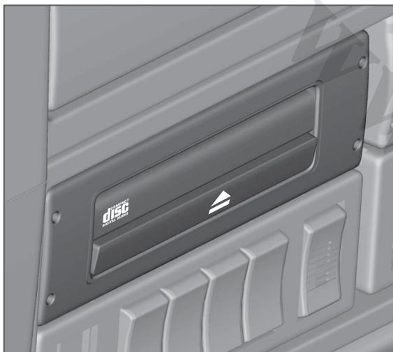
The CD player is fitted in the panel above the windscreen on the driver's side and consists of an opening for the disc and a button that ejects the disc.
