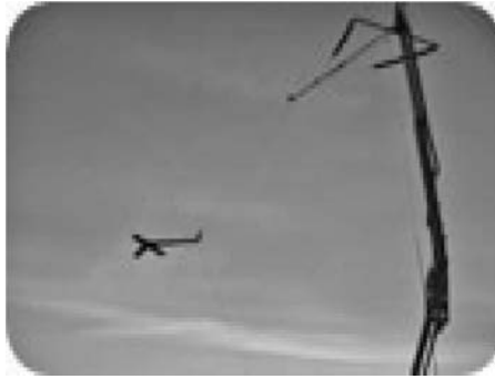
FIGURE 5.4 Insitu ScanEagle recovery.
