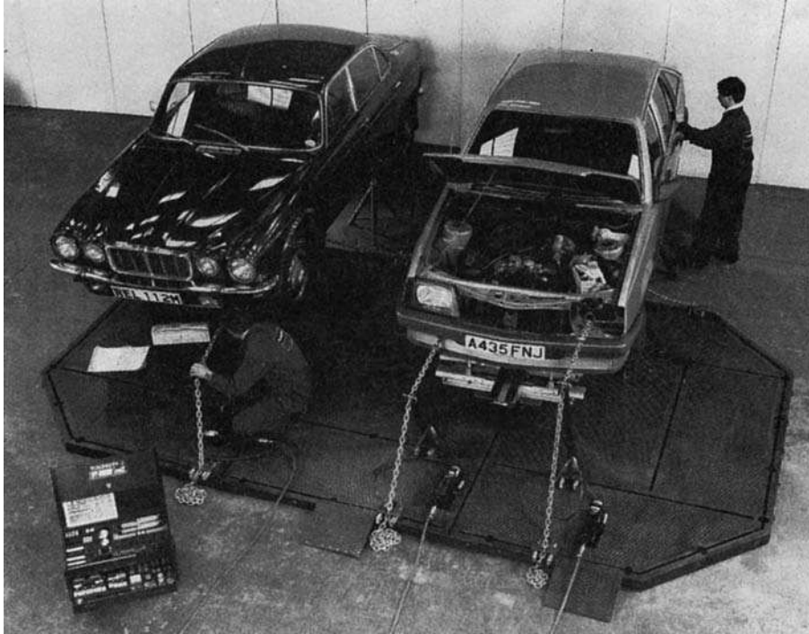
Figure 14.9 Korek system straightening two cars at the same time ( Blackhawk Automotive Ltd )
