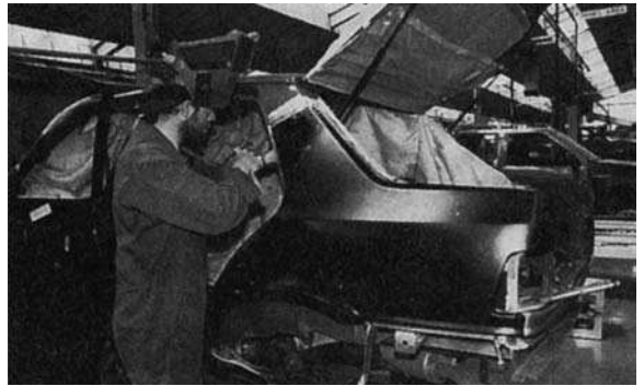
Figure 14.98 Alignment of new panel sections ( Motor Insurance Repair Research Centre )
