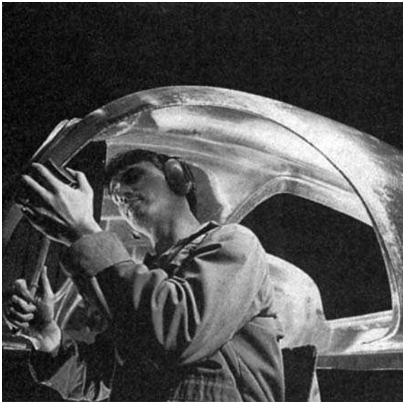
Figure 13.16 Planishing a hand-made panel (Autokraft Ltd)
