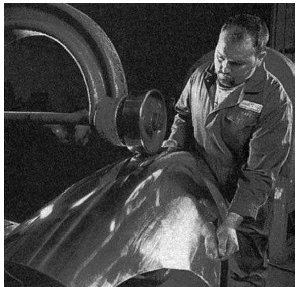
Figure 13.9 Sports car panel being shaped by wheeling ( Autokraft Ltd )
