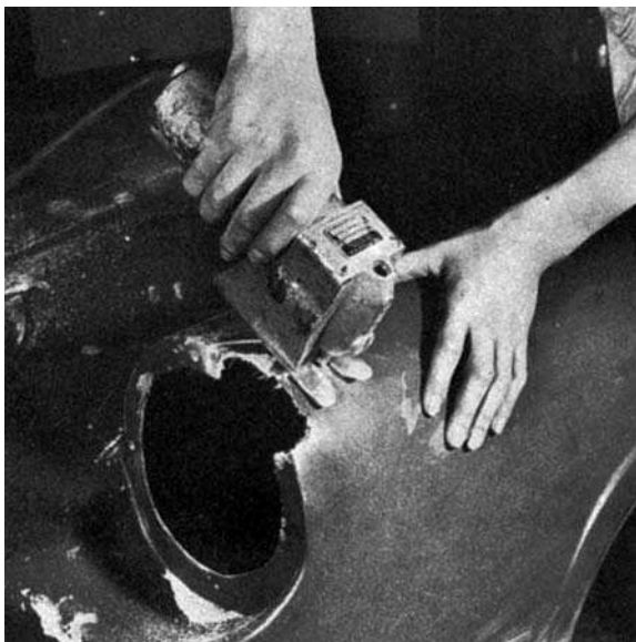
Figure 16.36 Removing damaged laminate
