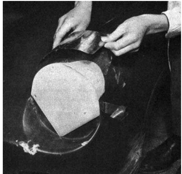
Figure 16.41 Removing temporary moulds
