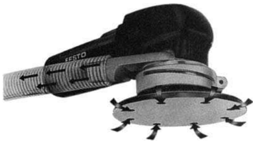
Figure 3.61 Rotex sander with full dust extraction ( Minden Industrial Ltd )
