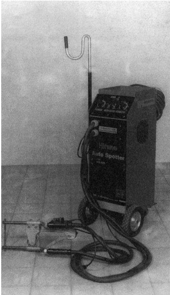
Figure 10.21 Single-sided and double-sided spot welding equipment (Stanners Ltd)
