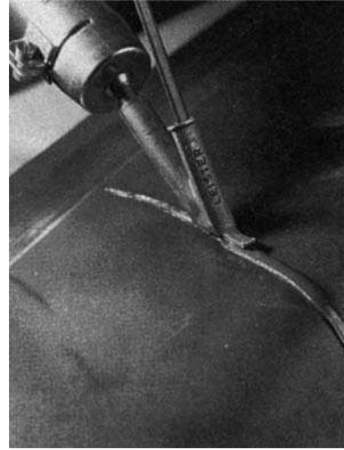
Figure 14.122 Main plastic welding operation (Welwyn Tool Co. Ltd)
