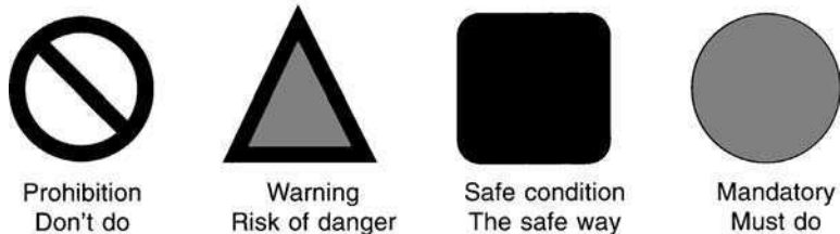
Figure 2.14 Standard safety signs
