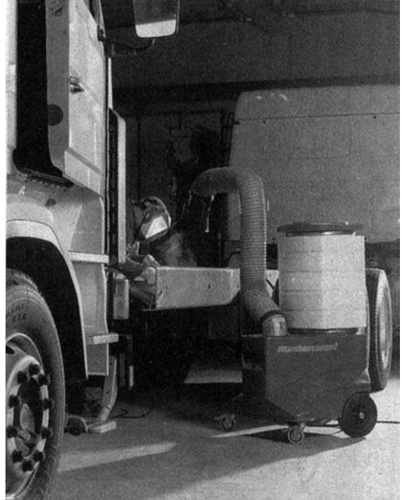
Figure 15.10 Portable fume and smoke extraction system ( Nederman Ltd )
