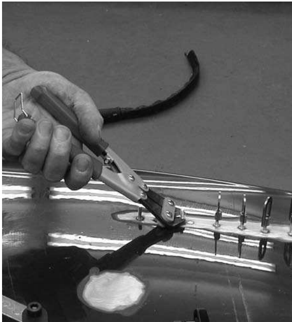
Figure 13.74 Snip-off the studs (Courtesy of POWER-TEC®)
