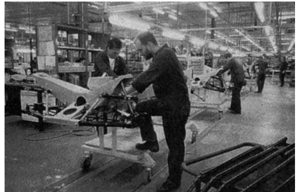
Figure 16.30 First stages in building up chassis details on the Lotus Elan ( Lotus Engineering )
