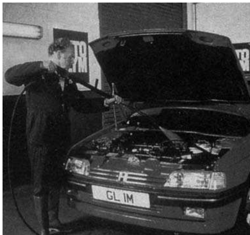
Figure 14.129 Pressure washing engine compartment ( Autoglym )
