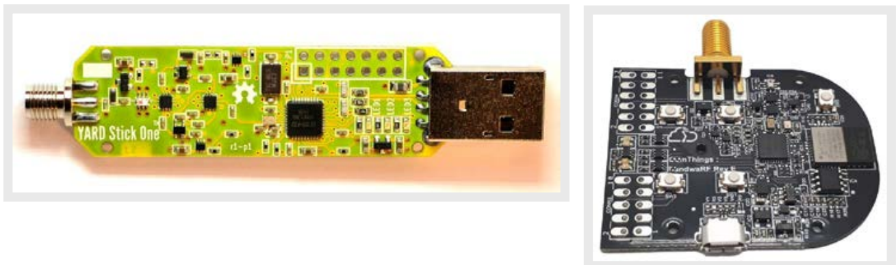
Figure 46. Yard Stick One dongle (left) 65 and PandwaRF device (right) 66
