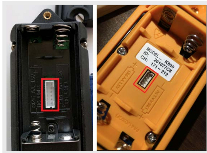
Figure 18. Programming interfaces on two of the units that we analyzed
