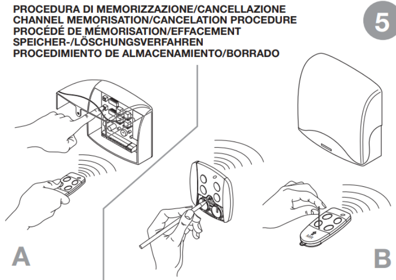
Figure 3. Instructions for the DOR procedure with a hidden button 3
