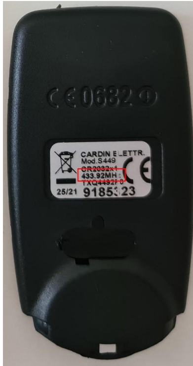
Figure 7. Our test remote's ID and the precise frequency it uses
