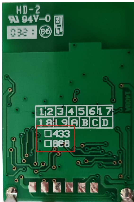
Figure 6. The back of the PCB with information about the possible bands
