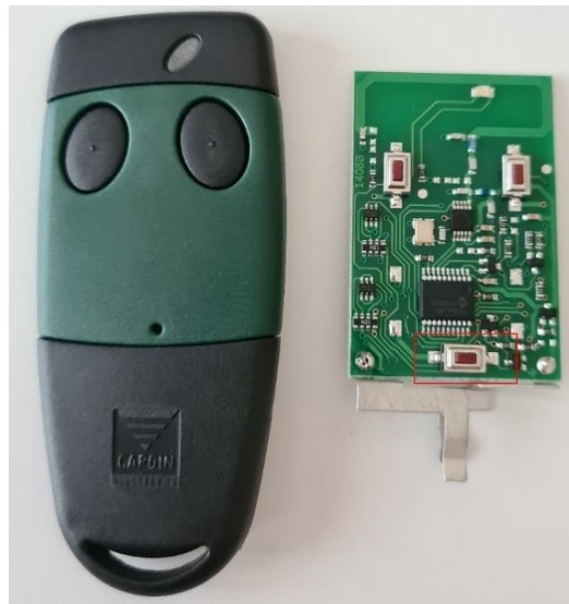
Figure 4. Image of the disassembled remote and the DOR's "hidden" button (in the red box)
