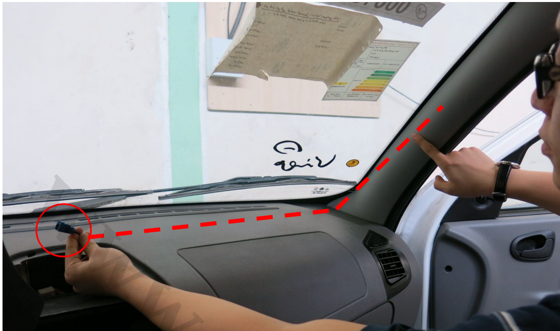
12. GPS cable through the Dash board .
