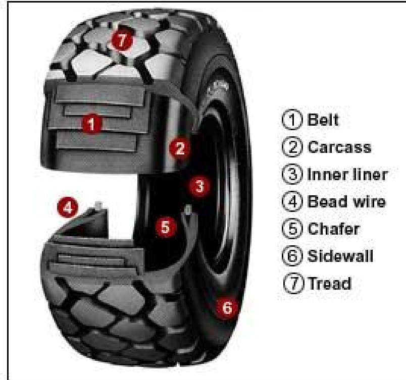
Structural Diagram of Off-the-Road Radial Tires
