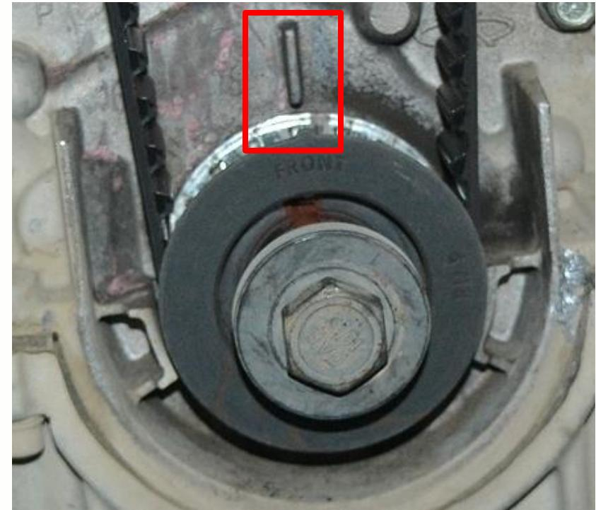
Alignment mark of crankshaft timing gear
