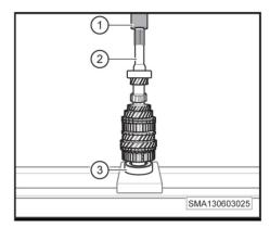
19. Install the 5th gear synchronizer cotter (-1-).20. Install the 3rd and 4th gear synchronizer cotter (-2-).
