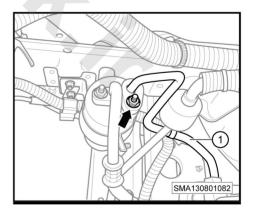
10. Unscrew the coupling nut between the reservoir dryer and the dryer-condenser pipe (-arrow-).
