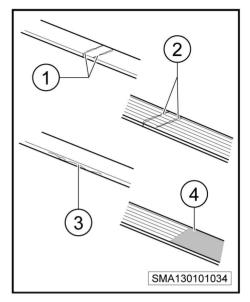
Checking the power steering belt
