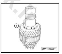
**10**. Install the steel balls (-1-) to the input shaft.
