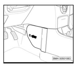
4. Remove the front console trim (-1-).5. Unscrew the front fixing bolts of the console (-arrow-).
