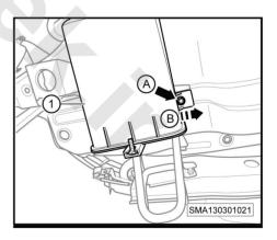
**3**. Unscrew the bolt (-arrow A-), loosen the body clip in the (-arrow B-) direction, and take out the activated carbon canister (-1-).
