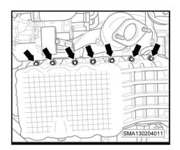
7. Unscrew the timing belt side oil pan fixing bolts (-arrow-).
