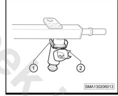
11. Loosen the holder (-1-) and pull out the injector (-2-).
