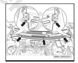
4. Remove the upper seal of the wiper cover and unscrew the wiper cover fixing bolts (-arrow-).
