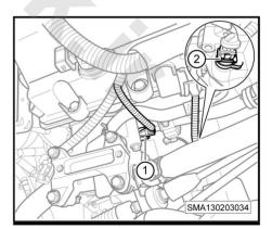
**16**. Disconnect the electronic throttle connector (-1-).
