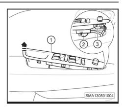
6. Remove the power window main switch (-1-).
