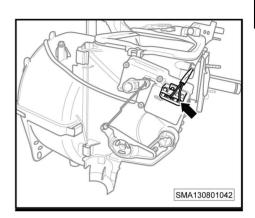
Remove the inner-outer circulation servo motor connecting rod (-1-).
