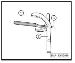
**9**. Separate the 1st and 2nd gear shift fork (-1-) from the shift shaft (-2-).
