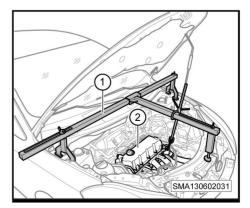
**14**. Fix the engine assembly (-2-) with the engine hanger (-1-).
