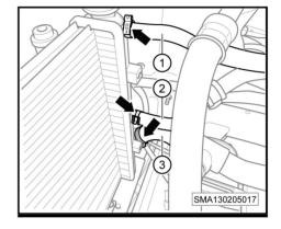
**4**. Loosen the clamp (-arrow-), pull out the hose (-1-) and remove the radiator.
