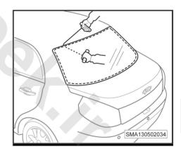
**3**. Remove the sealant residue (-2-) on the frame with a scraper (-1-).
