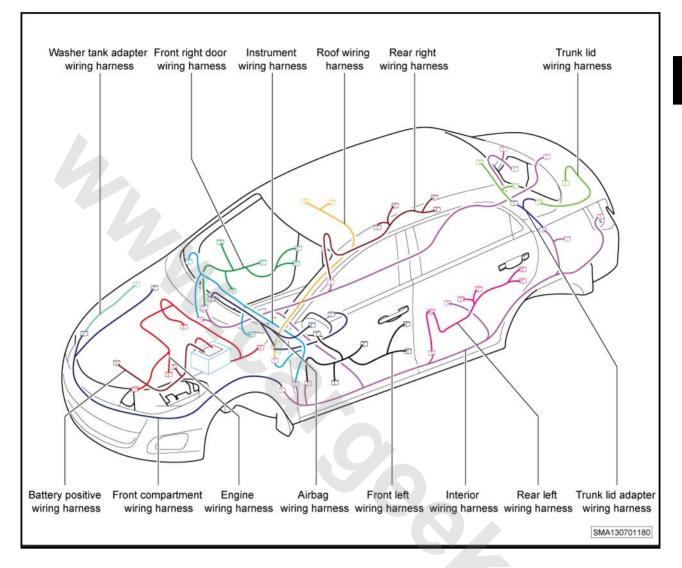
3.2.2 Front compartment wiring harness layout
