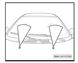
2. If the spray is normal while the nozzle angle is different, please use a pin to turn the adjustment device (-arrow-) until the nozzle is adjusted towards
