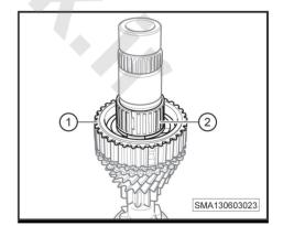
17. Remove the 4th speed gear (-1-).
