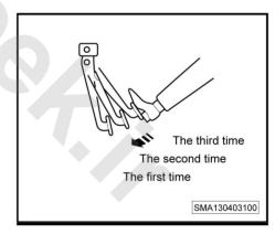
2. When the engine is running, press the brake pedal and then switch off the engine. If the pedal height remains unchanged within 30 seconds, it indicates the vacuum booster has sound airtightness. If it continues to sink, it indicates the vacuum booster has poor airtightness and needs repairing.
