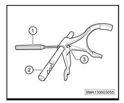
**6**. Knock out the dowel pin (-3-) from the shift shaft (-2-) with the punch (-1-).
