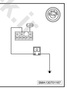
Replace the anti-theft control module, carry out the function test again, and read the fault code to verify if it exists or not.
