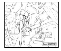
4. Lift the carpet. The pedal height equals the distance from the cabin floor to the pedal center point (-1-).
