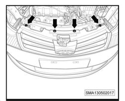
2. Disengage the lower fixing clips (-arrow-) and remove the front air intake grid (-1-).
