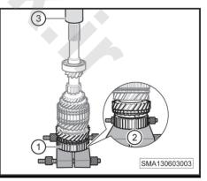
**15**. Press the 5th gear synchronizing gear (-1-) into the input shaft with the hydraulic press (-3-).
