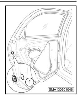
**3**. Disengage the door lock lever (-1-) in the (-arrow-) direction and disconnect the cable (-2-).
