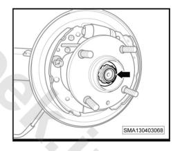
3. Pull out the rear wheel hub (-1-) with the puller.
