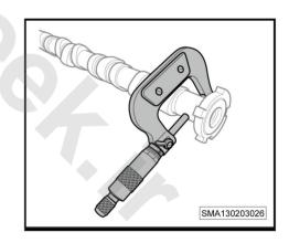
2. As shown in the figure, measure the camshaft lifting height with an outer diameter micrometer. The measured lifting heights of the intake and exhaust camshafts shall be 5.09 mm and 5.34 mm respectively.
