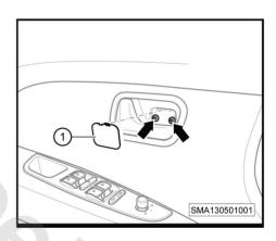
**3**. Lever out the power window main switch lid (-1-) and unscrew the fixing screw of the power window main switch (-arrow-).
