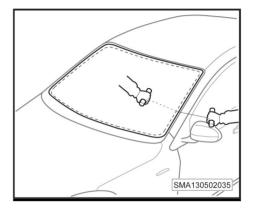
**4**. Remove the sealant residue (-2-) on the frame with a scraper (-1-).
