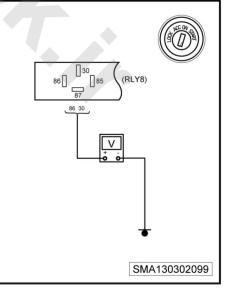
7. Pull out the main relay (RLY8) and check if the relay is normal.
