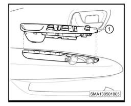
**7**. Remove the triangle block (-1-) inside the driver's side door.
