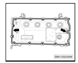
4. Install the cylinder head cover gasket into the groove of the cylinder head cover, and then apply sealant on the connection area between the front end of the cylinder head cover and the bearing cap and the area between the two rear bolts, i.e. the grey part of the gasket (-arrow-).
