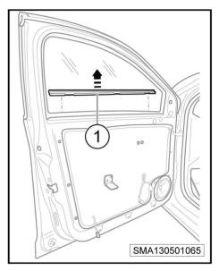
4. Remove the front outer door seal (-1-) in the (-arrow-) direction.
