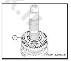
9. Fix the 3rd gear driven gear (-2-) with the special tool
