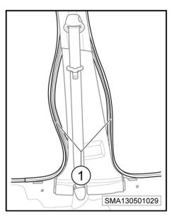
7. Move away the seat belt (-1-) and remove the B pillar lower trim (-2-).
