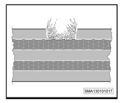
• **b**Rupture of seat belt edge fabric.
