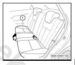
Unscrew the lower fixing bolts of the rear seat belt (-arrow-).
