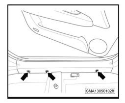
3. Remove the front door sill guard plate (-1-).
