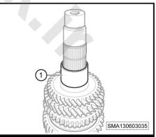
8. Install the 2nd gear driven gear (-1-).
