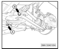
4. Unscrew the ball joint fixing bolts (-arrow-) of the front lower control arm (-1-) to remove the front lower
