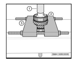
13. Remove the 5th gear needle bearing (-1-).
