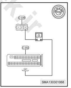
Remove the vehicle speed sensor, connect its connector and rotate the signal wheel of the speed sensor manually to check if the signal voltage at the
