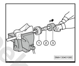
**3**. Make a mark (-1-) at the same height of the axle shaft (-2-) and the outer CV joint edge (-3-) to check with ease whether they are properly installed.
