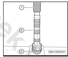
2. Install the 1st gear needle bearing (-1-).
