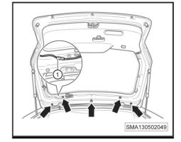
Remove the fixing bolts of the rear fender assembly (-1-).
