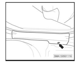
4. Remove the rear door sill guard plate (-1-).
