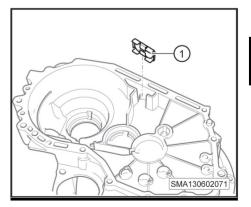
**3**. Install the input shaft oil seal (-2-) to the transaxle housing (-3-) with the tool (-1-).
