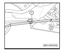
8. Unscrew the left cable fixing nuts of the parking brake (-arrow-).
