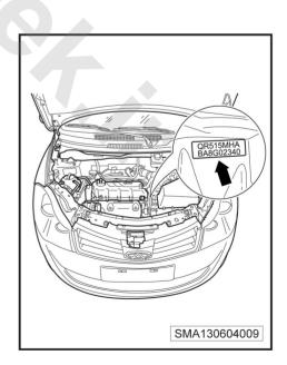
For transaxle QR515, the number consists of two parts: the transaxle type and the identification number.
