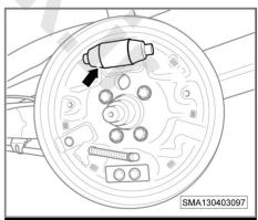
3. Unscrew the exhaust port bolt (-arrow-).
