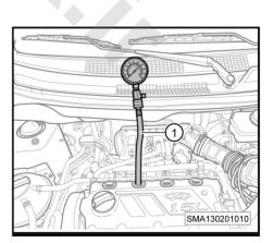
with the same method, taking the mean value among them. The standard cylinder compression pressure should be 12±2 bar.
