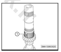
**20**. Fix the 3rd gear driving gear (-2-) with the special tool (-1-).
