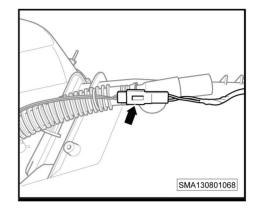
5. Remove the interior temperature sensor (-1-).
