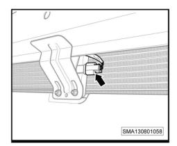
5. Remove the exterior temperature sensor (-1-).
