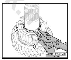
4. Install the 1st gear synchronizing ring assembly (-1-).
