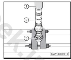
2. Install the 3rd gear needle bearing (-1-).
