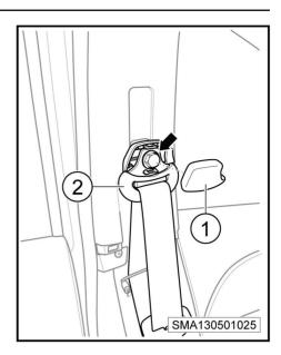
**10**. Unscrew the fixing screws of the B pillar upper trim (-arrow).
