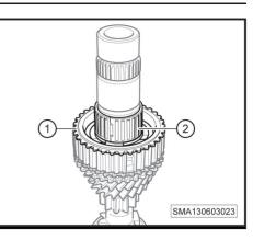
**9**. Install the 4th gear driving gear (-1-).
