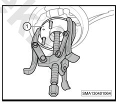
4. Pull out the rear wheel hub (-1-) with the puller.
