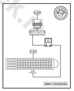
Replace the ECM control module, carry out the function test again, and read the fault code to verify if it exists or not.
