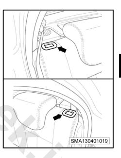
**3**. Remove the upper rubber cover of the rear shock absorber (-arrow-).
