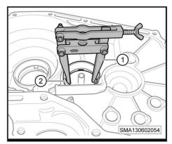
4. Lever out the axle shaft oil seal (-2-) with the slotted screwdriver (-1-).
