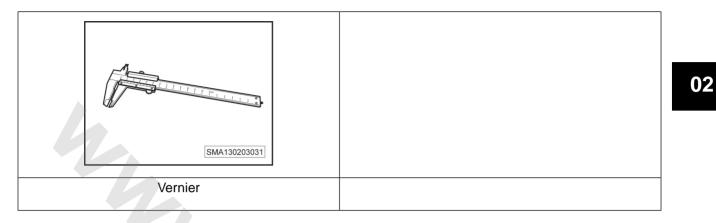
As shown in the figure, measure the free height and the pretension height of the valve spring with a vernier. The measured value of free height shall be 47.7 mm, and the installation height shall be 41 mm under the pretension of 260±11 N.
