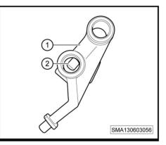
5. Remove the lock pin (-2-) from the 5th gear fork (-1-).
