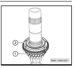
4. Install the 3rd and 4th gear synchronizing gear (-1-).
