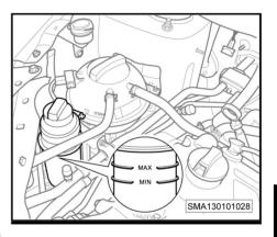
5. When the power steering fluid level is higher than the MAX (maximum) mark, please discharge the power steering fluid. When the power steering fluid level is lower than the MIN (minimum) mark, please check the steering system pipe for leakage. If there is, repair it.
