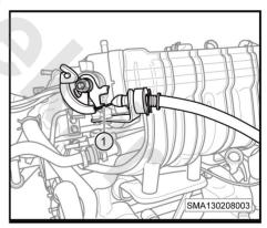
**6**. Loosen the mechanical throttle cable (-1-) and disconnect the cable from the bracket.
