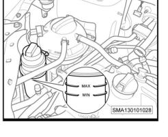
3. Switch off the engine and check the power steering fluid level. Add some if necessary.
