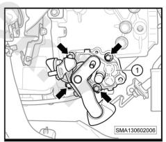
5. Unscrew the fixing bolts (-arrow-).
