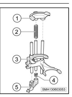
4. Remove the lock pin (-2-) from the reverse gear fork (-1-).
