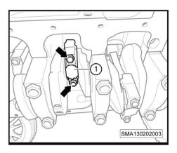
**2**. As shown in the figure, using soft materials (such as wooden or rubber hammer handle (-1-)), push out the piston component (-2-).
