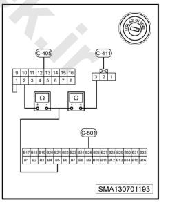
6. Check if the ground line between the the central door lock key switch connector and the central door lock switch is normal.
