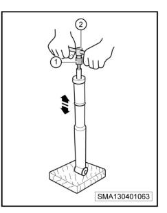
3. Check for oil leakage, abnormal noise and jamming.
