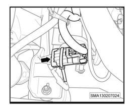
4. Unscrew the oxygen sensor (-1-).
