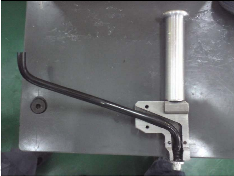
Fig. 16-1 Put vent pipe into the special tool.
