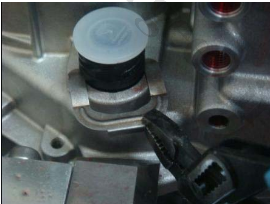
Fig. 15-1: Remove the fastener from main joint
