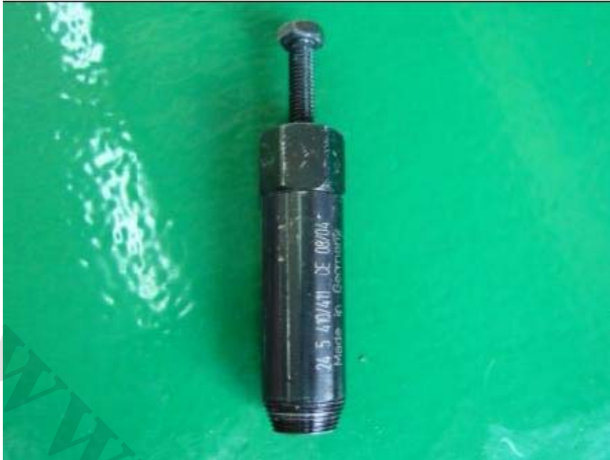
Dismantling tool of selector shaft oil seal (drawing 480127)
