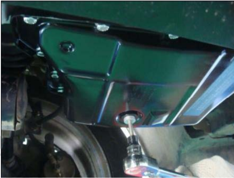
Fig. 9-1 Remove oil drain screw plug
