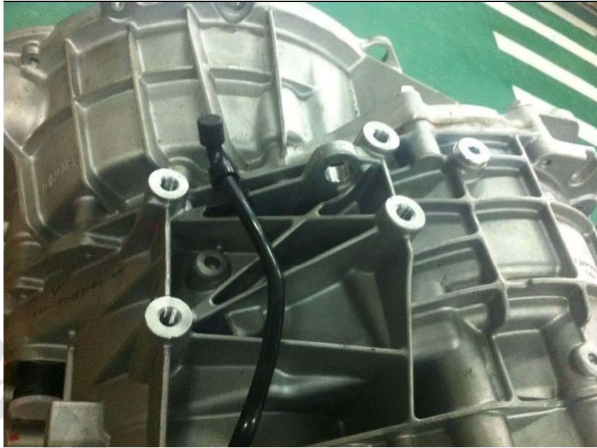
Fig. 16-3 Install the fastener and vent pipe cap
