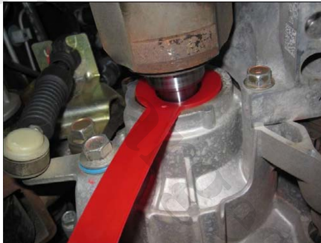
Fig. 1-4: 2cm between axle shaft and tool 480145
