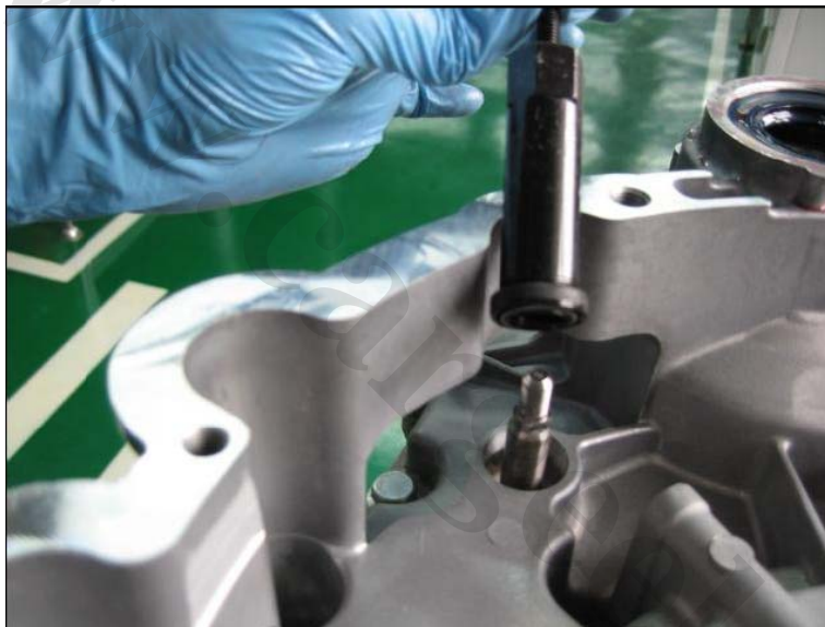
Fig. 4-4: Take out oil seal
