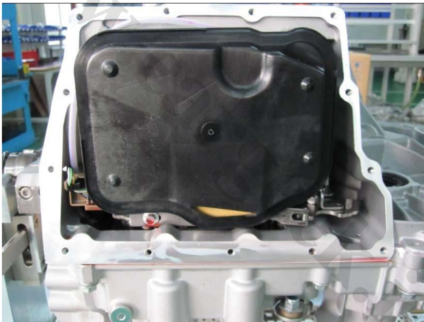
Fig. 10-2: Install the filter in place
