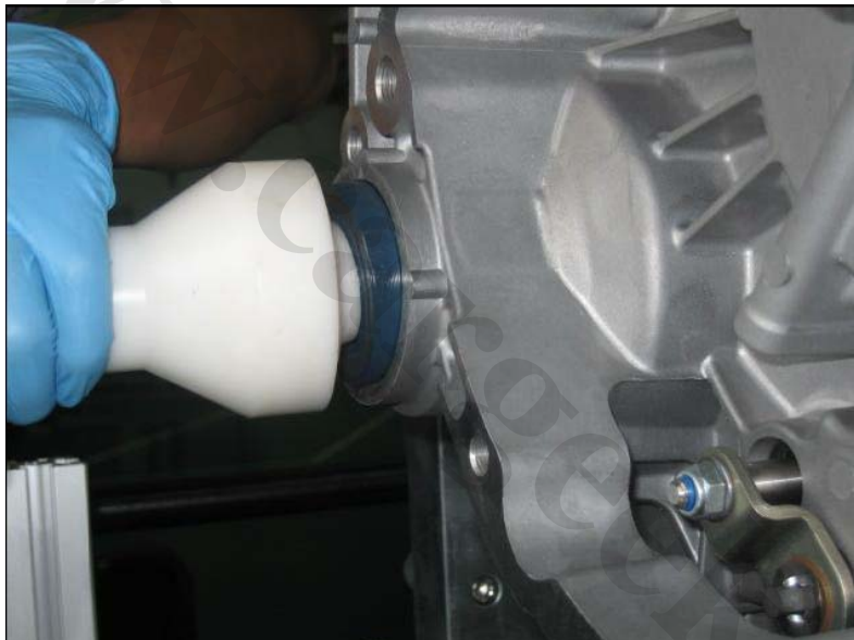
Fig. 2-2 Install oil seal with special tool
