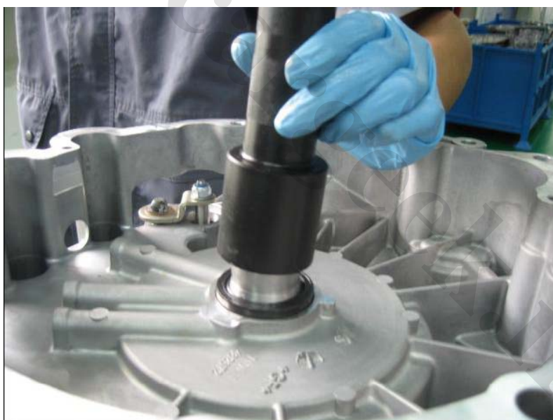
Fig. 3-4: Install oil seal by special tool (480130)
