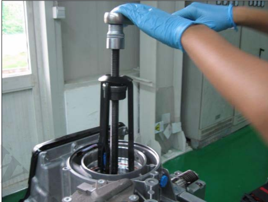
Fig. 7-5: Screw out middle bolt to pull out the bearing
