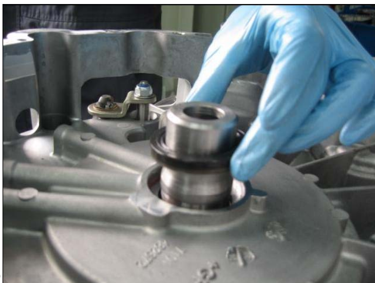
Fig. 3-3: Press oil seal down
