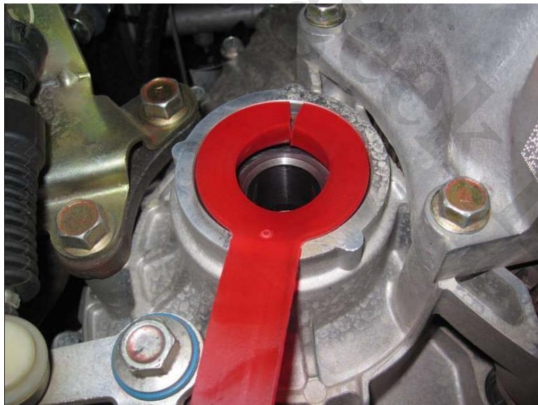
Fig. 1-2: Install axle shaft tool 480145
