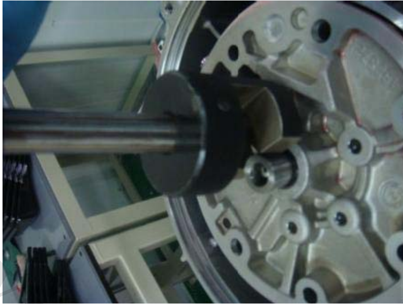
Fig. 6-1: Remove six bolts and install special tool
