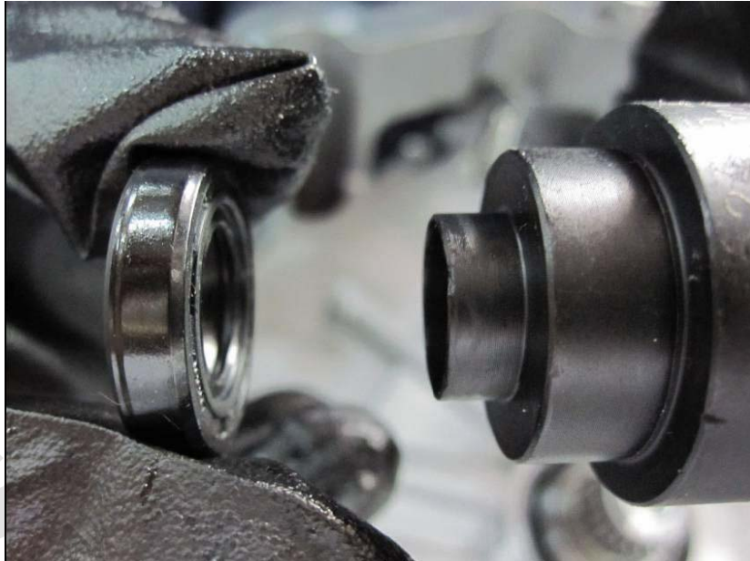
Fig. 4-5: Install oil seal on the punch (480125)
