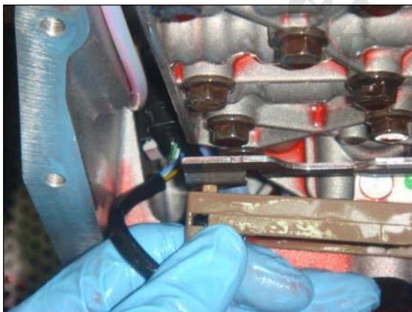
Fig. 11-2: Press down the sensor and take it out
