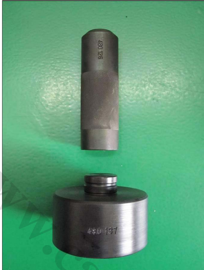
Drive cone wheel bearing punch (drawing 480137 + 480126)
