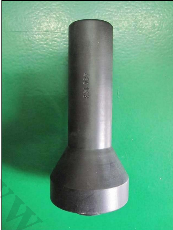
Differential oil seal punch (drawing 480143)
