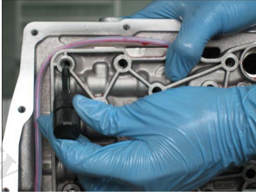
Fig. 12-6: Special tool (23K002-099-84312) fixes hydraulic control block
