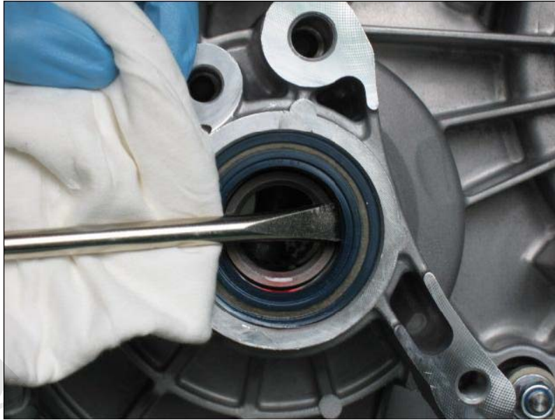
Fig. 2-1: Remove oil seal
