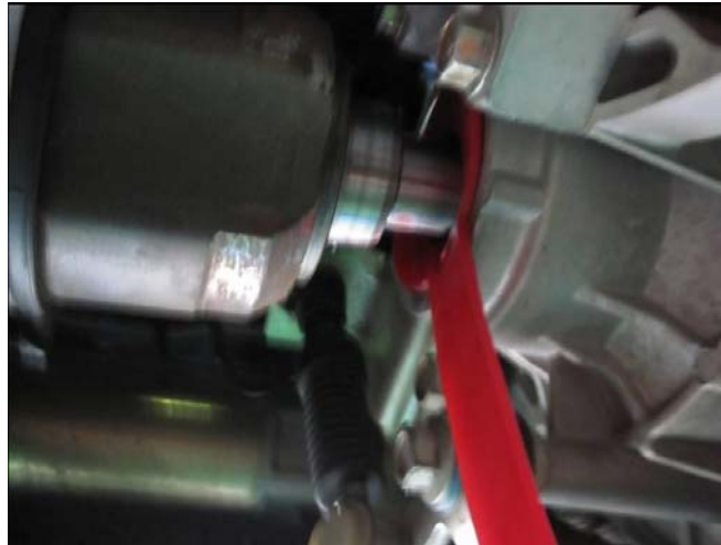
Fig. 1-3: Axle shaft is 4cm deep in the transmission
