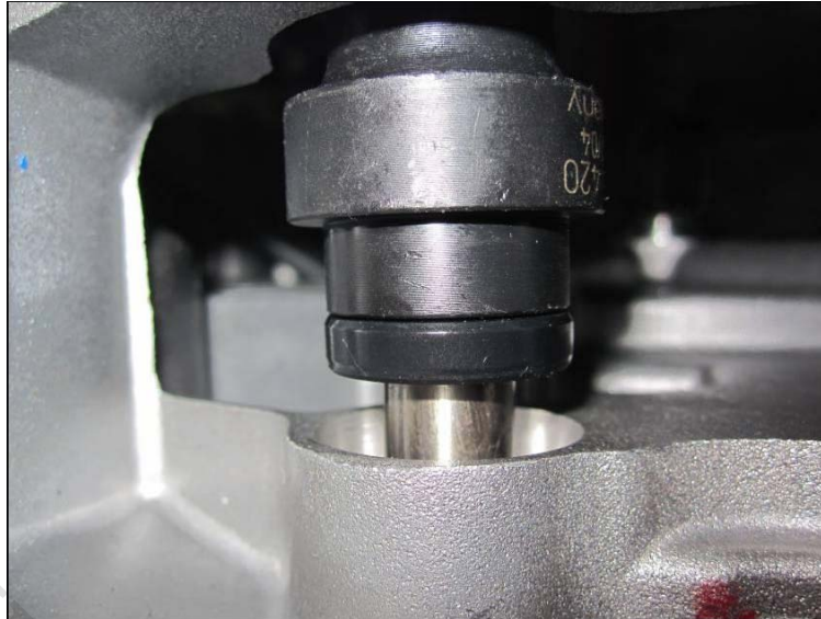
Fig. 4-7: Knock the punch (480125) in place by hammer
