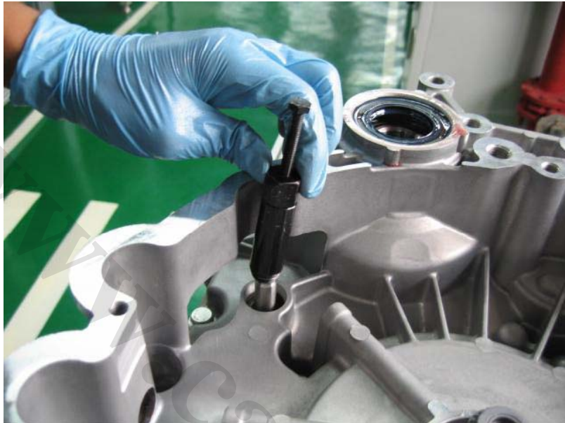
Fig. 4-1: Put special tool (480127) on selector shaft
