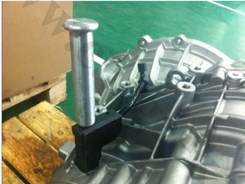
Fig. 16-2: Knock the tool with vent pipe into the transmission
