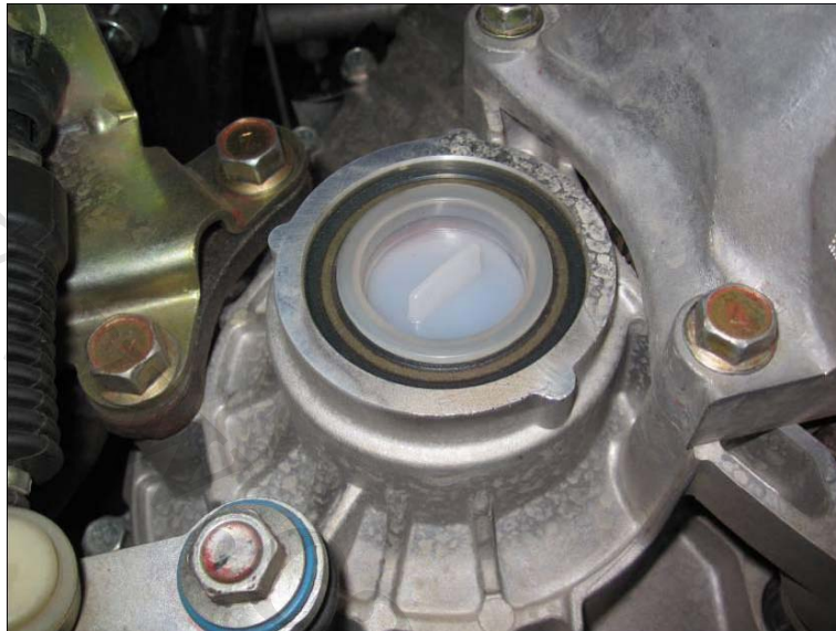
Fig. 1-1: Transmission oil seal protection cover
