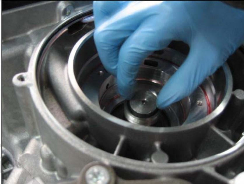
Fig. 7-3: Put special tool on the shaft (drive cone wheel plug T00222)
