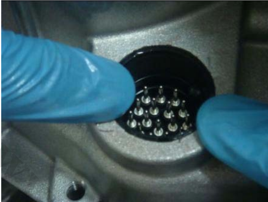
Fig. 15-2: Press main joint into the transmission
