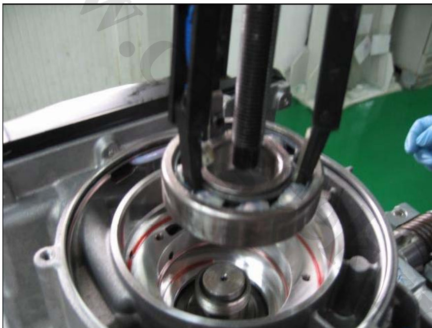
Fig. 7-6: Remove drive cone wheel shaft bearing
