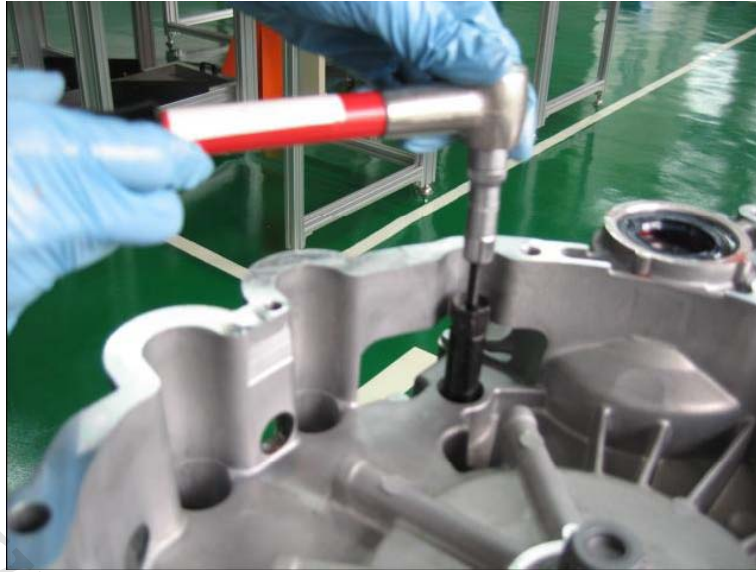
Fig. 4-3: Screw out small bolt to pull out oil seal
