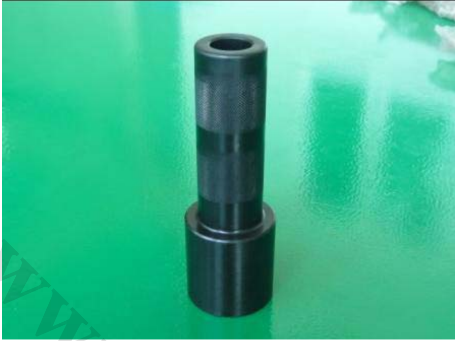
Input shaft oil seal punch (drawing 480130)
