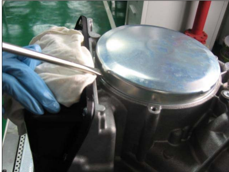
Fig. 5-1: Dismantle drive cone wheel shaft end cover
