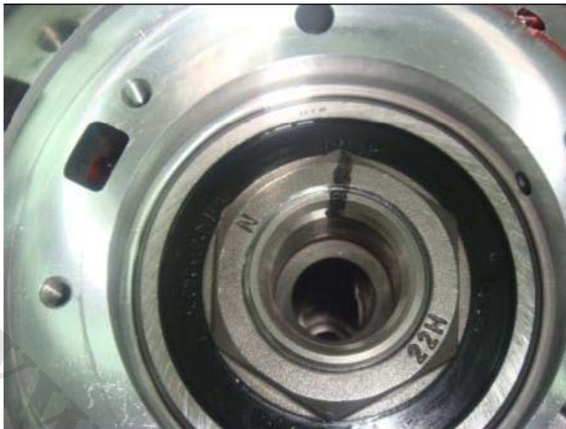
Fig. 7-1: Make marks on the shaft and nut
