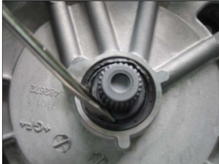
Fig. 3-1: Remove input shaft oil seal
