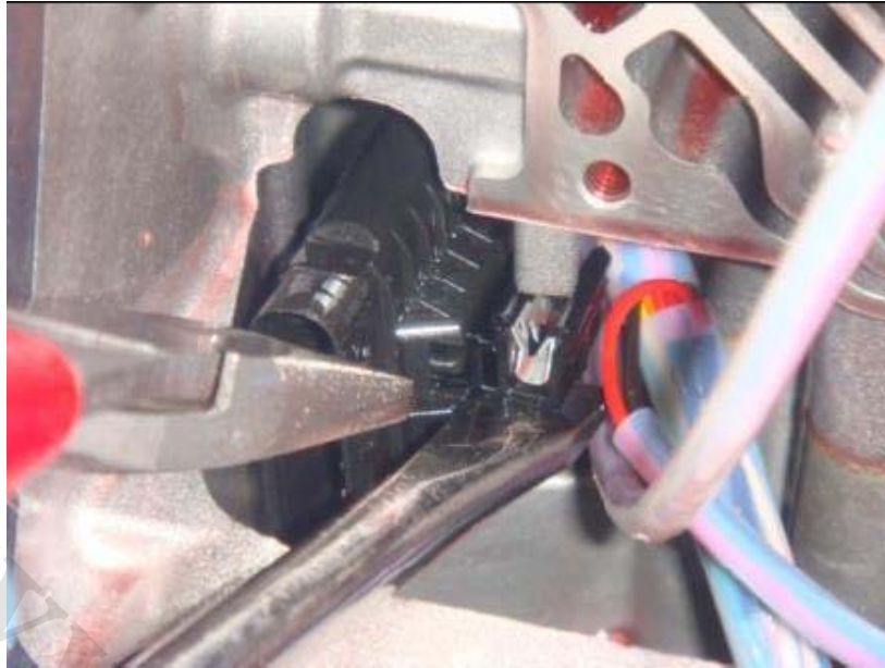
Fig. 15-6: Press driving mode sensor joint on the housing
