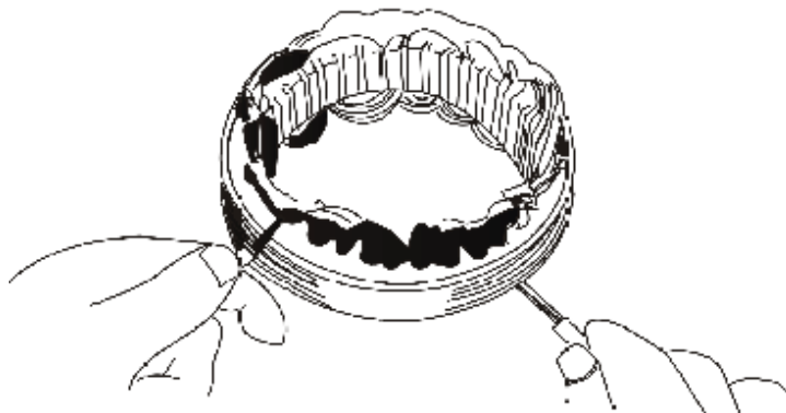
Fig.12-27 Earthing Check of Generator Stator Winding
