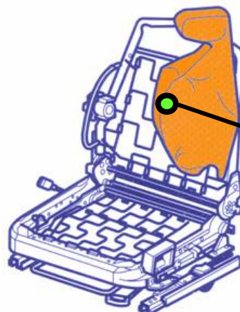
Lateral Airbag Module ( 12 Liter Capacity )
