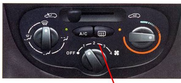
AC / Heater Control Panel
