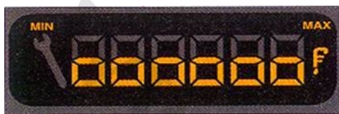
Engine Oil Level Indicator
