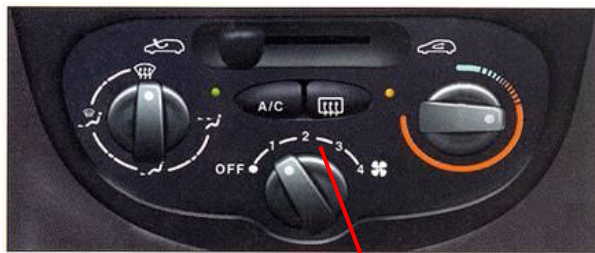
AC / Heater Control Panel
