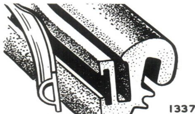
Fig. 2 Removing bright plastic beading from the weatherstrip
