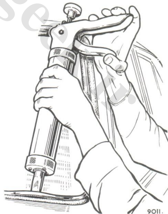
Fig. 11 Sealing glass side of weatherstrip
