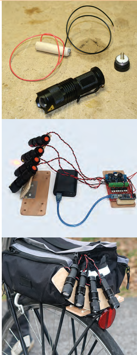
LIGHT IT UP: Wooden "dummy" cells connect to each flashlight's battery terminals [top]; power comes from an Arduino-controlled external source [center]. The flashlights [bottom] are arranged to project light onto the ground.
