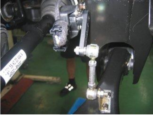
Height sensor attached on rear axle
