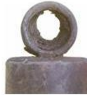
Worn out rubber bearing
