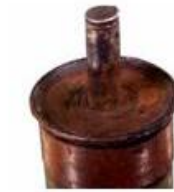
Incorrect tightening torque
