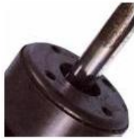
Damaged oil seal
