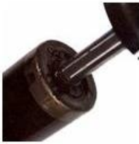
Damaged oil seal
