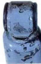
Cracked mounting joint
