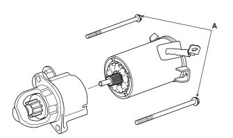
4. Remove the brush holder assembly (A), yoke (b) and armature (C).
