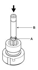
10. After removing the stopper (A) using stopper pliers (B).
