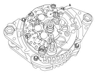
Remove the nut, pulley(A) and spacer.
