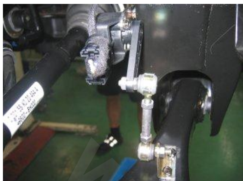
Height sensor attached on rear axle
