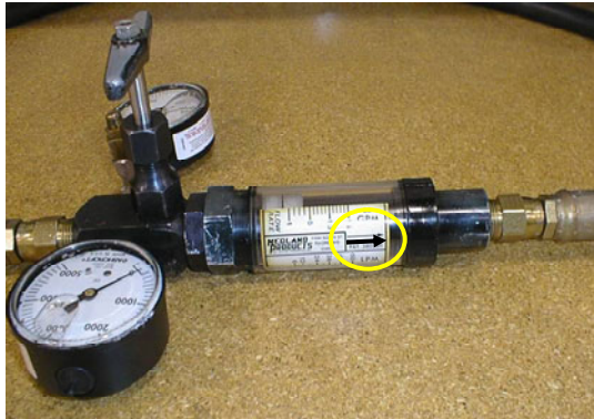
Flow Tester - Install in Series with Circuit Being Tested
