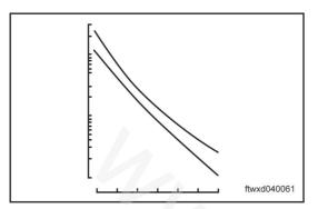
Description Engine coolant temperature sensor is a resister of negative temperature coefficient type. It is characterized by reduction of resistance when engine coolant temperature rises. When resistance rises, the output voltage of engine coolant temperature sensor rises; when resistance drops, the output voltage of engine coolant temperature sensor drops.
