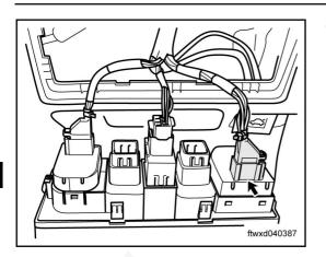
(c) Disconnect switch connector C003 of power rearview mirror
