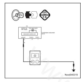
Use a multimeter to measure resistance value.
