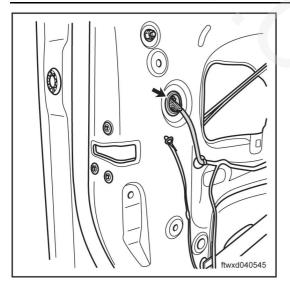
Disconnect connector J007, lock assy, left front door.
