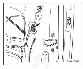
Disconnect connector J007, lock assy, left front door.
