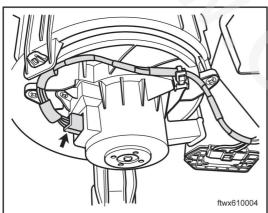
Disconnect the connector C025 of front blower.
