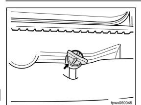
6. Slowly unscrew the coolant drainage plug and drain the coolant.
