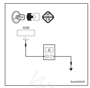
(b) Measure the resistance value between the pin 1 of the connector A006 of ABS control module and ground.
