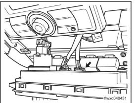
Disconnect the connector C021 of front air conditioner controller.
