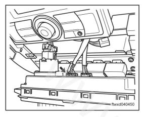
Disconnect the controller connector C022 of air conditioner.
