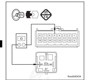
(d) Measure the electrical resistance based on the value in the following form.
