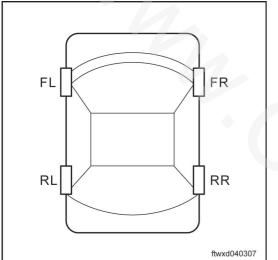
Set the tyre pressure monitoring module at right-rear position, press down RR button for about 3s, if the wheel corresponding to a wheel location stops flickering, setting succeeds.
