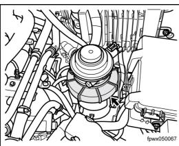
Install the cap and tighten it by turning 3 and a half circles clockwise.
