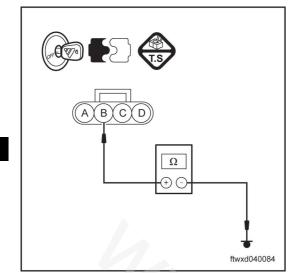
(a) Measure the resistance between pin B of connector E008 of oxygen sensor and ground.
