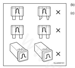
Check fuse : F11 (60A).inside fuse box, engine compartment Check fuse: F40 (10A). inside fuse box of the body
