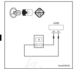
(b) Measure the voltage between the pin 25 and pin 38 of the connector A006 of ABS control module.
