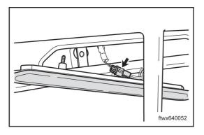
(b) Disconnect the top brake lamp connector F003.
