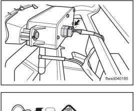
(b) Disconnect the connector C027 of the combined display.
