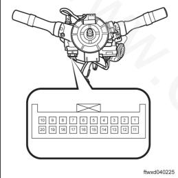
(c) Check the combination switch (lamplight switchover) Standard resistance:
