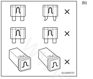
Check the fuse F32 (10A) in the vehicle-borne fuse box.
