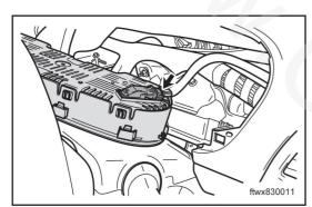
(b) Disconnect the connector C013 of combination instrument.
