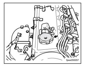
15. Unscrew the engine oil filler cap.
