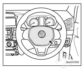
The driver's air bag is located in the center of the steering wheel. Visually inspect the completeness of the plastic cover.
