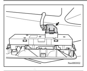
(a) Disconnect connector J004 of power window switch, driver's door.
