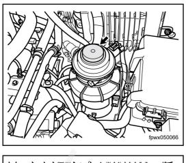
(b) Press the cover and pump the fuel manually, until fuel spills front he discharge screw.
