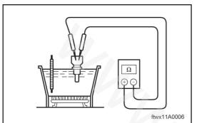
(c) Use a multimeter to measure the resistance of engine coolant temperature sensor at different water temperature, and its reference value shall conform to the items listed in the table below.
