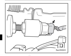
(b) Disconnect the brake lamp switch connector.
