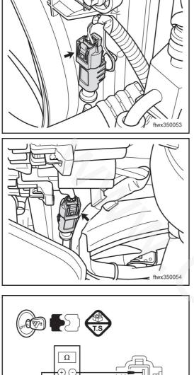
Disconnect the connector A002 of right front wheel speed sensor and the connector A014 of left front wheel speed sensor.
