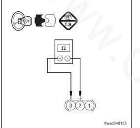
Use multimeter to measure the resistance between No.2 stitch speed sensor E001 connector and No.3 stitch.
