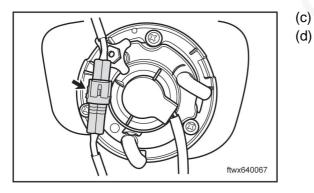
Disconnect the left front fog lamp connector A016. Disconnect the right front fog lamp connector A005.
