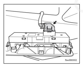
(b) Pull out power window switch J004, driver's door
