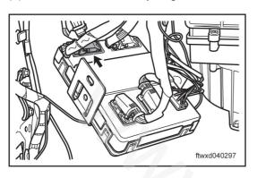
Disconnect the connector C036 of BCM control unit.
