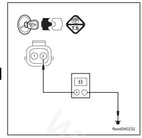
(e) Measure the electrical resistance based on the value in the following form.
