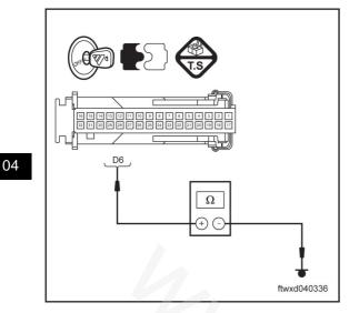
(b) Use multimeter to measure the resistance between stitch D6 of connector C035 of body controller and the ground.
