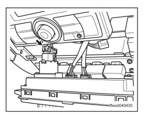
Disconnect the connector C018 of blower switch.
