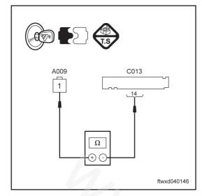
(b) Use a multimeter to measure the resistance between no. 14 pin of connector of the combination instrument C013and the pin 1 of connector of the brake liquid level alarm switch A009.
