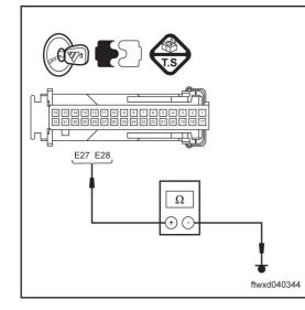
(b) Use multimeter to measure the resistance between. stitches E27, E28of connector C036 of the body controller and the ground.
