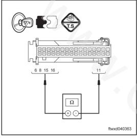
(b) Use a multmeter to measure power window switch, driver's door.
