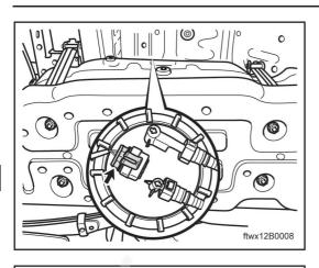
(b) Disconnect the connector of the fuel sensor B001.
