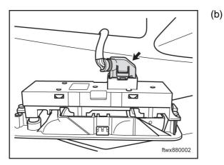
Pull out Power window switch connector J004, driver's door
