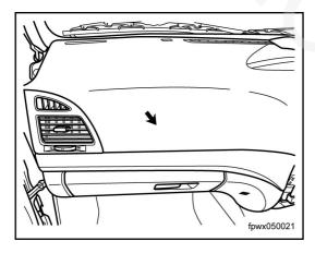
The front passenger's air bag is located above the glove compartment. Visually inspect the completeness of the plastic cover.
