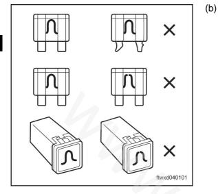
Check fuse of fuse box, engine room: F13 (30A), F14 (30A)
