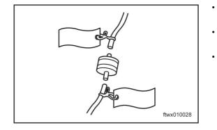
L1 L2 ftwx010029 When disconnecting a vacuum hose connector, label it to faciliate the identification upon connection.
