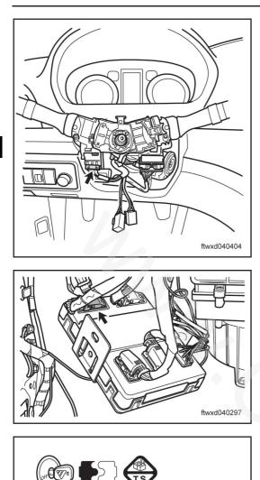
(b) Disconnect the connector C008 of combination switch (lamplight switchover).
