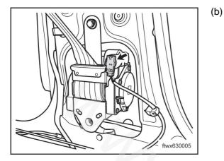
Disconnect preloading assembly connector D002, driver's seat belt.
