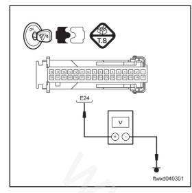
(b) Use a multimeter to measure the voltage between pin E24 of connector C036 of vehicle body controller and ground.
