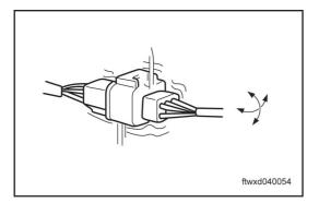
Connector: Shake the connectors gently in vertical and horizontal directions, and check whether or not the harness connectors connected to corresponding parts get loose. Check the terminals for soil, rust, corrosion, and bend. Check for any loose contact caused by elongation of terminals.
