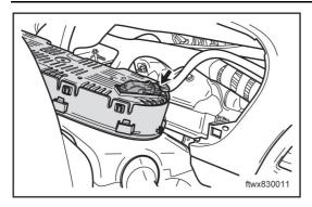
Disconnect the connector C013 of combination instrument.
