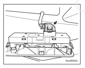
Pull out Power window switch connector J004, driver's door
