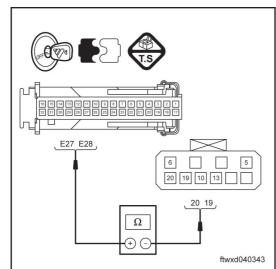
Use multimeter to measure the resistance between stitches 19 and 20 of connector J007of lock assy for the left front door and stitchesE27,28 of connector C036 of body controller.
