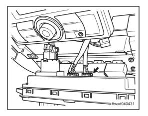
(b) Disconnect the connector C021 of air conditioner controller.
