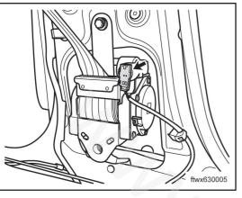
Disconnect preloading assembly connector D009, passengers' seat belt.
