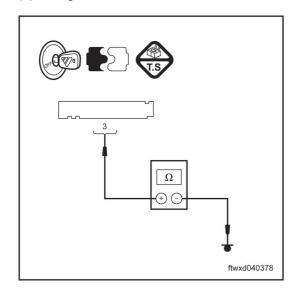
Use a multimeter to measure the resistance between pins 3 of connector C013 of the combination instrument and the ground.
