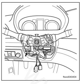
(b) Disconnect the connector C008 of combination switch (lamplight switchover).
