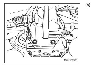
Disconnect reverse lamp switch connector E002.
