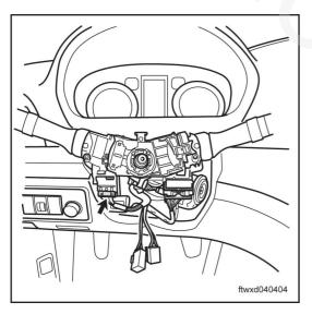
Disconnect the connector C008 of combination switch (lamplight switchover).
