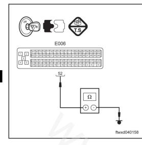
Use a multimeter to measure the resistance between pin 52 of connector E006 of engine control module and the ground.
