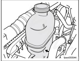
Check the coolant level, which should be near Line (when the engine is cooled down).
