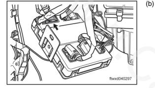
Disconnect body controller C036 connector.
