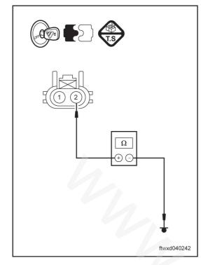
Measure the electrical resistance based on the value in the following form.
