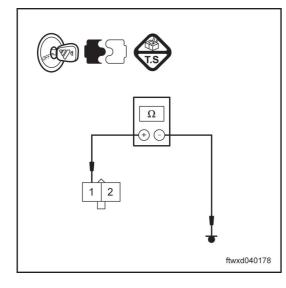
Use a multimeter to measure resistance value.
