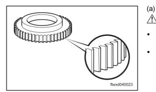
Check the teeth of signal gear.
