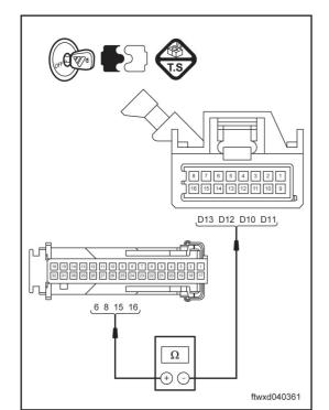
(c) Measure the electrical resistance based on the value in the following form.
