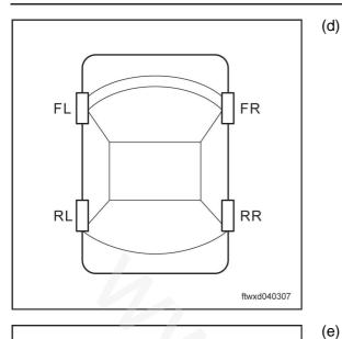
(d) Set the tyre pressure monitoring module at right-front position, press down FR button for about 3s, if the wheel corresponding to a wheel location stops flickering, setting succeeds.
