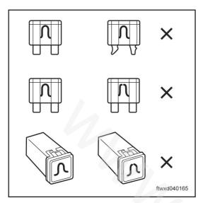
Check the fuse F30(7.5 A) in the indoor fuse box (C037).
