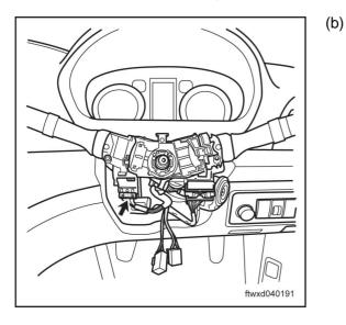
Disconnect the connector C008 of combination switch (turn).
