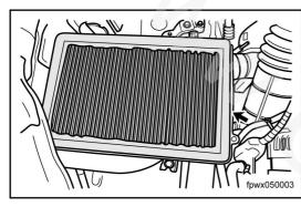
4. Remove the air filter element.
