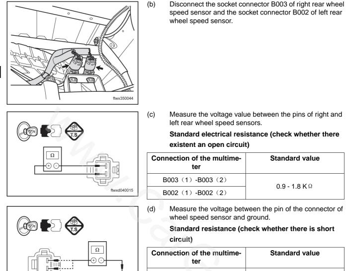
Connection of the multime-<br/>terStandard valueB003 (1) - groundB003 (2) - groundB002 (1) - ground $\geqslant 1 M \Omega$ B002 (2) - ground $\implies 1 M \Omega$
