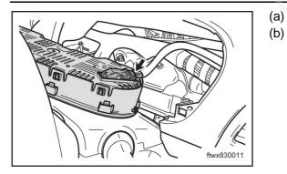
Disconnect assembly instrument C013 connector Ignition Switch: ON.
