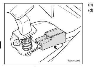
Disconnect the braking switch connector D007. Ignition Switch: ON.
