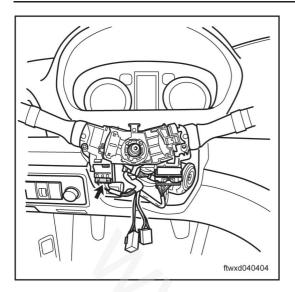
(b) Disconnect the connector C008 of combination switch (lamplight switchover).
