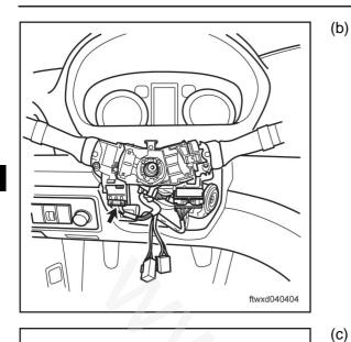
(b) Disconnect the connector C008 of combination switch (lamplight switchover).
