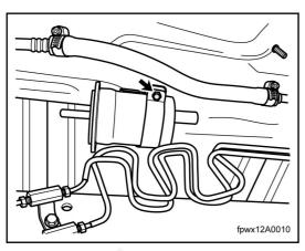
6. Install a new fuel filter assembly and tighten the retaining bolts.
