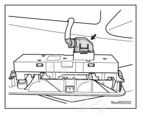
Disconnect connector J004 of power window switch, driver's door.
