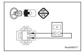
(a) Check output voltage of the right rear, left rear wheel speed sensors while rotating.
