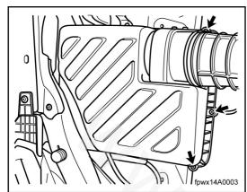
Unscrew the screw. Slightly lift up the outlet in the upper housing of the air filter, while pulling it towards the engine. Pull it out of the dowel pin hole in the lower housing, in order to separate the upper and lower housings.
