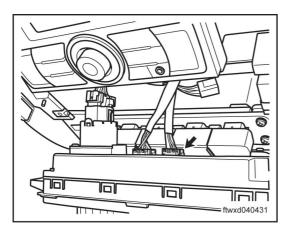
Disconnect connector C021 of air-conditioner controller.
