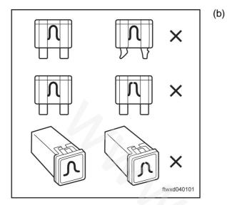
Check fuse inside fuse box, engine compartment : F14 (30 A).
