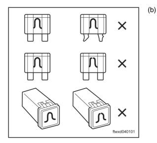
Check the fuse F5 (10A) in the indoor fuse box.
