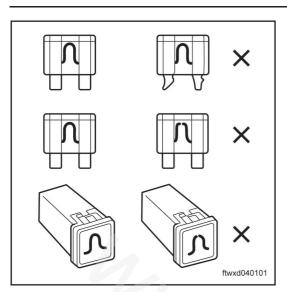
(a) Check whether fuse F26 (7.5A) of the body is fusing or not.
