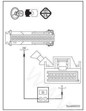
(c) Use multimeter to measure the resistance between stitch 2 of connector J004 of power window switch of right front door and stitch D6 of connector C035 of body controller.
