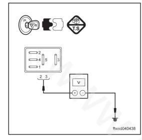
(f) Measure the voltage based on the value in the following form.
