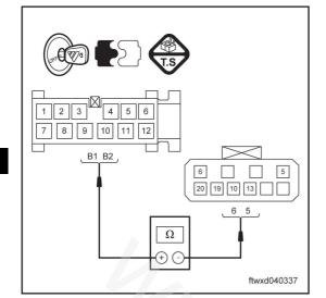
Use multimeter to measure the resistance between stitches B1, B2 of connector C033 of body controller and stitches 6 and 5.
