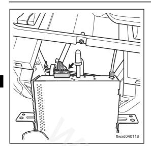
(a) Disconnect the connectors of acoustics unit.
