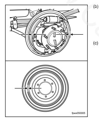
Measure the thickness of the brake lining (without back plate) and brake drum.
