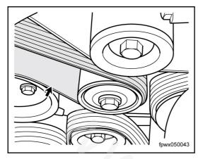
Check for breakage and aging sign on the accessory belt and replace it if needed.
