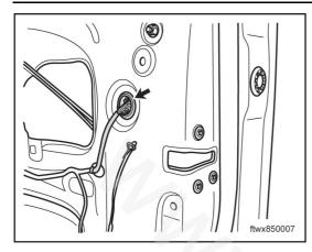
Disconnect connector G006 of door lock motor of right front door.
