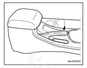
2. Check whether the park brake works smoothly, whehter the pulling strength required by the handle is correct and whether the cable is damaged. Overhaul it if needed.
