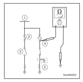
Remove the blown-out fuse, and measure the resistance between the load side of the blown-out fuse and the ground. Turn off all switches connected to the circuit where the said fuse stays. If the resistance measured at this moment approximates to 0, a short-circuit must occur in some places
