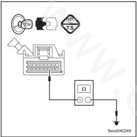
(b) Use multimeter to measure the resistance between stitch 11 of connector J004 of power window switch of left front door and the ground.
