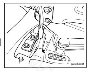
Check whether there is any impurity and blockage in the drain whole and clean it if needed.
