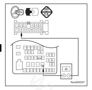
(c) Measure the electrical resistance based on the value in the following form.
