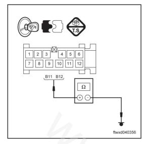
(b) Use multimeter to measure the resistance between stitches B11, B12 of connector C033 of the body controller and ground.
