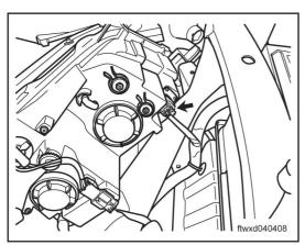
Disconnect the left front turn light connector A010.
