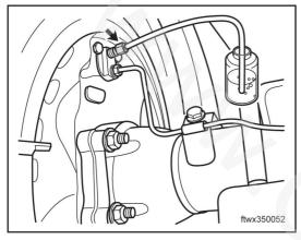
Connect the discharge screw and the collection vessel with a clear plastic hose.
