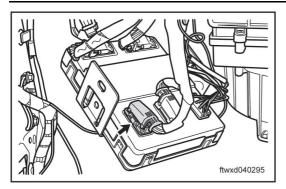
Disconnect connector C033, body controller.
