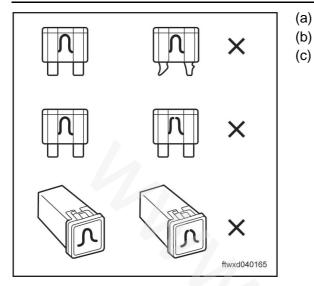
Switch off the ignition. Disconnect fuse F12 (30A). Check fuse
