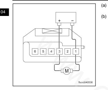
Connect the battery positive terminal (+) to pin 3 of connector of temperature regulation servo motor.Connect the battery negative terminal (-) to pin 1 of connector of temperature regulation servo motor.
