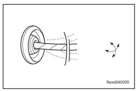
(b) Harness: Shake the harness gently in vertical and horizontal directions, and check thoroughly connections of the vibrated connectors and the harness inside the engine/ driver's cabin instruments for disconnected harness.
