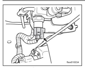
(c) Disconnect the connector A001 of air-condition pressure switch.
