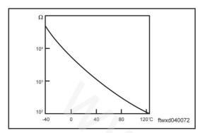
Description Intake temperature sensor is a resister of negative temperature coefficient type. Its resistance is drops when intake temperature rises. When resistance rises, the output voltage of intake temperature sensor rises; when resistance drops, the output voltage of intake temperature sensor drops.
