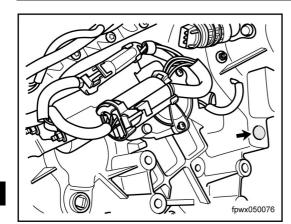
6. Use tools to top the differential oil up at the filler, until it overflows the hole.
