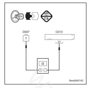
(b) Use a multimeter to measure the resistance between pin 31of connector of the combined instrument C013 and the pin 1 of connector D007 of manual braking switch.
