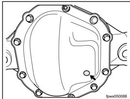
6. Use tools to add rear main reducer gear oil at the filler, and additive as well for LSD.
