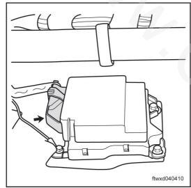
Disconnect SRS control module connector C016.
