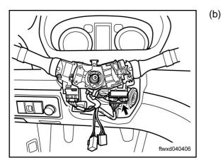
Disconnect the connector C012 of combination switch (wiper).
