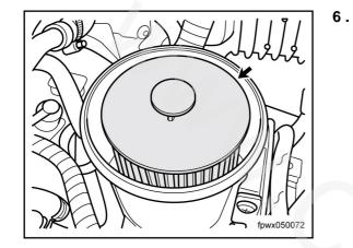
Remove the fuel filter element and replace it with a new one.
