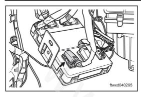
(a) Disconnect connector C033, body controller.
