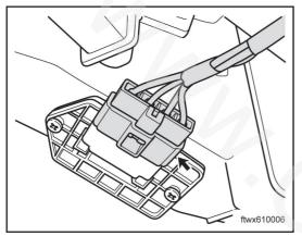
(b) Disconnect the connector C024 of blower governing resistor.
