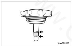
6. Check the level, which should be between the maximum level and the minimum level. If not, drain it or top it up.
