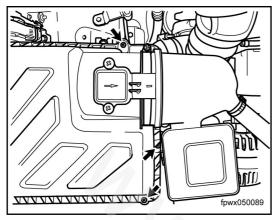
Unscrew the screw. Slightly lift up the outlet in the upper housing of the air filter, while pulling it towards the engine. Pull it out of the dowel pin hole in the lower housing, in order to separate the upper and lower housings.
