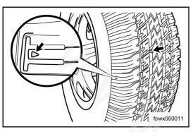
3. Check the tread depthn (including spare tire) and ensure the depth is greater than that of the wear indicator and the side wear indicator hasn't been fully worn.
