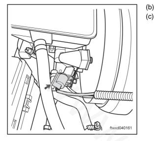
Disconnect the connector A008of the vacuum alarm. Ignition Switch: ON.
