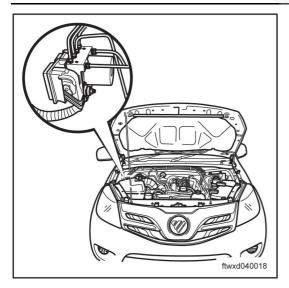
disconnect the connector A006 of the ABS module.
