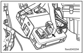
(b) Press down power window motor 1004, left rear door
