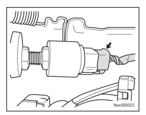
Disconnect the driving braking switch connector C004.
