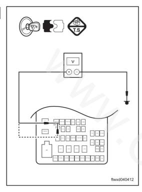
(b) When ignition switch is on, check fuse F24 of the fuse box on the vehicle body.
