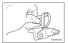
(a) Check right front, left front wheel speed sensor signal terminal
