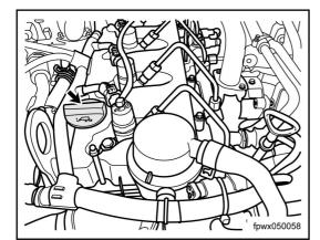
16. Unscrew the engine oil filler cap.
