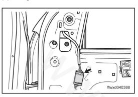
Disconnect left power rearview mirror connector J003. Disconnect right power rearview mirror connector G002.
