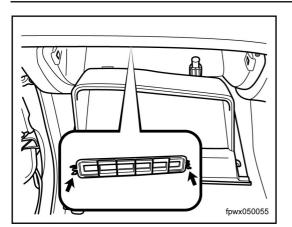
6. Mount the cover used to replace the filter element and then the clip.
