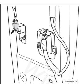
Disconnect the door control switch connector.
