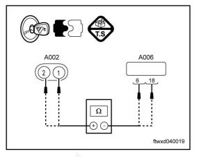
(b) Measure the resistance of the connectors of the harness as per the values given in the table below
