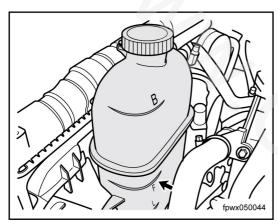
10. Top up the engine coolant to the specified level.
