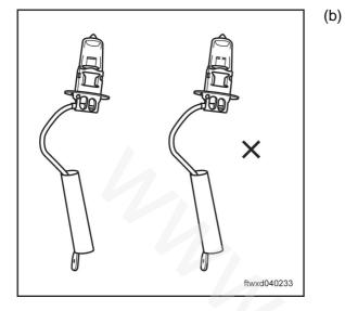
Check whether or not the bulbs of rear fog lamps are damaged.
