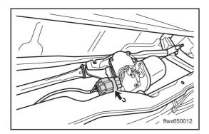
(b) Disconnect the connector A007 of front wiper assembly.
