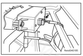
Disconnect the connector C027 of the combined display.
