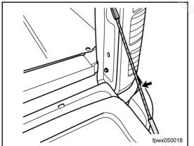
Repeatedly open and close the rear plate assembly hinge, check whether the hinge moves smoothly and apply grease if needed.
