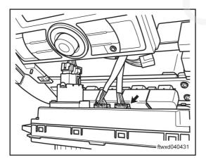
(b) Disconnect connector C021 of air-conditioner controller.
