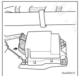
Disconnect SRS control module connector C016. Connect the negative pole of the battery and turn on ignition switch to "ON".
