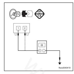
(e) Check the resistance between clock spring socket C010 and driver' s SRS assembly connector.
