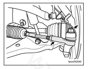
Swing the tie rod and make sure there is no gap. Check whether the retaining nut on the ball joint is secured.
