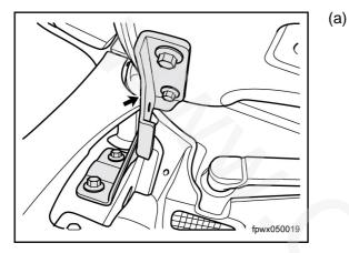
Repeatedly open and close the engine hood cover, check whether the hinge moves smoothly and apply grease if needed.
