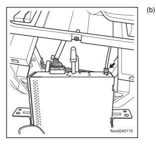
Remove the antenna connector of the acoustics unit.
