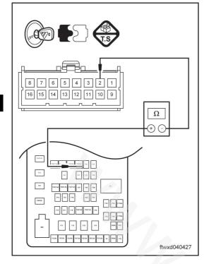
(c) Measure the electrical resistance based on the value in the following form.
