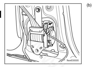
Disconnect preloading assembly connector D009, passengers' seat belt.
