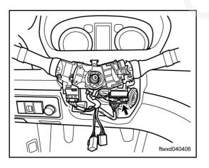
(b) Disconnect the connector C012 of combination switch (wiper).
