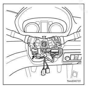
Disconnect the connector C008 of combination switch (turn).
