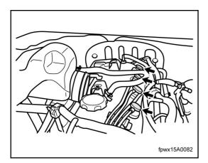
6. Install the spark plug cable to the rock arm cap.
