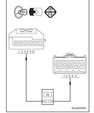
Disconnect the temperature regulation servo motor C031.
