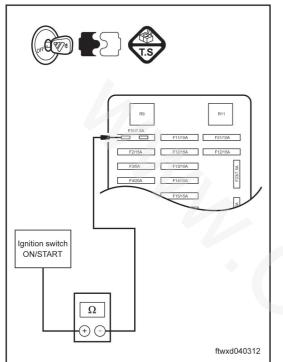
Measure the electrical resistance based on the value in the following form.
