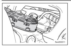
Disconnect assembly instrument C013 connector
