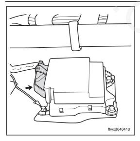
Disconnect SRS control module connector C016.
