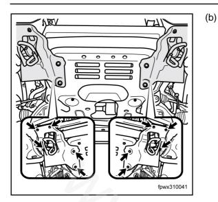
Install the small baffles on both sides and tighten the retaining bolts.
