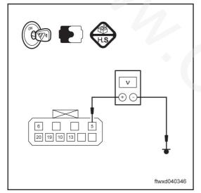
Use master control switch to lock the door, meanwhile use multimeter to measure the voltage between stitch5 of connector G006 of right front lock motor and the ground.
