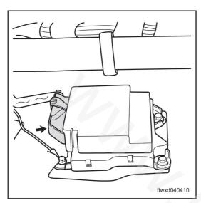
Disconnect SRS control module connector C016.
