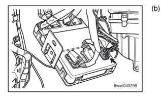
Disconnect the connector C034 of BCM control unit.
