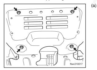
Install the front baffle and tighten the retaining nuts. Torque: 23±2N<sup>•</sup>m
