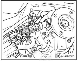
Disconnect speedometer E001 connector Ignition Switch: ON.
