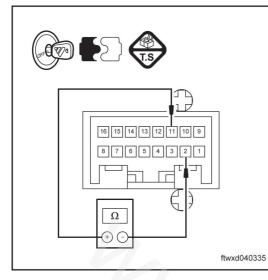
(b) Use multimeter to measure the resistance between stitch 11of connector J004 of power window switch of left front door and stitch11.
