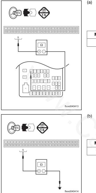
Check whether the result is normal? Yes> Replace SRS Control Module No> replace harness When ignition switch is off, pull out fuse F24 of the fuse box and check the resistance value between the connector C016 for the fuse box and SRS control module.
