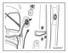
(a) Disconnect connector J007, lock assy, left front door.
