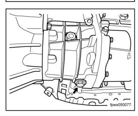
5. Once completely drained, tighten the drain bolt.
