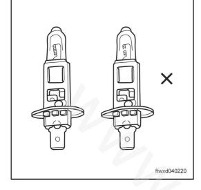
Check whether or not the bulb of left turn light is damaged.
