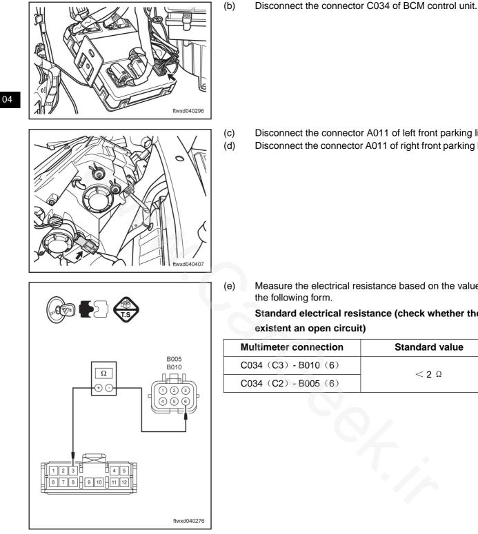
Disconnect the connector A011 of left front parking light. Disconnect the connector A011 of right front parking light.
