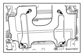
Install the rear baffle and tighten the retaining bolts. Torque: 23±2N°m
