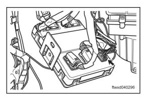
Disconnect the connector C034 of the vehicle body controller.
