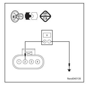
(b) Use a multimeter to measure the voltage between pin 2 of the connector of the fuel sensor B001 and ground.
