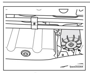
11. Use the tools to remove the oil filter and replace a new one.
