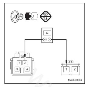
(d) Measure the electrical resistance based on the value in the following form.
