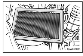
Mount the air filter element.
