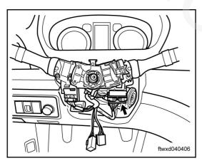
Disconnect the connector C012 of combination switch (wiper).
