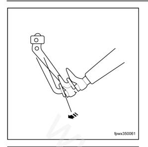
A mechanic shall press the brake pedal by full force for 7-9 times and hold it in position.
