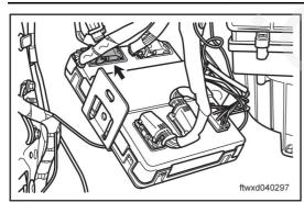
Disconnect body controller C036 connector.
