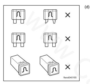
Check interior fuse box (C037) fuse: F31 (7.5A).
