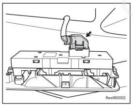
(b) Pull out power window switch J004, driver's door
