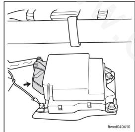
Disconnect SRS control module connector C016.
