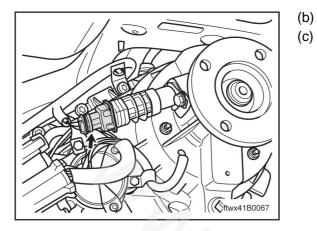
Disconnect speedometer E001 connector Ignition Switch: ON.
