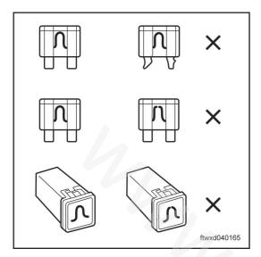
Check the fuse F36 (10 A) in the vehicle body fuse box (C037).
