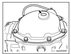
6. Use tools to front main reducer gear oil at the filler. Gear oil model: GL-5 85W/90 Filling volume: 1.2L
