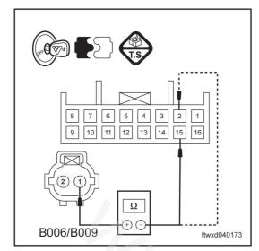
Standard electrical resistance (check whether there existent an open circuit)
