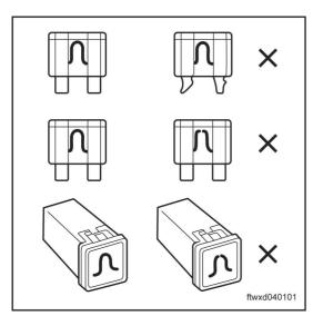
Check the fuse F27 (15A) inside the fuse box of engine compartment.
