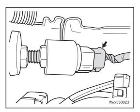
(b) Disconnect the brake lamp switch connector.
