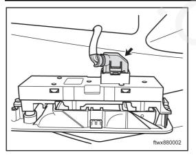
Disconnect connector J004 of power window switch, left front door.
