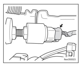
Disconnect the driving braking switch connector C004.
