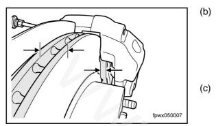
Meausre the thickness of the brake lining (without back plate) and brake disc.
