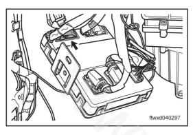
Disconnect connector C036, body controller
