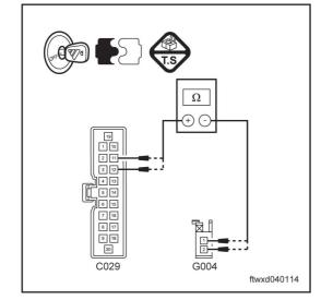
(c) Use a multimeter to measure the resistance between pins 11 and 12 of connector C029 of acoustics unit and pins 1 and 2 of connector G004 of speaker of front right door.
