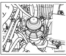
5. Remove the diesel filter & heater connector.
