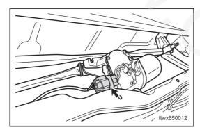
Disconnect the connector A007 of front wiper motor .
