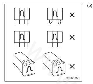
Check fuse inside fuse box, engine compartment : F13 (30 A).
