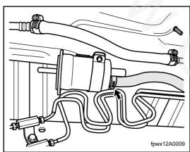
Unscrew the clip bolt and remove the hose.
