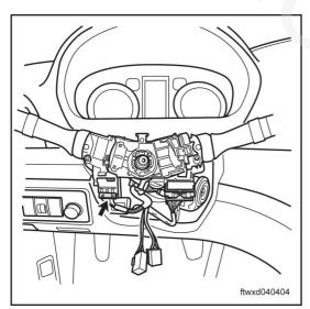
(b) Disconnect the rear fog lamp switch connector C017.
