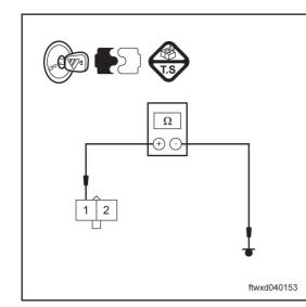
(c) Use a multimeter to measure the resistance between the pin 1 of the connector of the seat belt alarm switch D006 on the side of driver and ground.
