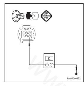
Use a multimeter to measure resistance value.
