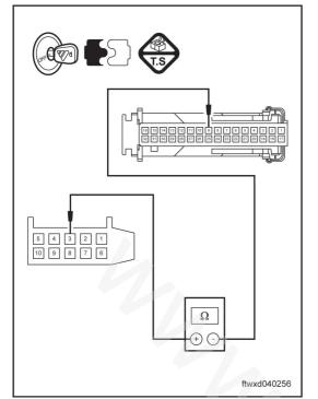
(d) Measure the electrical resistance based on the value in the following form.
