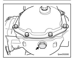
5. After completely drained, replace the drain bolt gasket and tighten the drain bolt.
