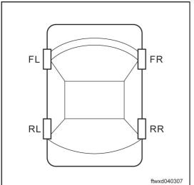
Graphic patterns appear on the instrument LCD of the vehicle, showing that it has entered studying state, now loosen the button. Now the four wheels are at twinkling state.
