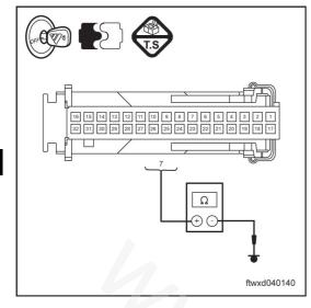
Use a multimeter to measure the resistance between pin 7 of connector of the combination instrument C013 and the ground.
