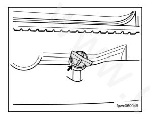
7. Once the coolant is drained up, tighten the plug.
