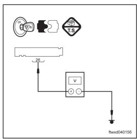
(a) Use a multimeter to measure the voltage between pin 26 of connector of the combination instrument C013 and the ground.
