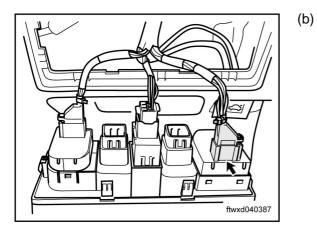
Disconnect switch connector C003 of power rearview mirror
