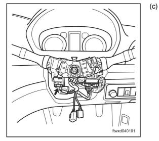
Disconnect the connector C008 of combination switch (turn).
