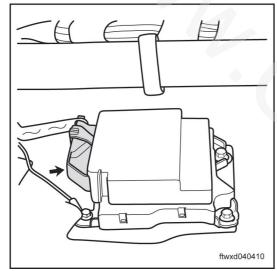
Disconnect SRS control module connector C016.
