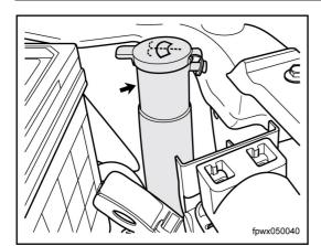
(a) The level of the windscreen cleaner shall be 10cm below the opening. Top it up if below that level.
