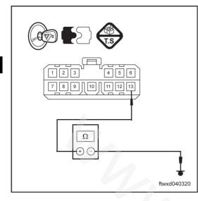
Use a multimeter to measure resistance value.
