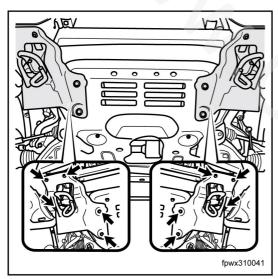
Unscrew the retaining bolts of the small baffles on both sides and remove the baffles.
