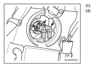
Disconnect the connector A011 of left front passing lamp. Disconnect the connector A003 of right front passing lamp.
