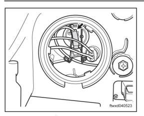
(c) Disconnect the connector A011 of left front driving light.(d) Disconnect the connector A003 of right front driving light.
