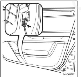
(b) (c) Disconnect the left step lamp connector J006.
