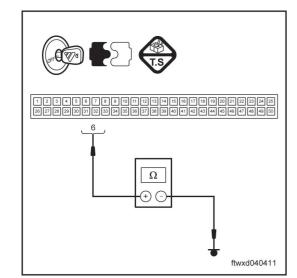
(d) Measure the electrical resistance based on the value in the following form.
