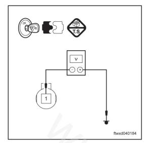
(d) Use the multimeter to measure the voltage betweenpin 1 of connector A008 of vacuum alarm and ground .
