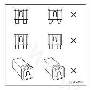
Check fuse: F8 (25A) inside interior fuse box fuse.
