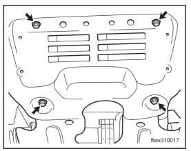
Unscrew the retaining bolts of the front baffle and remove the baffle.
