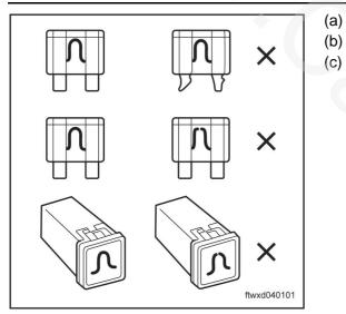
Switch off the ignition. Disconnect fuse F16 (40A). Check fuse
