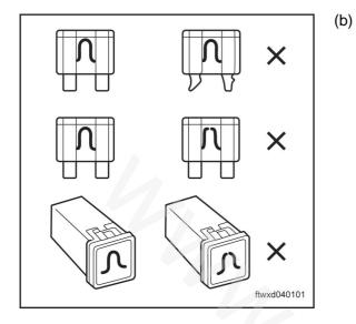
Check the fuse inside engine compartment: F8 (25A)
