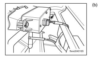
Disconnect the connector C027 of the combined display.
