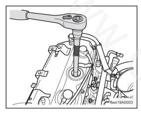
Remove the spark plug with tools. 4.
