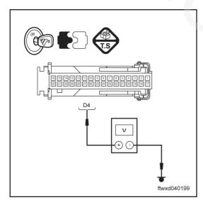
(b) Use a multimeter to measure the voltage between pin D4 of connector C035 of vehicle body controller and ground.
