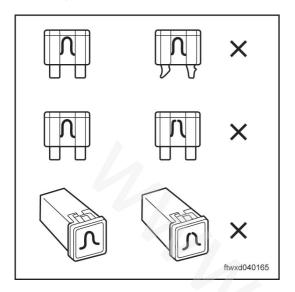
Check the fuse F35(20 A) in the indoor fuse box (C037).
