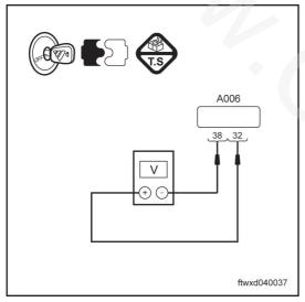
(b) Turn on the ignition switch and measure the voltage between the pin32 and pin 38 of the connector C006 of ABS control module.
