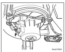
Disconnect the connector C025 of blower motor.
