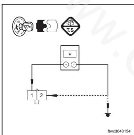
Use a multimeter to measure the voltage between the pin 1 of the connector of the seat belt alarm switch D013 on the side of passenger and ground; the pin 1 and pin 2.
