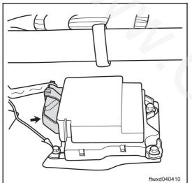
Disconnect SRS control module connector C016. Disconnect the connector of clock spring C010. Connect the negative pole of the battery and turn on ignition switch to "ON".
