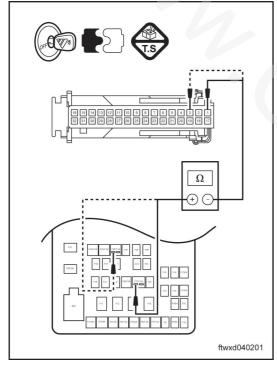
(c) Measure the electrical resistance based on the value in the following form.
