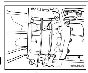
6. Top the gearbox lubricant from the filler until it overflows from the hole.
