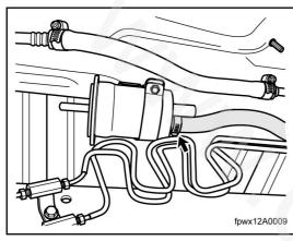
Install the hose and tighten the clip bolts.
