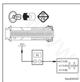
(d) Measure the electrical resistance based on the value in the following form.
