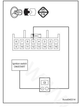
(c) Use a multimeter to measure resistance value.
