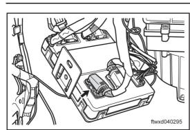
(b) Disconnect the connector C033 of BCM control unit.
