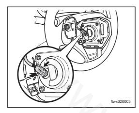
(b) Disconnect the connector of lock spring C009.
