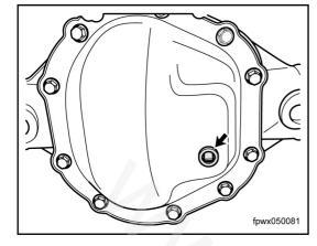
3. Unscrew the rear main reducer filler plug.
