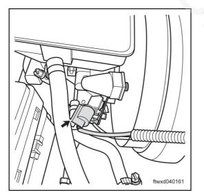
(b) (c) Disconnect the connector A008 of the vacuum alarm. Ignition Switch: ON.
