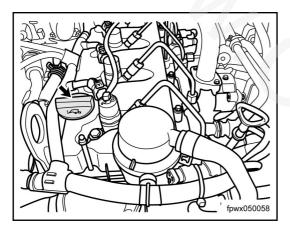
Tighten the engine oil filler cap.
