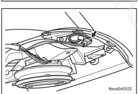
Disconnect the left rear-view mirror connector G002.
