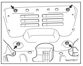
Install the front baffle and tighten the retaining nuts.
