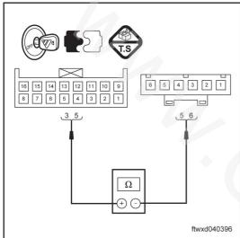
Measure the electrical resistance based on the value in the following form.
