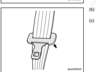
Check for distortion, disconnection and crack on the cover of guide buckle and replace it if needed.
