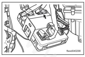
Disconnect connector C035, body controller.
