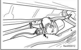
Disconnect the connector A007 of front wiper motor.
