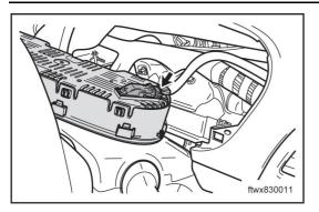
Disconnect assembly instrument C013 connector
