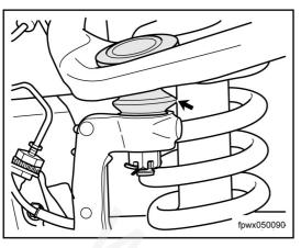
1. Check for damage in the dust shield of the upper arm ball and replace it if needed.
