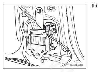
Disconnect preloading assembly connector D009, passengers' seat belt.
