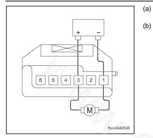
Connect the battery positive terminal (+) to pin 3 of connector of mode air door servo motor. Connect the battery negative terminal (-) to pin 1 of connector of mode air door servo motor.
