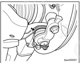
Check for damage in the dust shield of the bottom arm ball and replace it if needed.
