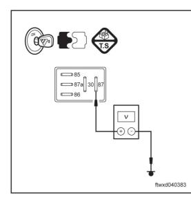
(c) Measure the voltage based on the value in the following form.
