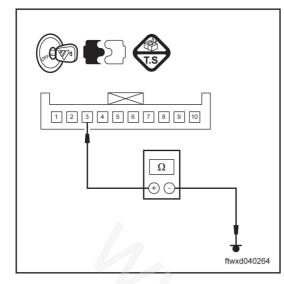
(c) Measure the electrical resistance based on the value in the following form.
