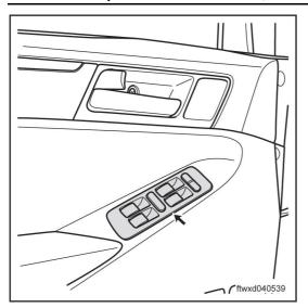
Dismantle power window switch, left front door.
