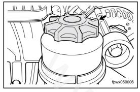
Screw out the filler cap of the power steering tank.
