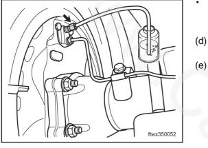
The other mechanic unscrews the braking fluid discharge screw, until the pressed brake pedal moves downward. Immediately tighten the discharge screw.
