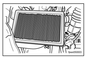
Mount the air filter element.
