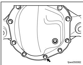
5. Once completely drained, tighten the drain bolt.
