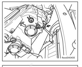
(c) Disconnect the right front turn light connector A004.
