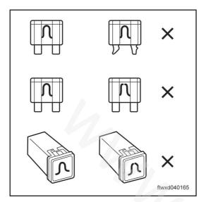
Check whether the fuse of the interior fuse box: F7 (7.5A), F30 (7.5A) is fusing or not.
