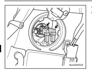
(c) Disconnect the connector A011 of left front passing lamp.(d) Disconnect the connector A003 of right front passing lamp.
