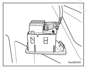
(b) Press down power window switch H001, right rear door.
