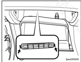
Press the clip and remove the cover used to replace the air-conditioning filter element.
