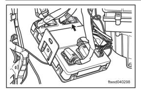
Disconnect connector C035, body controller.
