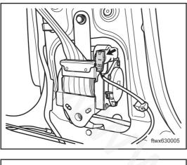
Disconnect preloading assembly connector D002, driver's seat belt.
