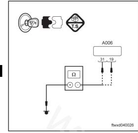
(c) Measure whether there is short circuit in the resistance between harness pins
