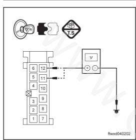
(c) Measure the electrical resistance based on the value in the following form.
