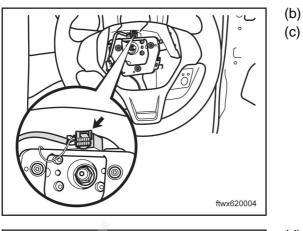
Disconnect the connector of lock spring C009. Disconnect the horn switch connector.
