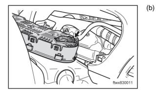
Disconnect the connector C013 of combination instrument.
