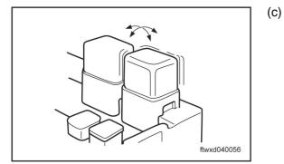
Relay: parts and sensors: Pat the sensors, relays, or parts which are considered as the source of failure, and check them for malfunction. However, do not beat the relays violently for fear of open circuit of the relays.
