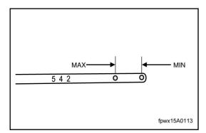
22. Check the engine oil level. If it is above the maximum level, drain the oil to the normal range. If it is below the minimum level, top it up to the normal range.
