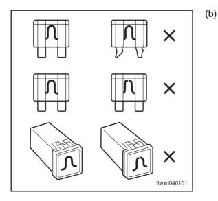
Check the fuse F1 (15A) in the indoor fuse box.
