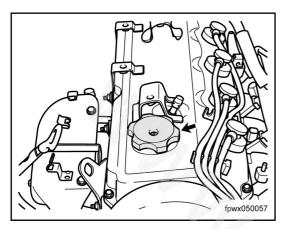
17. Tighten the engine oil filler cap.
