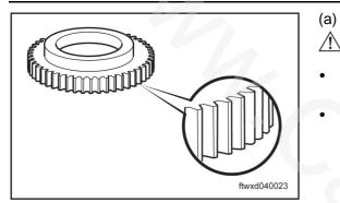
Check the teeth of signal gear.
