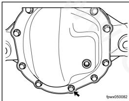
4. Unscrew the rear main reducer drain plug and drain the gear oil.
