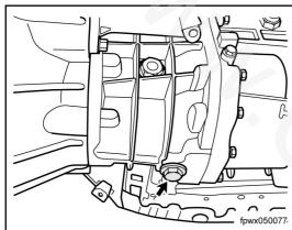
4. Unscrew the gearbox drain bolt and drain the lubricant.  $\triangle$
