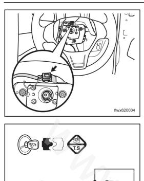
Disconnect the connector of lock spring C009.
