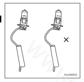
Check whether or not the bulbs of front fog lamps are damaged.
