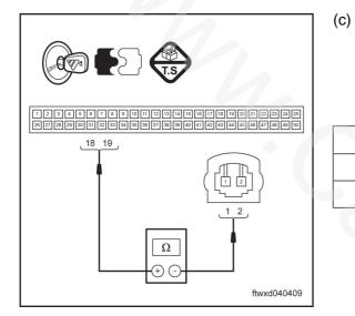
Measure the resistance between SRS control module connector C016 and Passengers' air bag connector C030.
