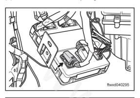
Disconnect the connector C034 of BCM control unit.
