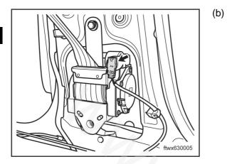
Disconnect preloading assembly connector D002, driver's seat belt.
