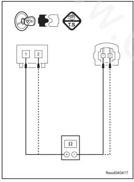
(d) Check the resistance between clock spring socket C010 and driver' s SRS assembly connector.
