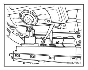
Disconnect the connector C021 of air conditioner controller.
