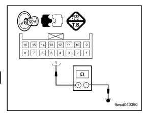
(c) Measure the electrical resistance based on the value in the following form.
