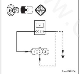
Use multimeter to measure speedometer sensor E001 connector No.1 stitch and No.2 stitch respectively, and the voltage between No.1 stitch and ground connection.
