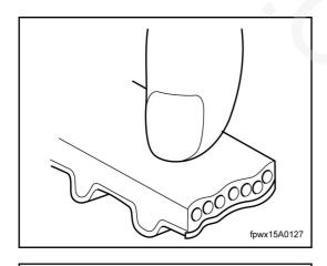
Aged and shiny rubber on the back, showing no nail scratch.
