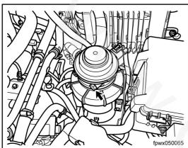
Tighten the discharge screw.
