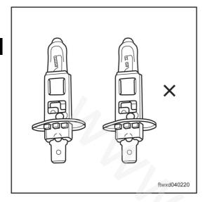
Check whether or not the bulb of right turn light is damaged.
