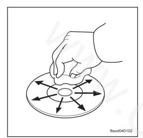
(b) If yes, wipe and clean the CDs from interior to exterior in radial direction with soft cloth, as shown in the figure.
