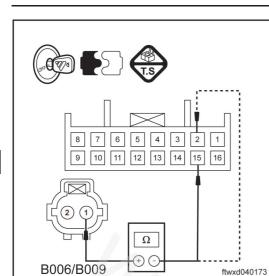
(e) Measure the electrical resistance based on the value in the following form.
