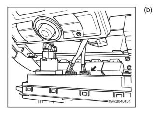
Disconnect connector C021 of air-conditioner controller.
