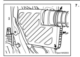
Insert the dowel pin in the upper housing of the air filter to the hotel in the lower housing, in an inclined way. Press the outlet of the upper housing downward and align three screw holes in both housings. Install and tighten the retaining screws.
