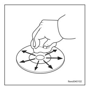
(b) If yes, wipe and clean the CDs from interior to exterior in radial direction with soft cloth, as shown in the figure.
