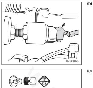
Ω +) (- Disconnect the driving braking switch connector C004.
