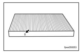
5. Mount a new air-conditioning filter element.
