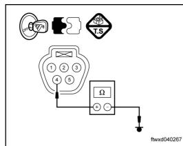
(d) Measure the electrical resistance based on the value in the following form.
