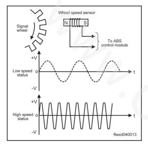
Speed sensor detects wheel speed and transmits speed signal to the ABS module. ABS system uses these signals to control each actuator.
