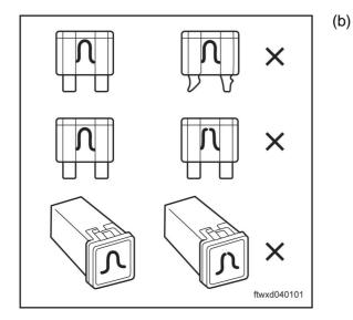
Check the fuse F18 (15A) inside the fuse box of engine compartment.
