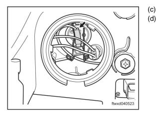
Disconnect the connector A011 of left front driving light. Disconnect the connector A003 of right front driving light.
