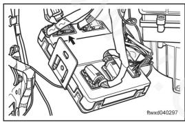
Disconnect the connector C036 of BCM control unit.
