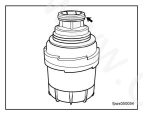
13. Apply a small amount of engine oil on the O-ring of the new oil filter.
