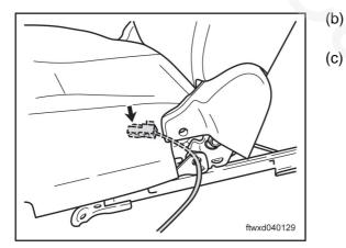
Disconnect the connector of the seat belt alarm switch D013 on the side of driver. Ignition Switch: ON.
