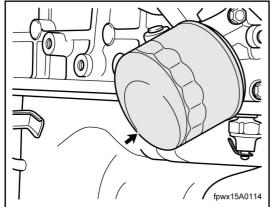
Use the tools to remove the oil filter and replace a new
