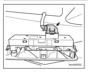
(a) Disconnect connector J004 of power window switch, left front door.
