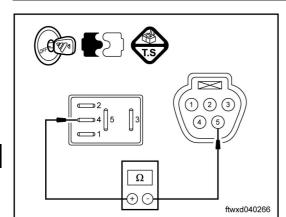
(d) Measure the electrical resistance based on the value in the following form.
