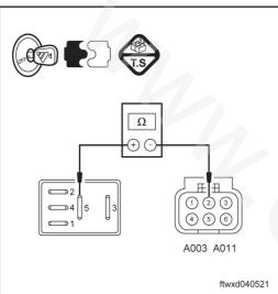
Measure the electrical resistance based on the value in the following form.
