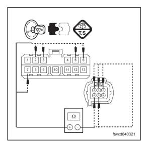
Use a multimeter to measure resistance value.
