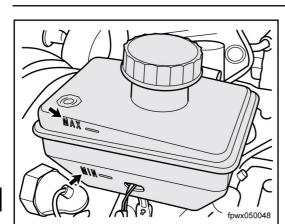
5. After the drainage, top the braking fluid inside the tank up to the standard range.
