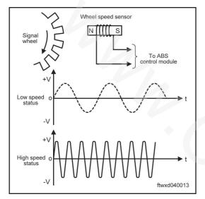
Speed sensor detects wheel speed and transmits speed signal to the ABS module. ABS system uses these signals to control each actuator.
