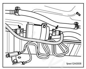
3. Press the locking block and remove the fuel filter connector.
