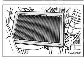
4. Remove the air filter element.
