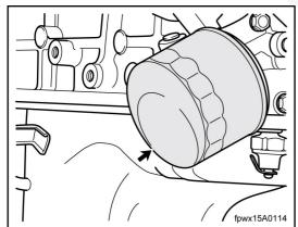
13. Mount the oil filter onto the holder by hand, until the O-ring of the filter touch the holder, and then tighten the filter with tools.
