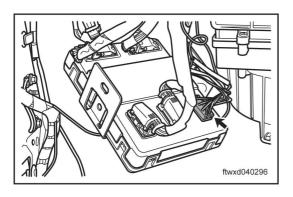
Disconnect the connector C034 of BCM control unit.
