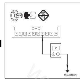
(c) Measure the voltage based on the value in the following form.
