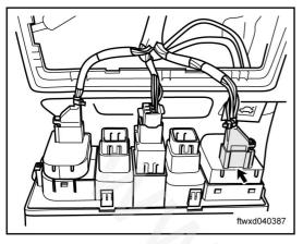
Disconnect switch connector C003 of power rearview mirror
