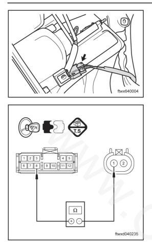
(c) Disconnect the left rear fog lamp connector B011.(d) Disconnect the right rear fog lamp connector B004.
