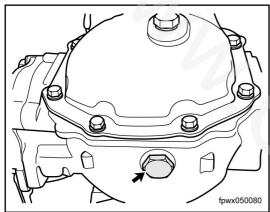
4. Unscrew the front main reducer drain plug and drain the gear oil.
