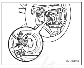
Dismantle horn button assembly and disconnect the driver's SRS assembly connector.
