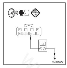
(b) Use multimeter to measure the resistance between stitch 13of connector J007 of lock assy of left front door and the ground.
