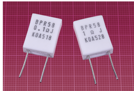
Figure 30-6 Two current resistors manufactured by KOA Speer. Left: 0.1 ohms, 5W, 5%. Right: 1 ohm, 5W, 5%. The background grid is in millimeters.
