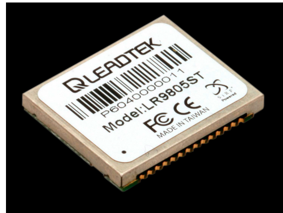
Figure 1-1 A GPS sensor. This surface-mount chip is hidden beneath a metal shield.
