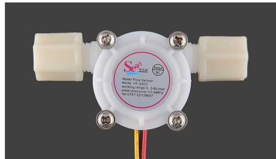
Figure 16-3 An inline flow sensor rated for 3 to 6 liters per minute.
