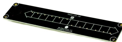
Figure 13-6 Multiple capacitive touch pads arrayed as a strip, made by GHI Electronics.
