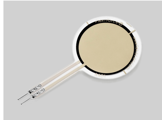
Figure 12-8 A FlexiForce A401 resistive film sensor made by Tekscan, Inc. Its sensing area is 25.4mm in diameter (1 inch) and is rated to measure up to 111N (25lbs).
