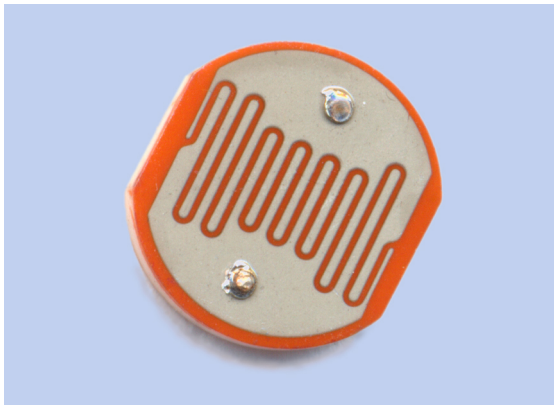
Figure 20-2 Closeup of a photoresistor. Two interlocking electrodes are mounted on a brown semiconductor layer.
