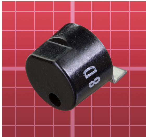
Figure 30-4. Front view of a surface-mount speaker measuring less than 0.4" diameter.
