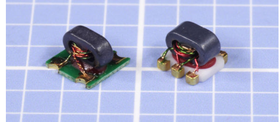
Figure 15-13. Two surface-mount transformers, each measuring less than 0.2" square, typically used in communications equipment and suited for frequencies higher than 5 MHz.
