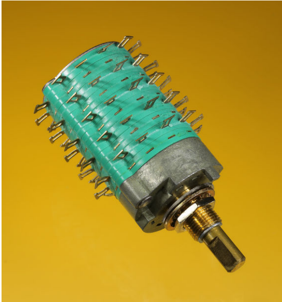
Figure 7-4. A five-pole, twelve-position rotary switch.
