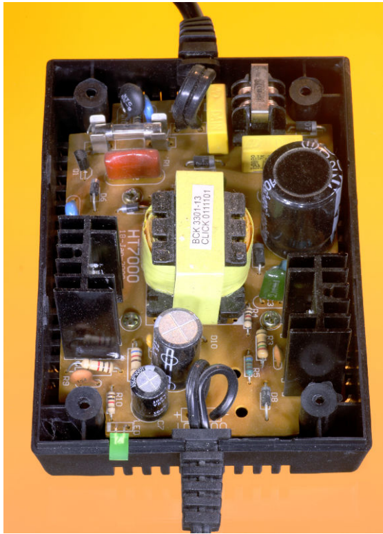
Figure 16-5. The interior of an early switching power supply.
