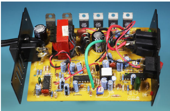
Figure 18-1. The interior components in a 175-watt inverter.
