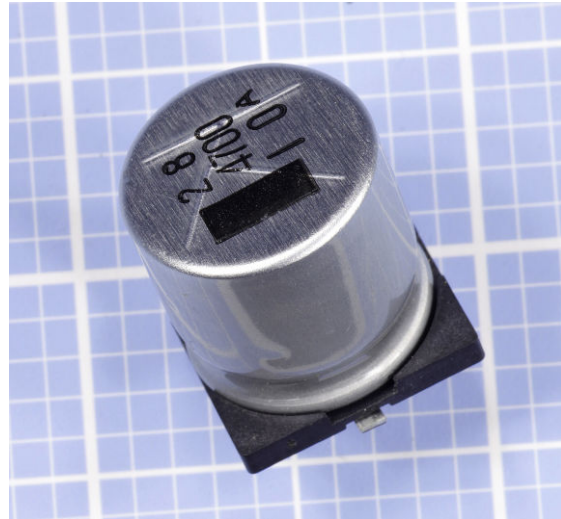
Figure 12-8. Most surface-mount capacitors are as tiny as other surface-mount components, but this 4,700µF electrolytic (at 10V) has a base approximately 0.6" square. A solder tab is visible at the center of the nearest edge.
