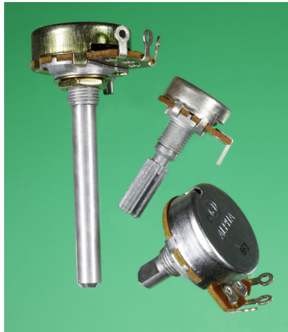
Figure 11-6. Three shaft options for potentiometers.
