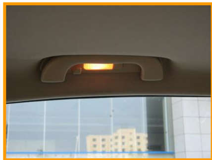
Ceiling handrail light
