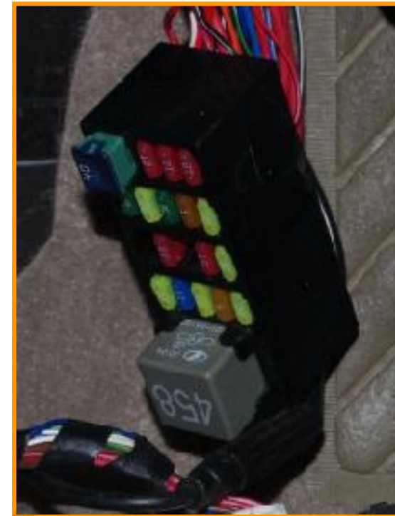
Instrument fuse box
