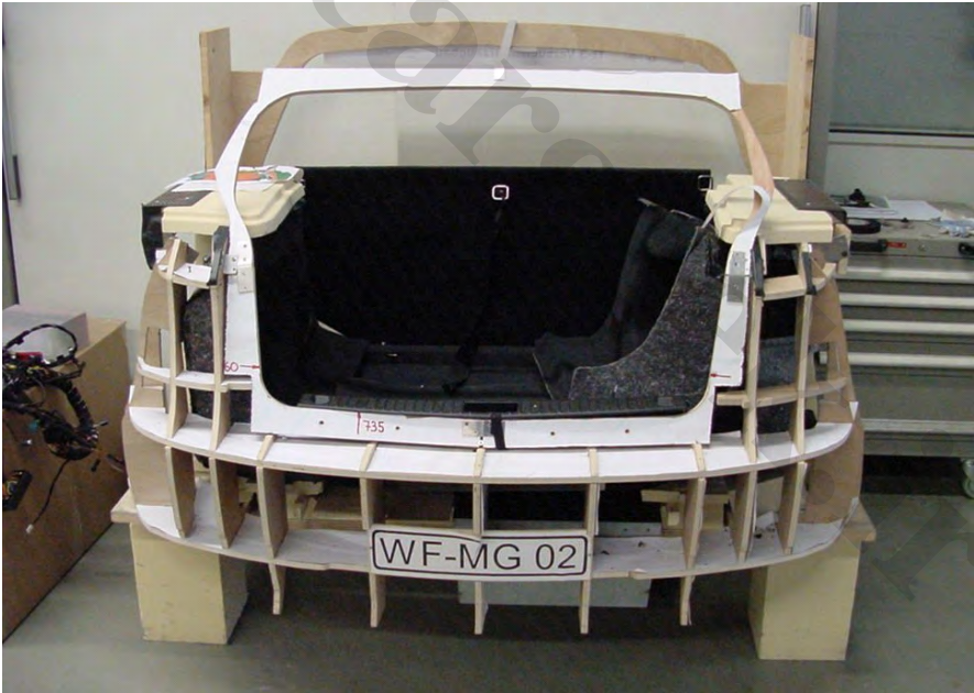
Fig. 7.19 Early concept mock-up for trunk practicality evaluation (Source: BMW)
