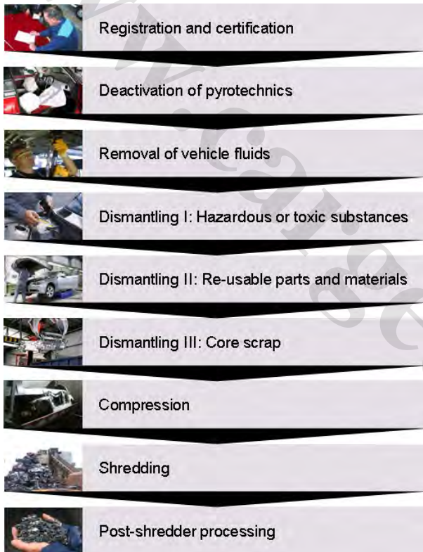
Fig. 7.118 Motor vehicle dismantling procedure (Source: BMW)
