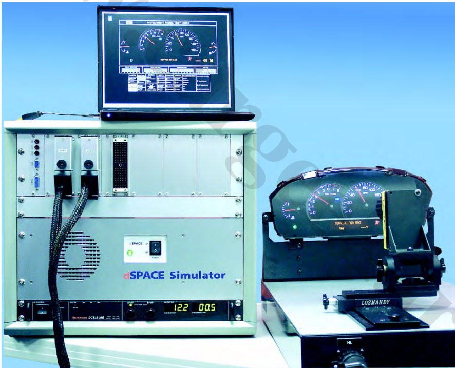
Fig. 5.9 HIL test bench for an instrument panel (Source: dSPACE)
