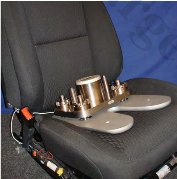
Fig. 7.26 Vibration measurement dummy (Source: WÖLFEL)
