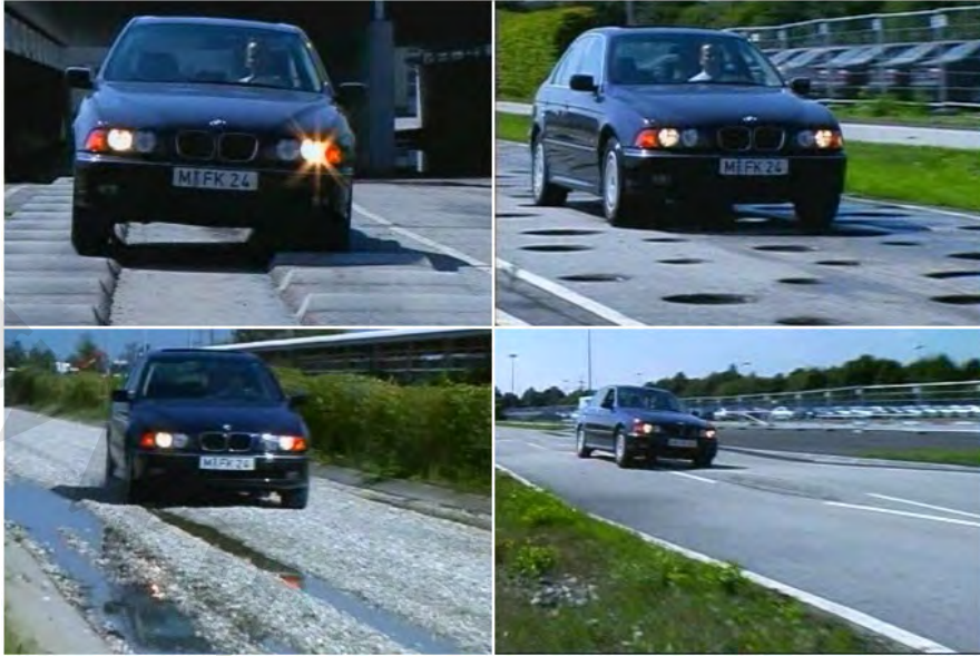
Fig. 7.27 Standardized ride comfort test tracks (Source: BMW)
