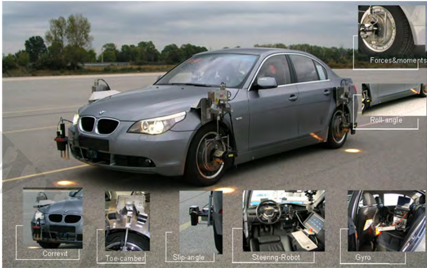
Fig. 7.59 Test vehicle with dynamics measuring equipment (Source: BMW)
