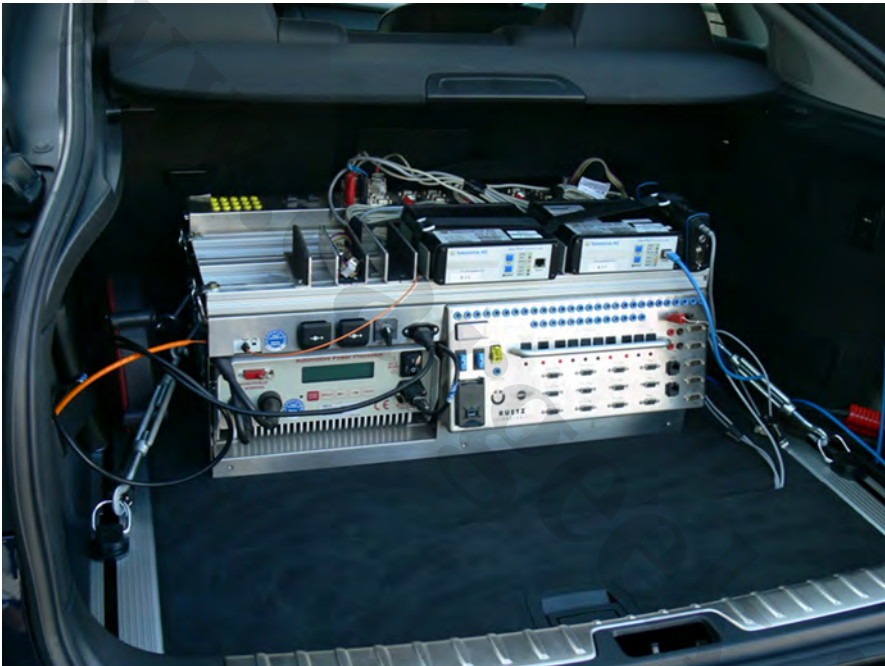
Fig. 5.13 Measuring equipment in a dynamic lab-car (Source: BMW)
