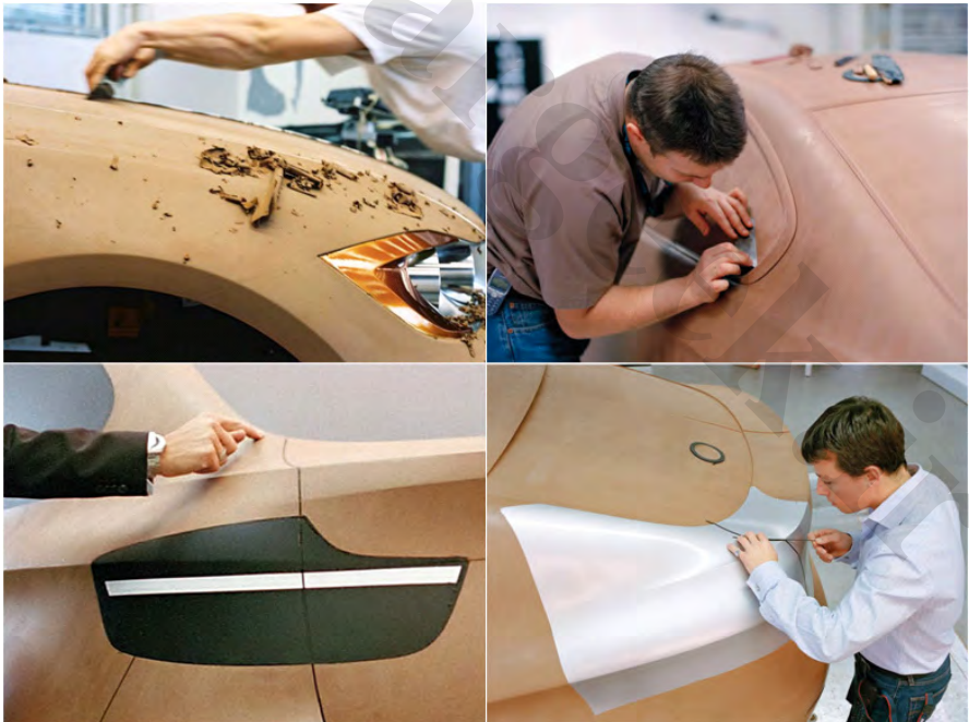
Fig. 7.12 Manufacturing of 1:1 exterior clay models (Source: BMW)
