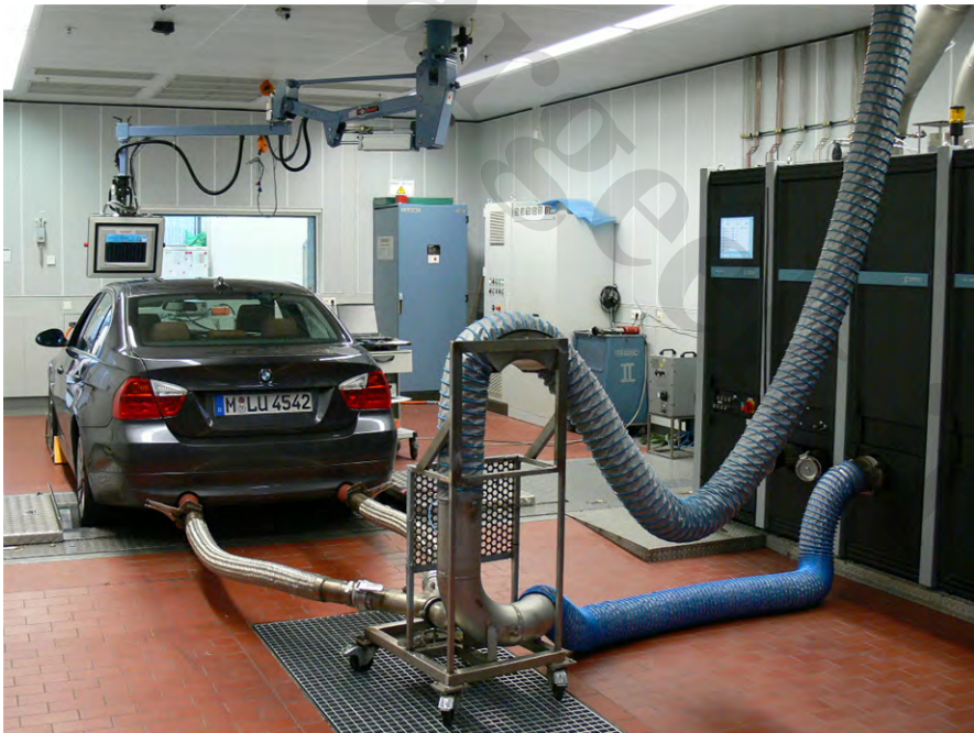
Fig. 7.113 Emissions testing on dynamometer (Source: BMW)
