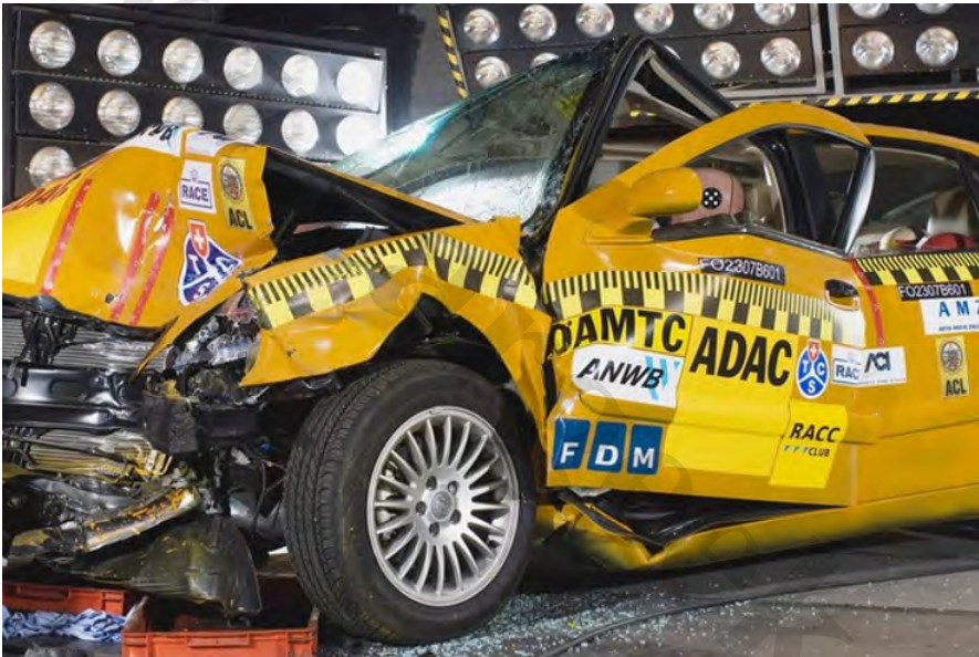
Fig. 7.64 Vehicle with collapsed cabin after Euro NCAP frontal crash (Source: ADAC)
