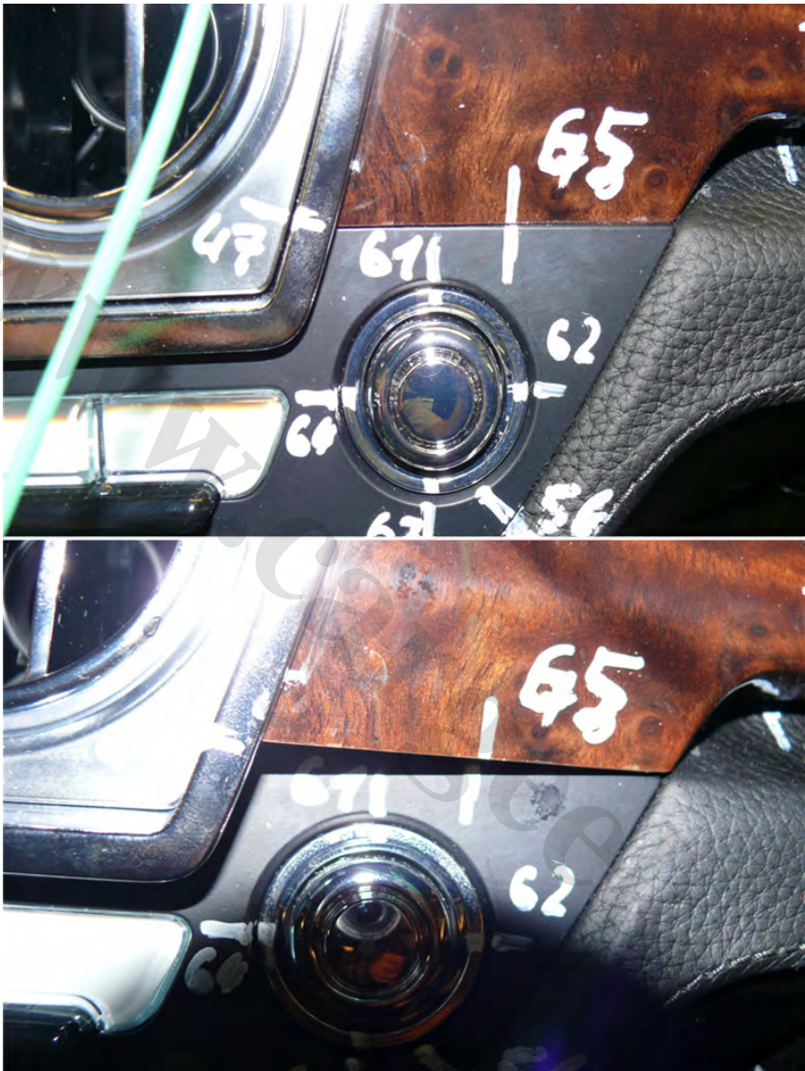
Fig. 7.86 Dashboard before and after sunlight simulation (Source: BMW)
