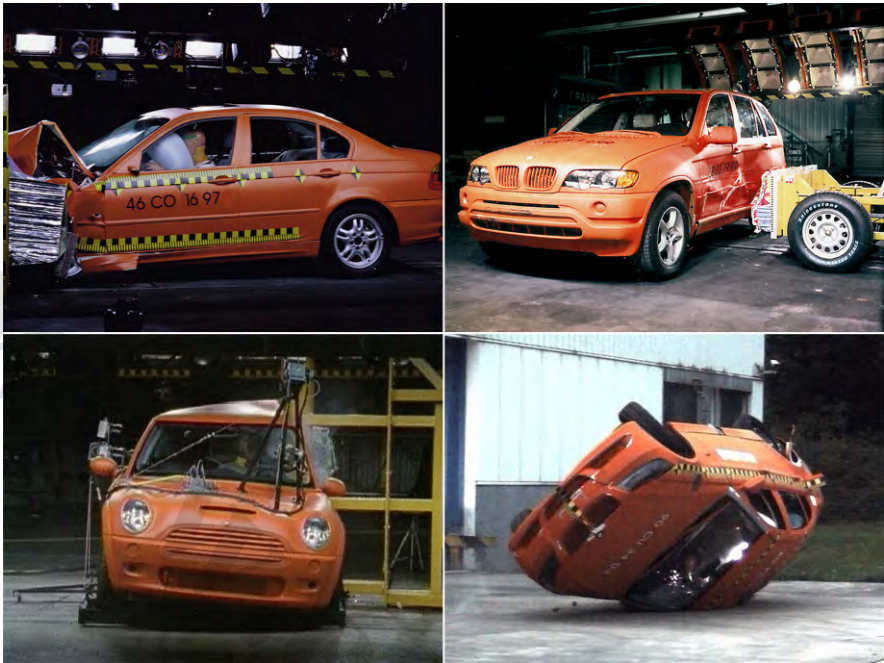
Fig. 7.74 Real crash tests: Frontal impact, side impact, side pole impact, rollover (Source: BMW)
