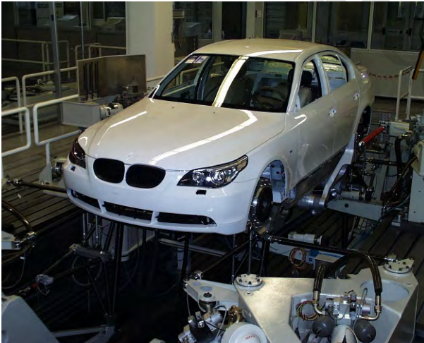
Fig. 7.89 Complete vehicle fatigue test rig (Source: BMW)
