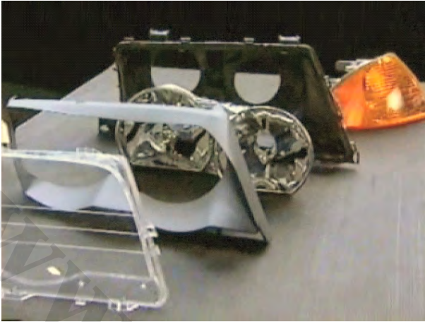
Fig. 7.120 Single-material variety components of a dismantled headlight (Source: BMW)
