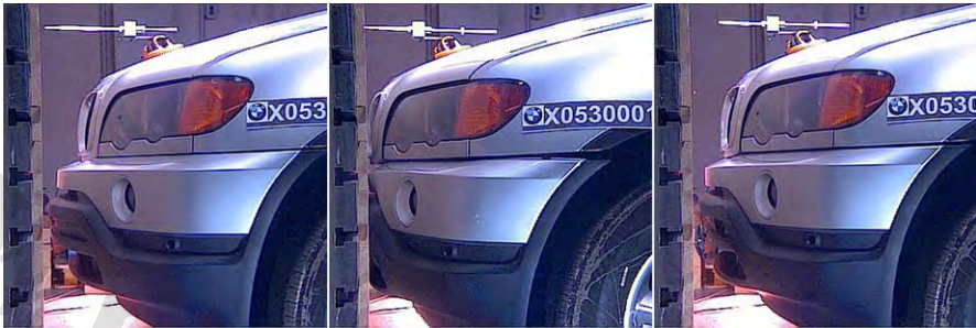
Fig. 7.67 Front bumper before, during, and after a low speed frontal collision (Source: BMW)
