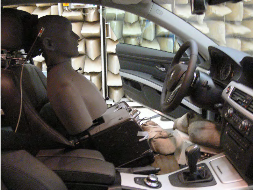
Fig. 7.21 Vehicle sound recording using an artificial head (Source: BMW)
