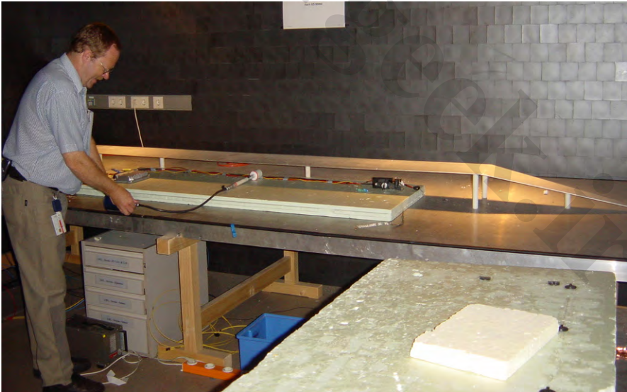
Fig. 7.82 Strip line immunity test according to ISO 11452-5 (Source: BMW)
