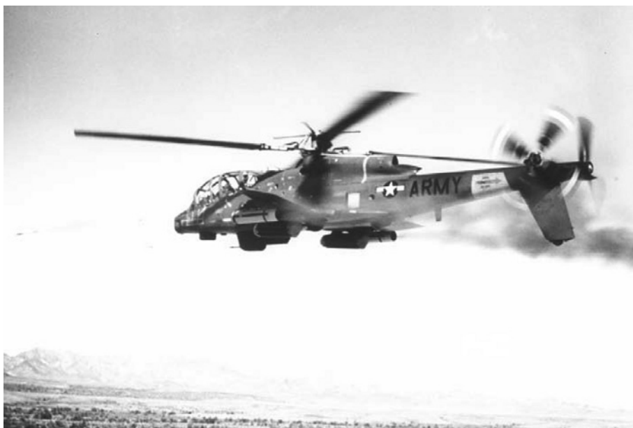
Figure 7.1-12 The Lockheed Cheyenne with fixed-wing, anti-torque rotor and pusher propeller was a very fast, highly manoeuvrable machine. (Lockheed Martin.)
