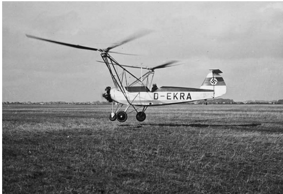
Figure 7.1-1 The Focke-Wulf Fw-61 was the first helicopter to move beyond the experimental stage and was capable of extended flights. The hull was based on that of an Fw Stieglitz aeroplane. Note the vestigial airscrew that simply cools the engine. (Steve Coates.)
