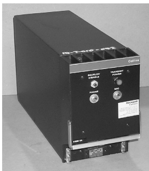
Figure 6.1-21 Aircraft VHF radio removed from its rack mounting.
