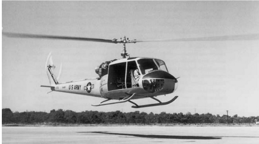
Figure 7.1-8 The Bell Huey was officially designated the Iroquois, but the Helicopter, Utility designation, HU-1, led to the nickname of Huey, which stuck. In Vietnam the Huey was used in enormous numbers. (Bell Helicopter Textron.)
