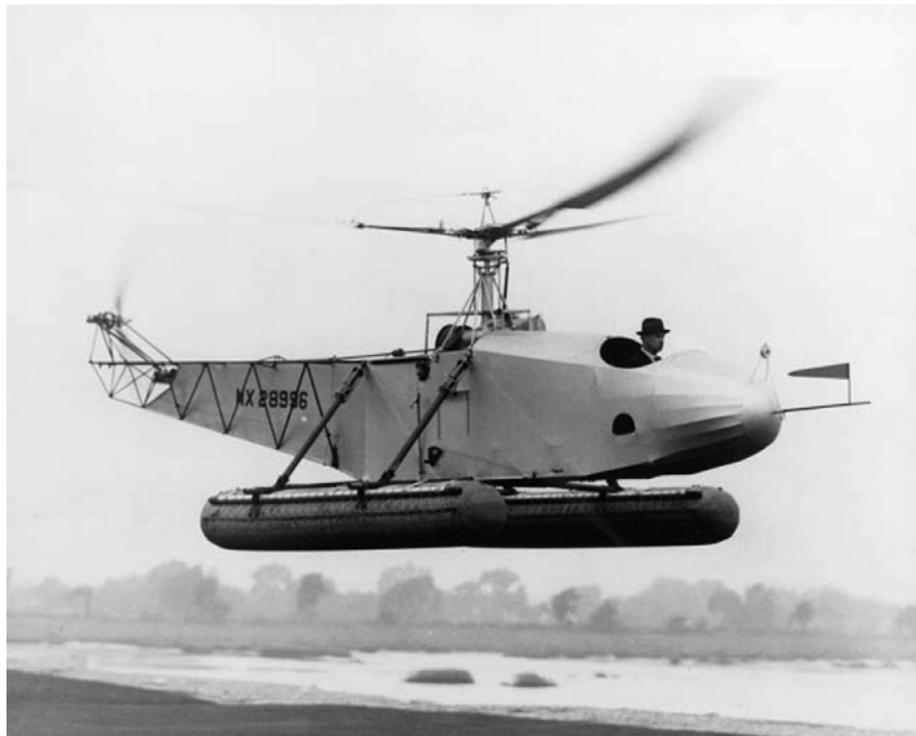
Figure 7.1-3 The Sikorsky VS-300 had an extended development period during most of which cyclic control was not understood and unwieldy auxiliary rotors were used instead. (Igor I. Sikorsky Historical Archives Inc.)
