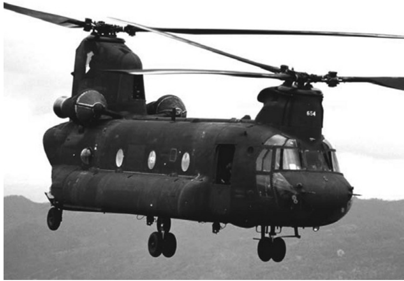
Figure 7.1-16 The Chinook is the definitive tandem rotor helicopter and has been produced in large numbers. (Boeing.)
