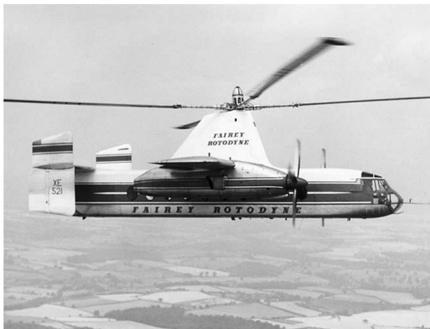
Figure 7.1-13 The Rotodyne hovered as a tip jet powered helicopter and cruised as a compound gyroplane. (AugustaWestland.)
