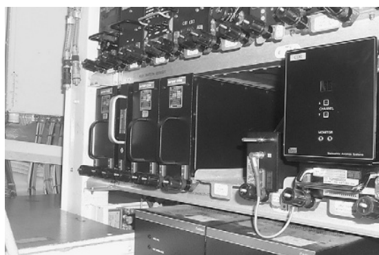
Figure 6.1-18 Three VHF radios (on the extreme left) installed in the aircraft's avionics equipment bay.
