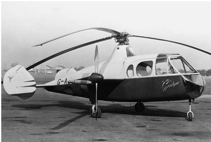
Figure 7.1-11 The Fairey Gyrodyne had a side-mounted anti-torque rotor that became a tractor propeller in forward flight. (AugustaWestland.)
