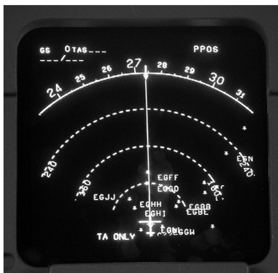
Figure 6.7-9 Airports within the navigation database displayed on the EHSI.
