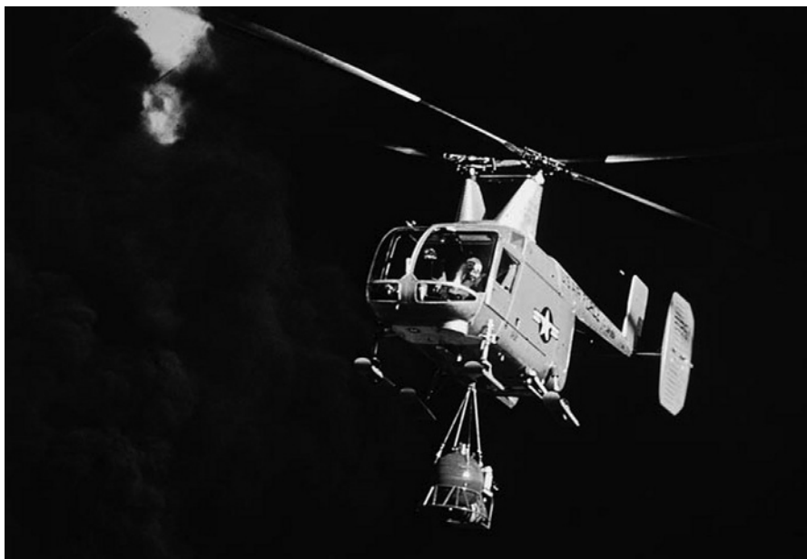
Figure 7.1-17 The Kaman Huskie is the most successful synchropter design. Note the large fin area needed. (Kaman Aerospace.)
