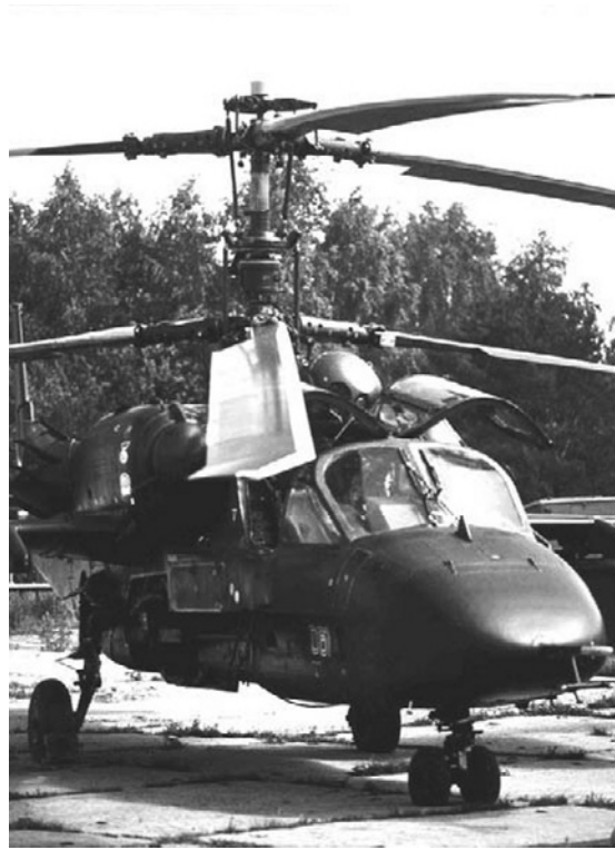
Figure 7.1-18 The contra-rotating coaxial principle is used extensively by Kamov. (Kamov.)
