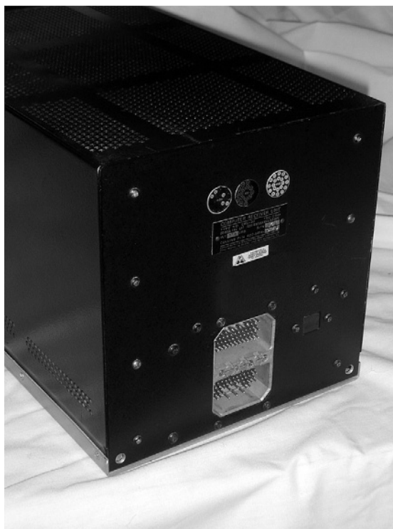
Figure 6.7-8 Program pins located in the computer's connector.
