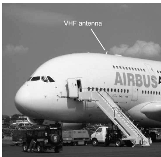
Figure 6.1-25 The forward quarter-wave VHF blade antenna on the Airbus A380.
