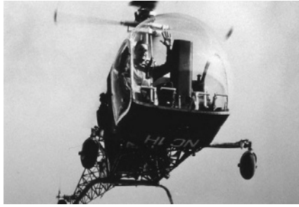
Figure 7.1-6 The legendary Bell 47 was based on Arthur Young's research and was the first helicopter to be certified in the USA. Larry Bell never liked the utilitarian appearance, but it outsold all of the more stylish models. The flybar stabilization system was adopted extensively in later Bell machines. (Bell Helicopter Textron.)
