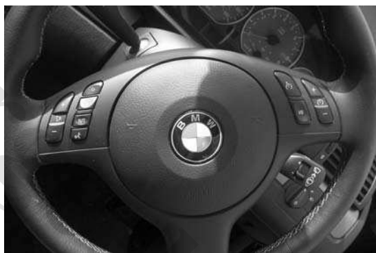
Figure 9.63 Supplementary restraint system (SRS) – an air bag is incorporated in this steering wheel
