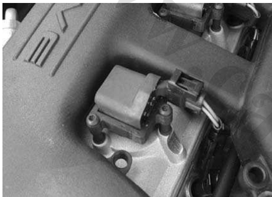
Figure 4.35 Direct ignition coils in position
