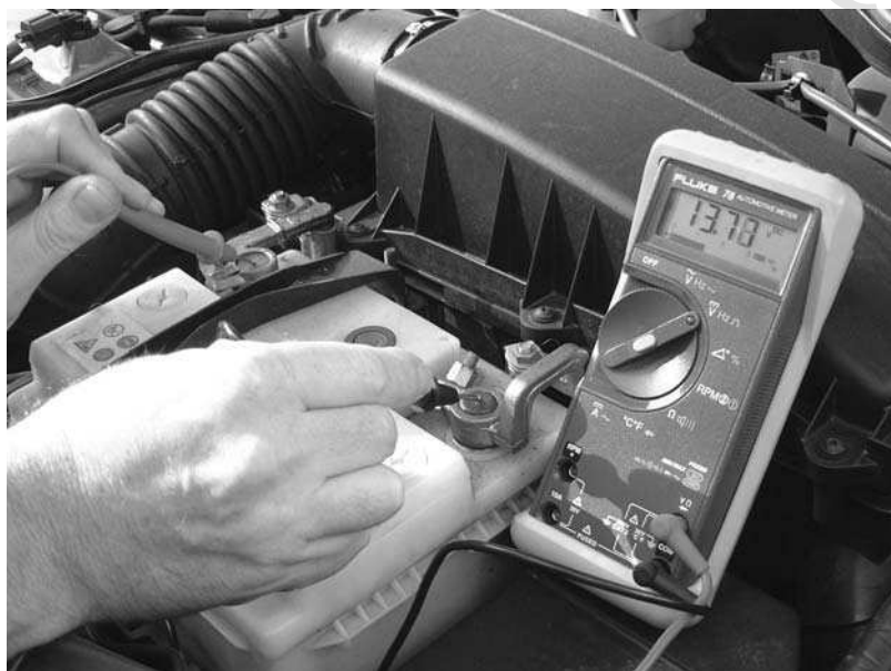
Figure 7.57 Battery voltage testing
