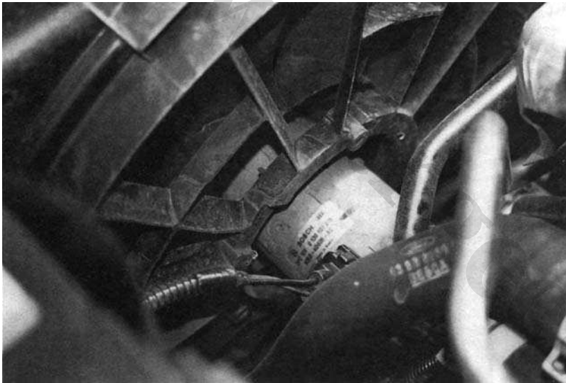
Figure 9.23 Cooling fan motor
