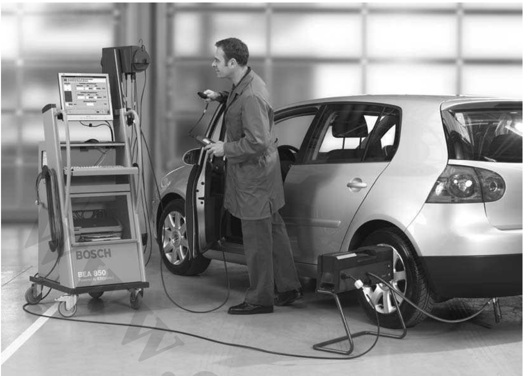
Figure 7.9 Exhaust gas analyser
