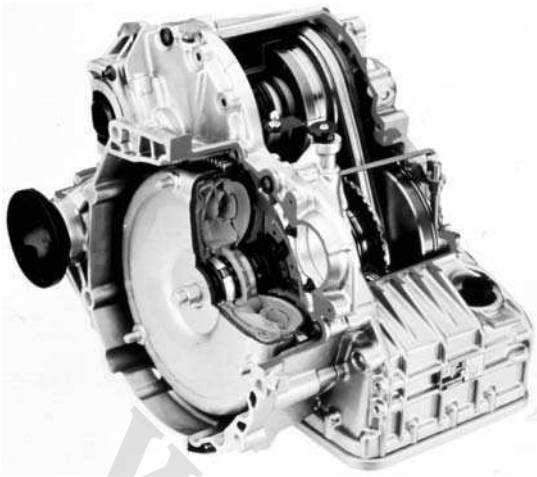
Figure 10.7 This cut-away gearbox shows the torque converter components
