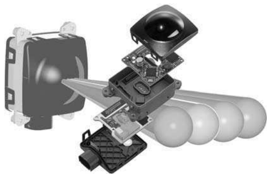
Figure 9.60 Headway sensor and control electronics
