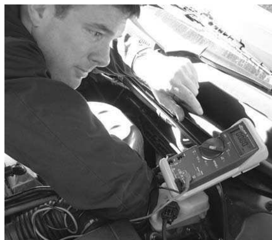
Figure 9.56 Circuit voltage testing
