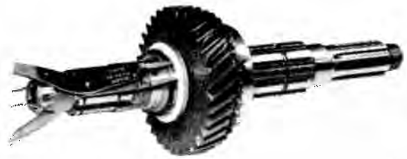
Fig. 6-31 Second-Speed Gear and Washer Installation
