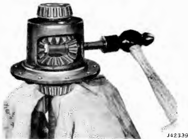
Fig. 10-51 Installing Cross Pin
