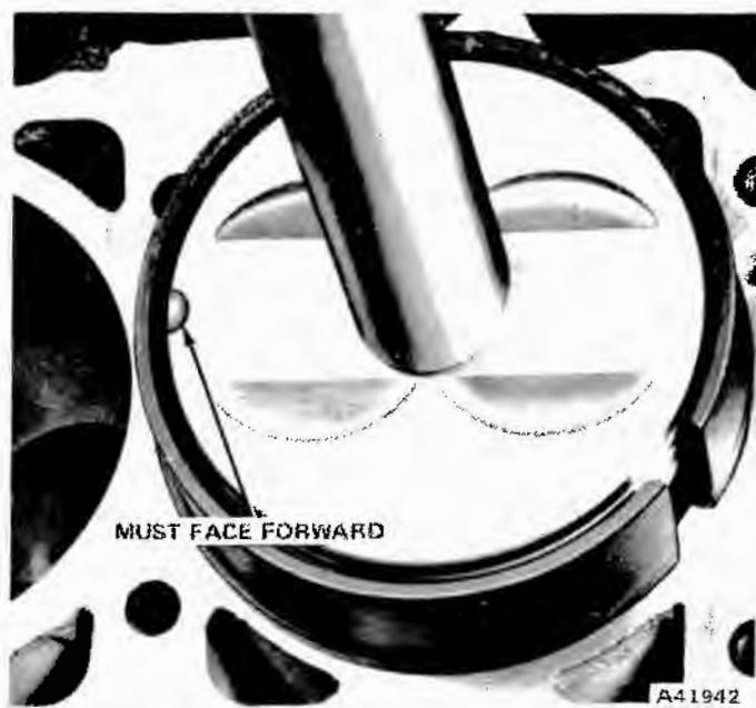
Fig. 1B-33 Installing Piston Assembly Into Bore
