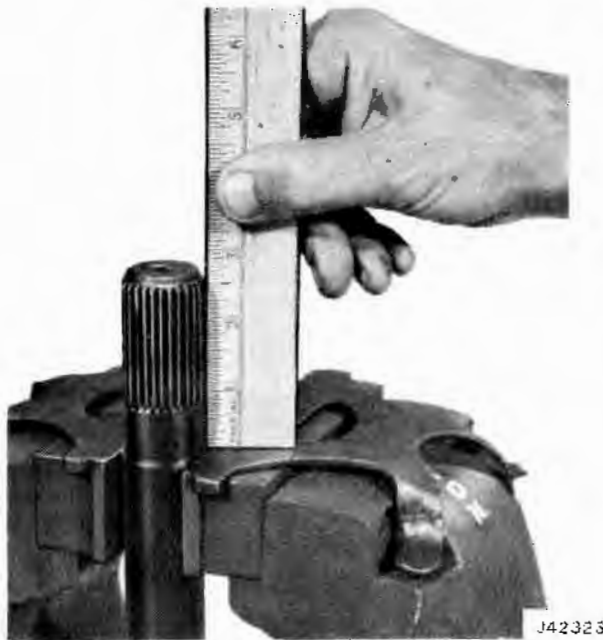
Fig. 10-35 Axle Shaft Positioned in Vise
