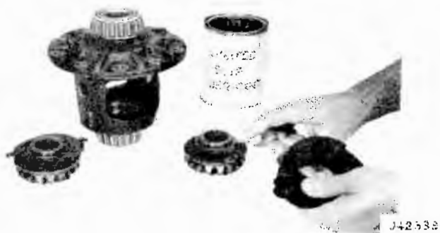
Fig. 10-45 Lubricating Trac-Lok Components
