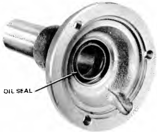
Fig. 6-21 Main Drive Gear Bearing Retainer Oil Seal
