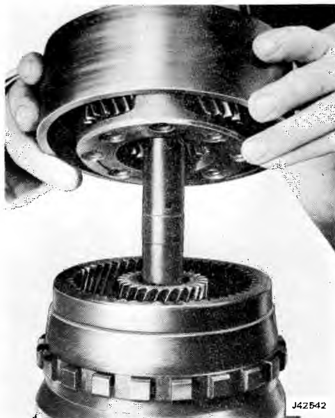
Fig. 7-112 Installing Reaction Carrier Assembly
