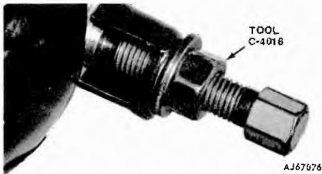
Fig. 11-21 Pivot Pin Removal
