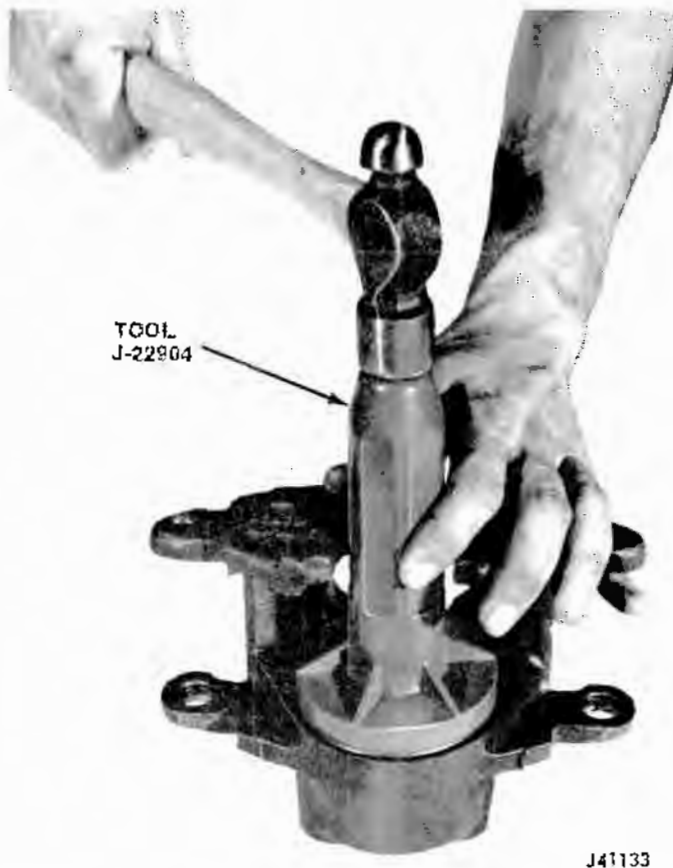
Fig. 9-49 Seating Dust Boot Retainer
