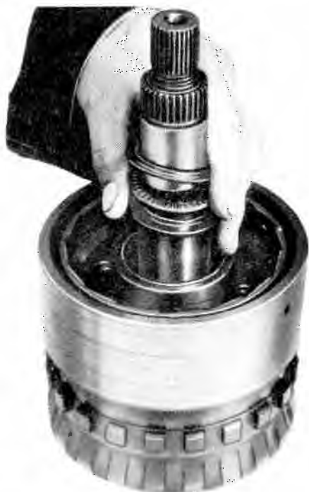
Fig. 7-113 Center Support to Sun Gear Thrust Bearing and Races
