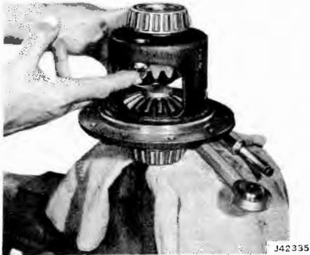
Fig. 10-47 Installing Clutch Pack and Side Gear
