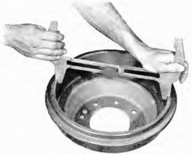
Fig. 9-30 Using Drum-to-Shoe Clearance Gauge
