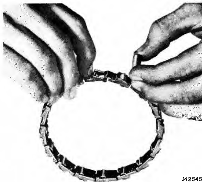
Fig. 7-115 Installing Roller in Roller Clutch
