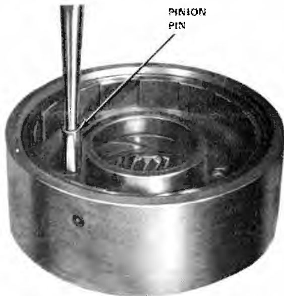
Fig. 7-100 Installing Planet Pinion Pin
