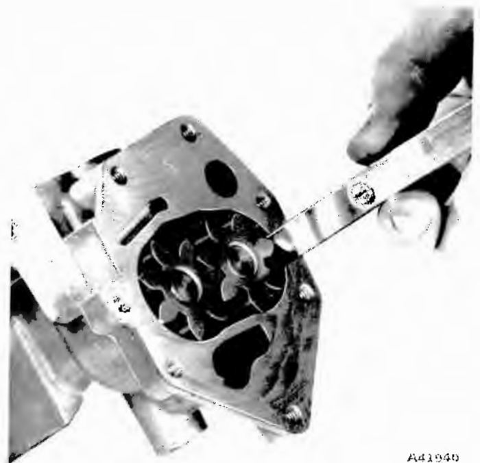
Fig. 1B-27 Gear-to-Body Clearance Measurement
