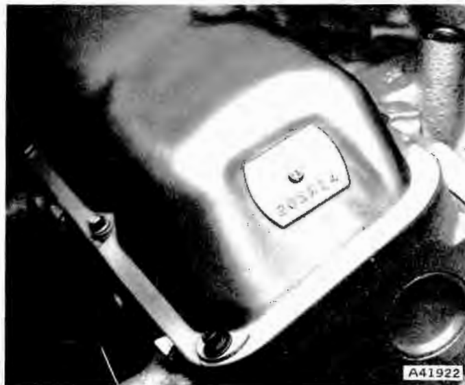
Fig. 1B-3 Build Date Code Location V-8
