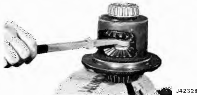
Fig. 10-40 Installing Gear Rotating Tool
