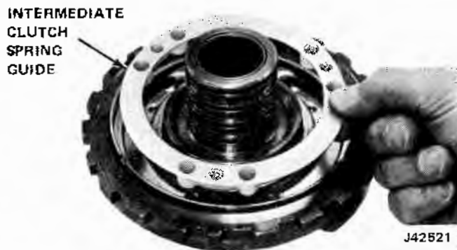
Fig. 7-91 Installing Spring Guide
