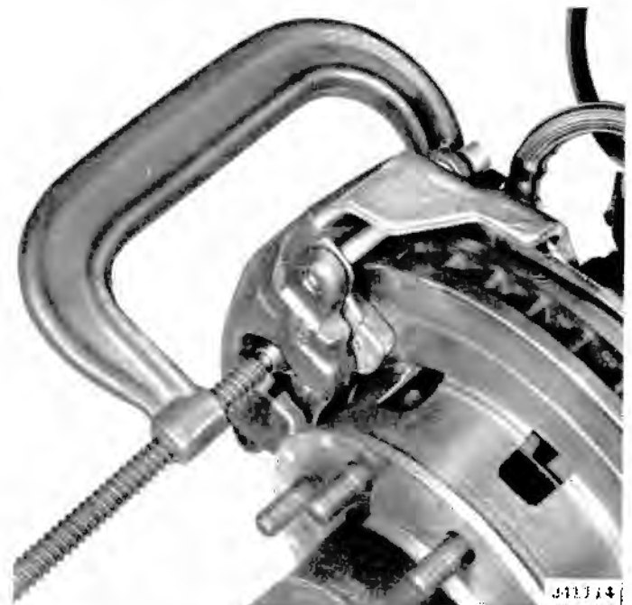
Fig. 9-39 Backing Piston with C-Clamp
