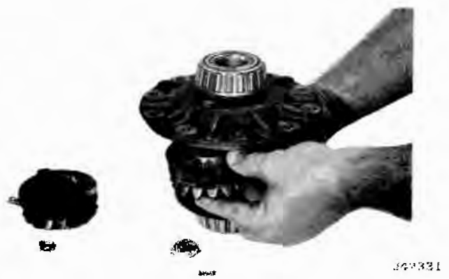
Fig. 10-43 Trac-Lok Unit Disassembly
