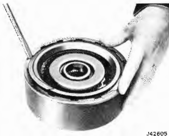
Fig. 7-75 Removing Direct Clutch Snap Ring
