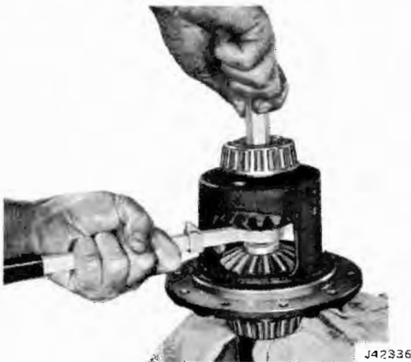
Fig. 10-48 Threading Forcing Screw into Rotating Tool
