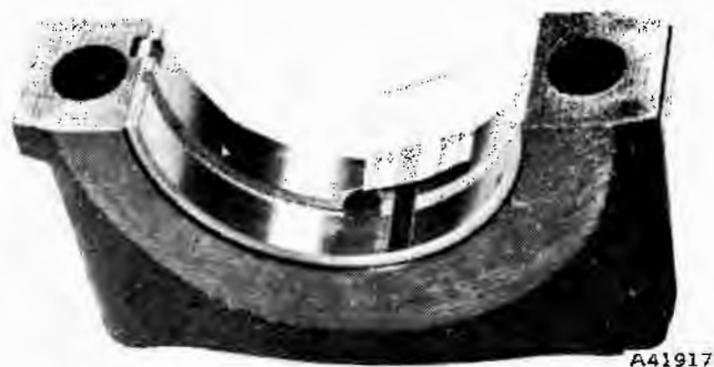
Fig. 1B-42 Main Bearing Clearance Measurement
