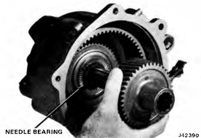
Fig. 8-39 Installing Mainshaft and Sun Gear Assembly
