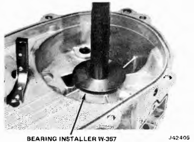
Fig. 8-52 Installing Differential Rear Needle Bearing
