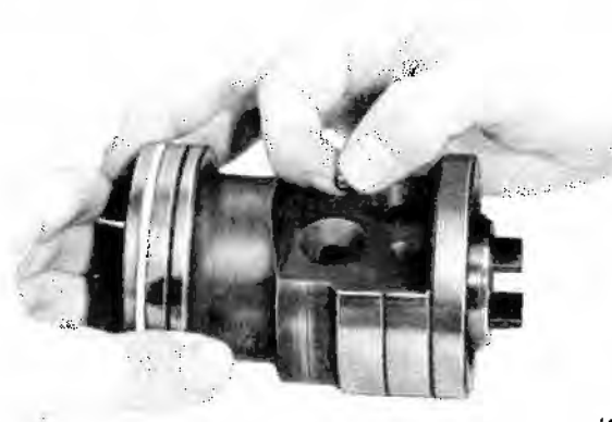
Fig. 11-74 Inserting Balls in Rack-Piston Nut
