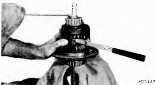
Fig. 10-49 Starting Pinion Mate Gears into Case
