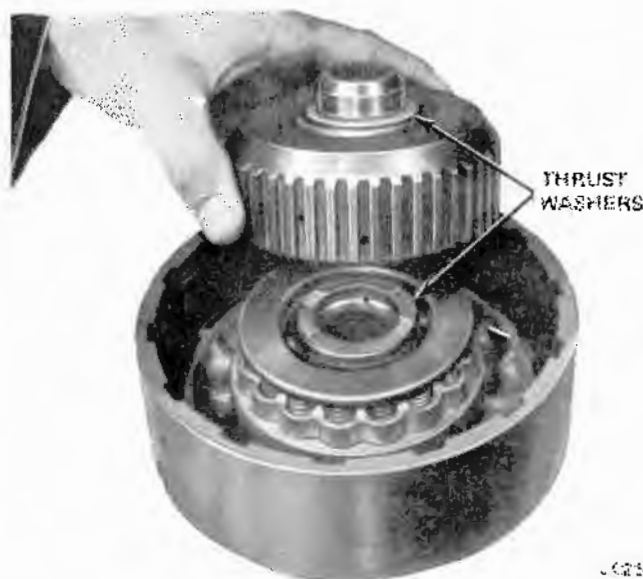
Fig. 7-70 Installing Thrust Washers On Forward Clutch Hub
