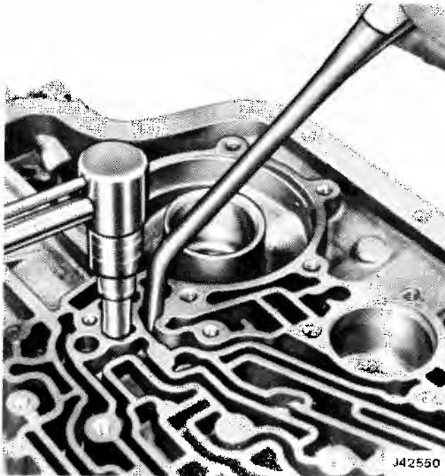
Fig. 7-120 Installing Center Support Screw
