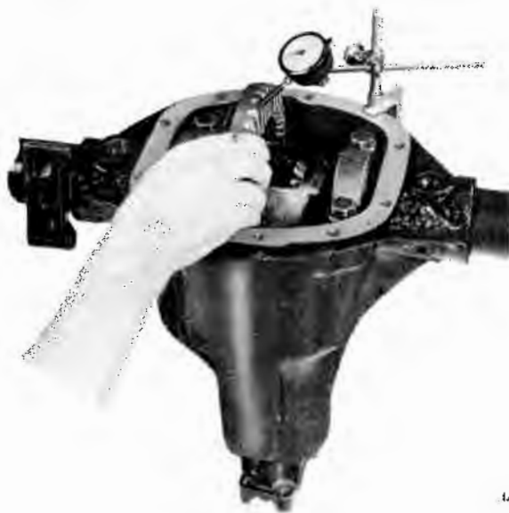
Fig. 10-32 Checking Ring Gear Backlash
