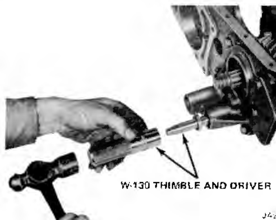
Fig. 8-13 Shift Rail Oil Seal Replacement
