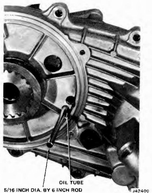
Fig. 8-47 Aligning Oil Tube for Cover Assembly Installation
