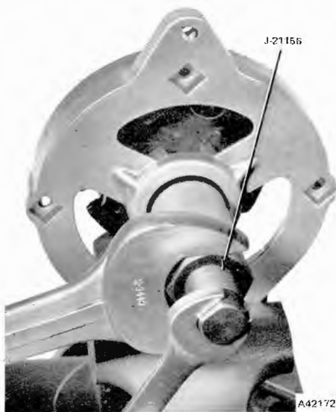
Fig. 3-33 Assembling Front Housing and Rotor
