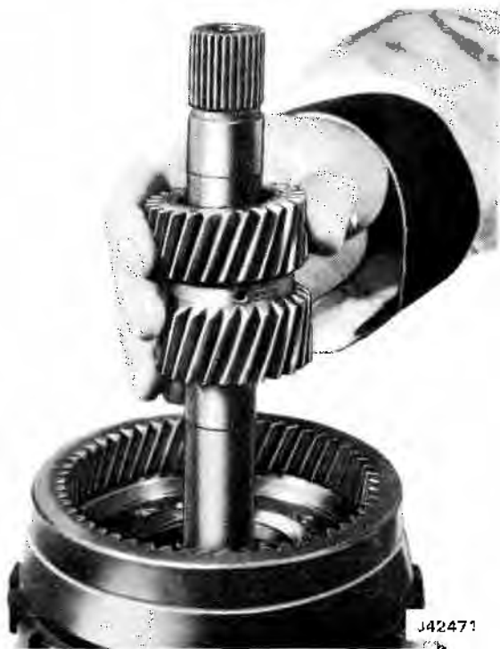
Fig. 7-41 Removing Sun Gear
