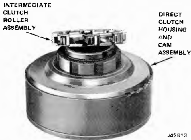
Fig. 7-83 Installing Roller Assembly
