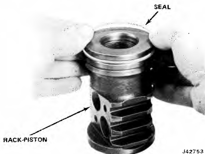
Fig. 11-72 Assembling Seal on Rack-Piston Nut
