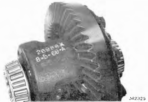
Fig. 10-37 True-Lok Differential Identification
