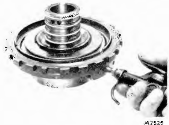
Fig. 7-95 Checking Operation of Intermediate Clutch Assembly
