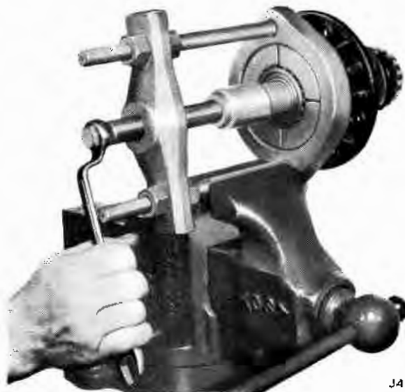
Fig. 10-22 Pulling Differential Side Carrier Bearing
