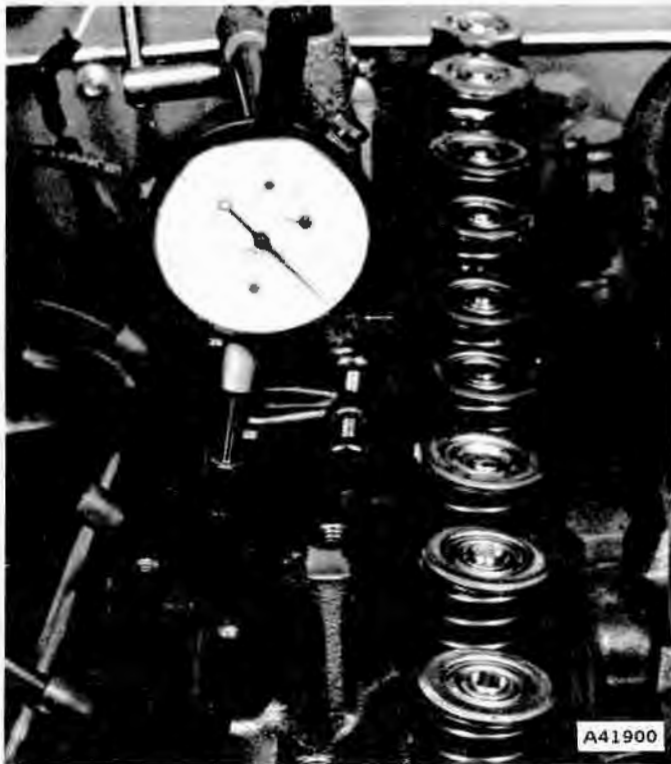
Fig. 1A-30 Cam Lobe Lift Measurement
