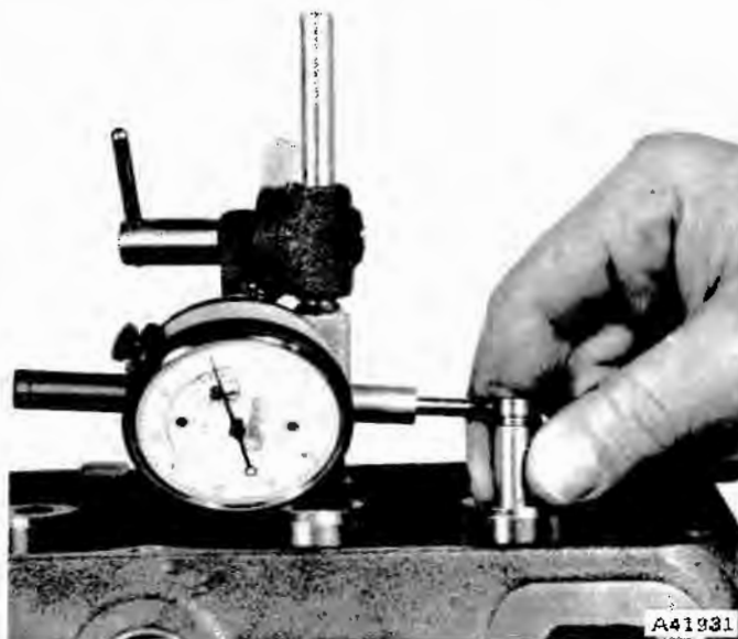
Fig. 1B-15 Valve Stem-to-Guide Clearance Measurement
