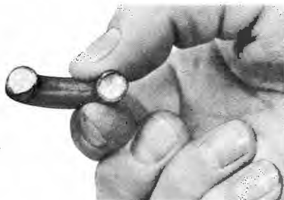
Fig. 11-75 Ball Return Guides Plugged With Grease
