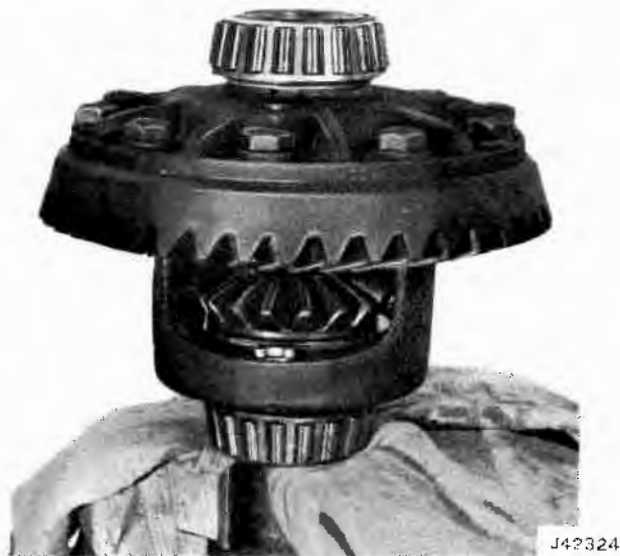
Fig. 10-36 Differential Positioned on Axle Shaft
