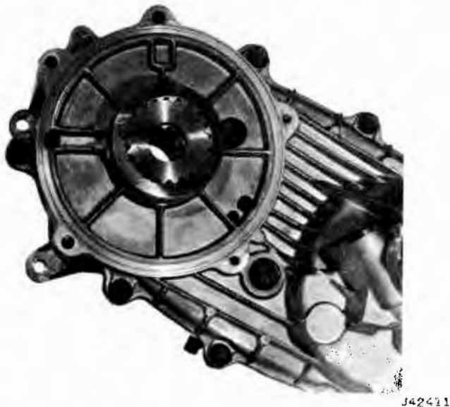
Fig. 8-58 Drive Hub and Sleeve Installed
