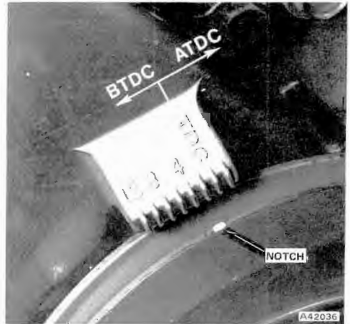
Fig. 4A-46 Timing Mark Location - Six-Cylinder
