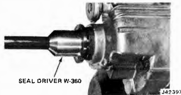
Fig. 8-46 Installing Rear Output Shaft Oil Seal
