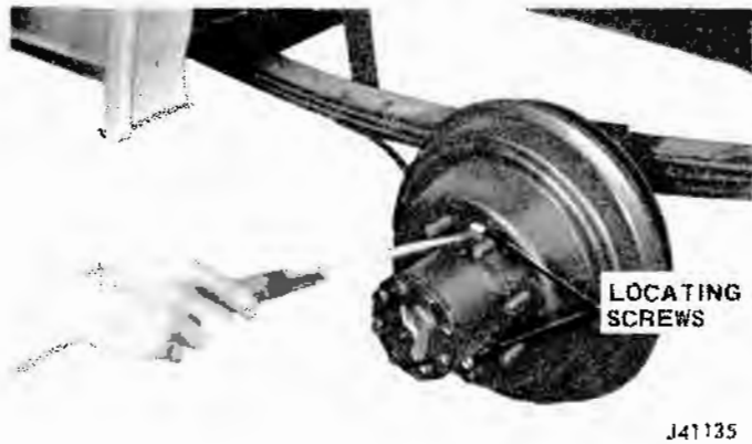
Fig. 9-27 Locating Screw Removal - Model 60 Full Floating Axle
