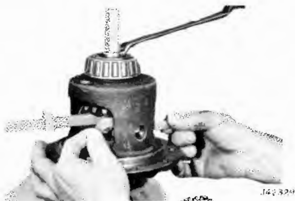
Fig. 10-41 Removing Pinion Mate Washers
