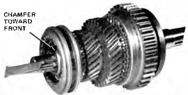
Fig. 6-33 Third- and Fourth-Speed Synchronizer Installation
