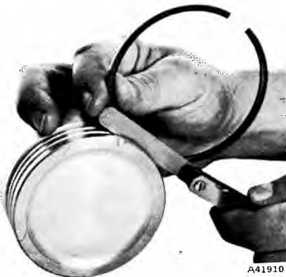
Fig. 1A-40 Ring Side Clearance
