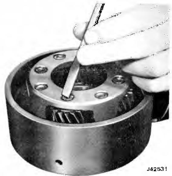
Fig. 7-101 Staking Pinion Pin
