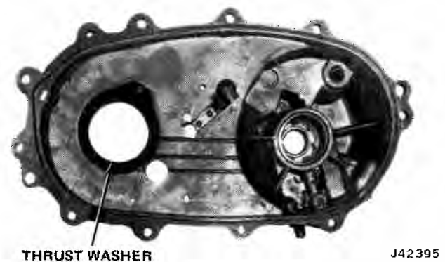
Fig. 8-44 Drive Sprocket Thrust Washer in Position on Case Cover
