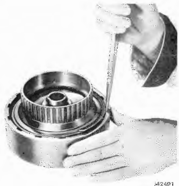
Fig. 7-61 Removing Forward Clutch Housing Snap Ring
