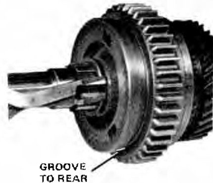
Fig. 6-32 Second-Speed Synchronizer Installation
