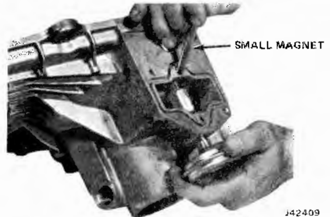
Fig. 8-56 Removing Diaphragm Control
