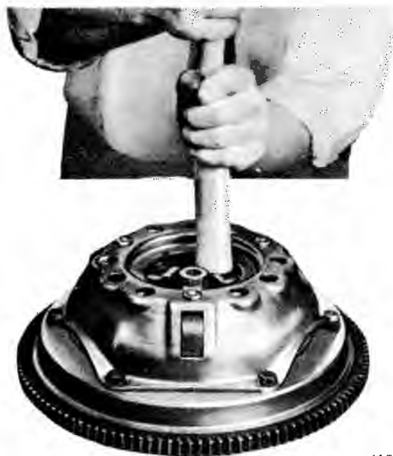
Fig. 5-7 Depressing Clutch Levers
