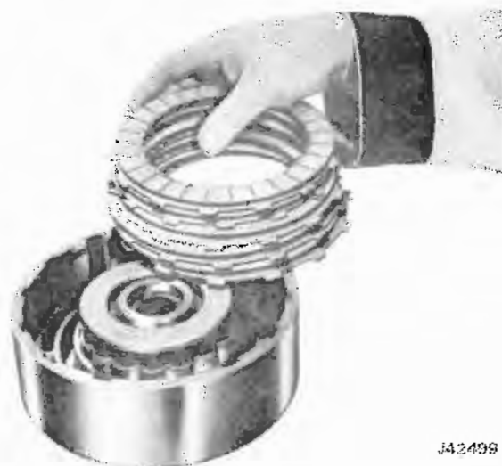
Fig. 7-69 Installing Forward Clutch Plates
