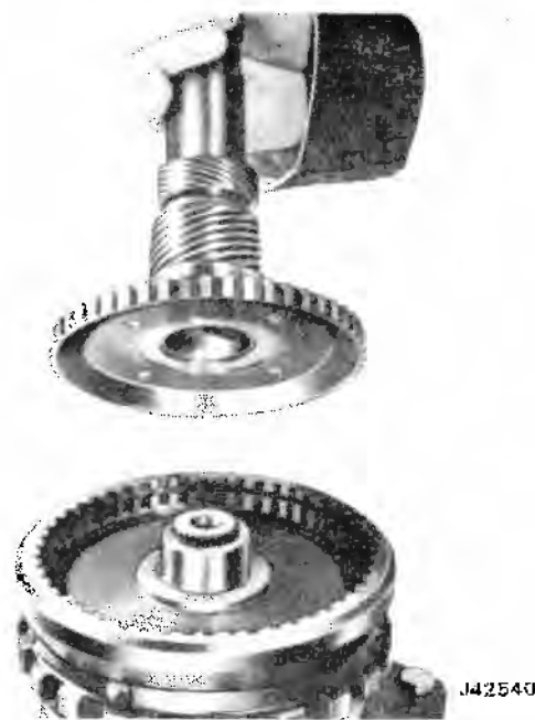
Fig. 7-110 Installing Output Shaft Into Output Carrier Assembly
