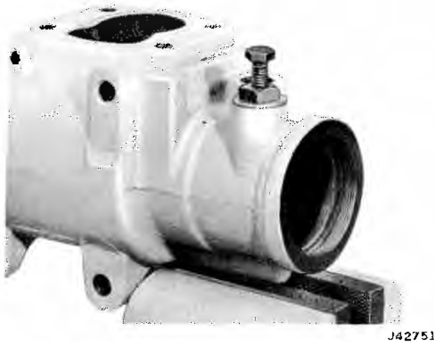
Fig. 11-70 Using Puller Screw to Remove Connector
