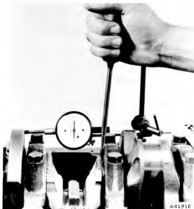
Fig. 1A-46 Crankshaft End Play Measurement
