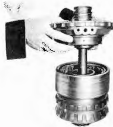
Fig. 7-38 Removing Center Support from Gear Unit
