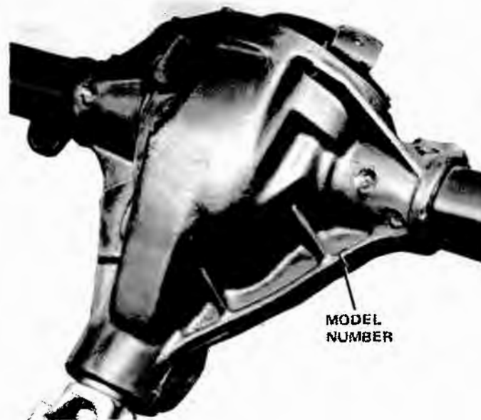
Fig. B-4 Axle Differential Model Number Location
