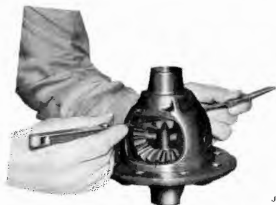
Fig. 10-29 Checking Side Gear Clearance
