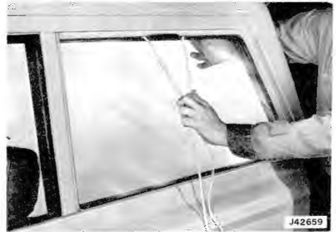
Fig. 15-6 Rear Quarter Window Installation
