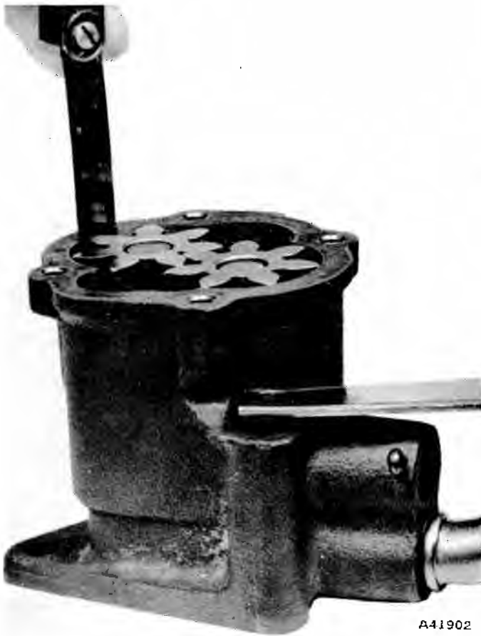
Fig. 1A-33 Oil Gear-to-Body Clearance Measurement
