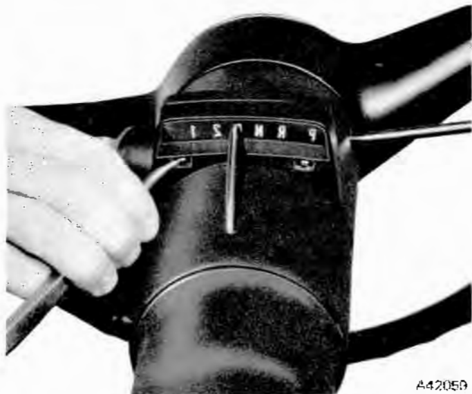
Fig. 11-13 Retainer Clip Removal
