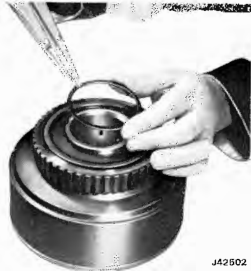
Fig. 7-72 Removing Intermediate Clutch Roller Snap Ring
