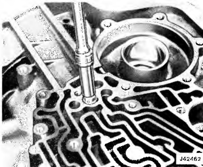
Fig. 7-32 Removing Center Support Bolt
