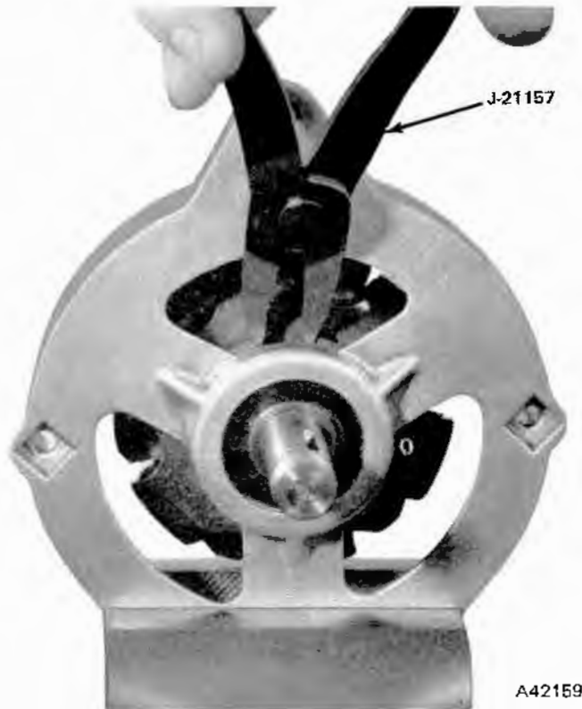
Fig. 3-28 Removing Split Ring Washer
