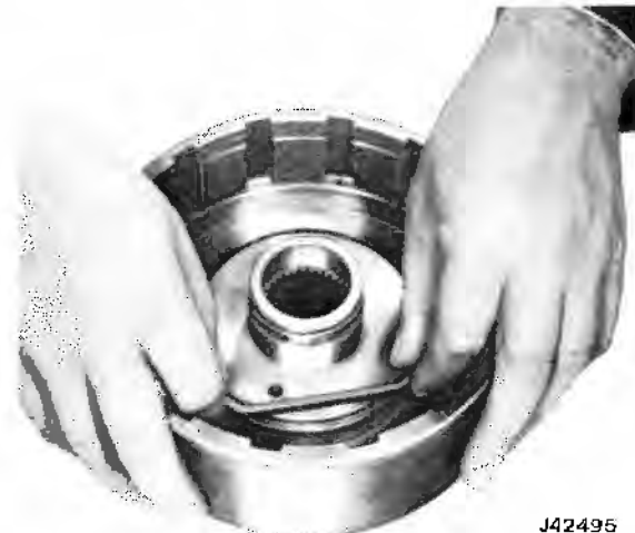
Fig. 7-65 Forward Clutch Housing with Center Piston Seal
