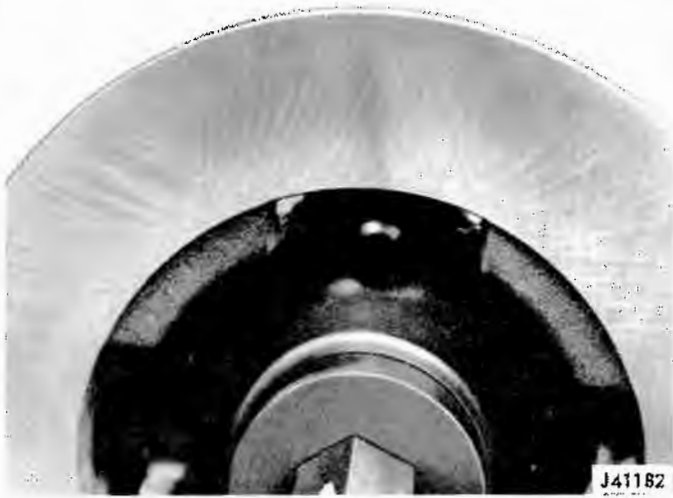
Fig. 9-55 Correct Surface Finish - Non-Directional Cross-Hatch Pattern
