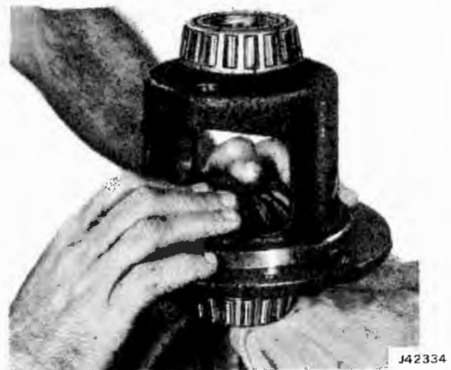
Fig. 10-46 Install Differential Case on Axle Shaft
