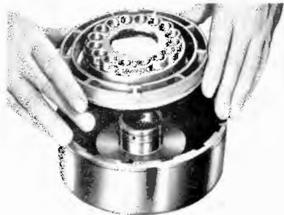
Fig. 7-77 Removing Piston From Direct Clutch Housing
