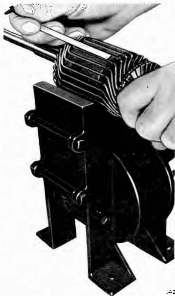
Fig. 3-36 Testing Armature for Shorted Winding
