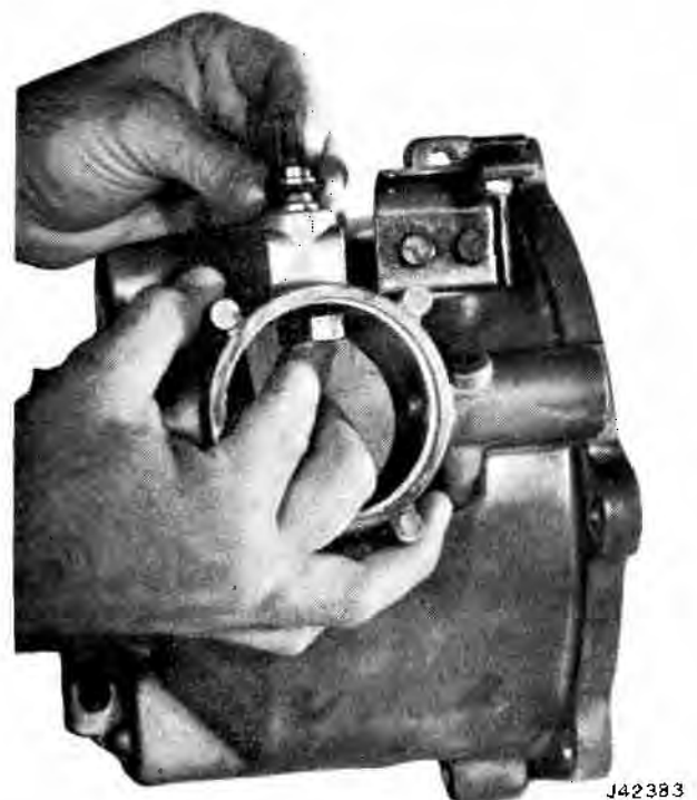
Fig. 8-32 Shift Lever O-Ring Installation
