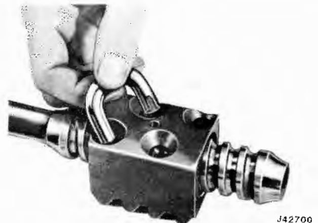
Fig. 11-40 Installing Ball Guides
