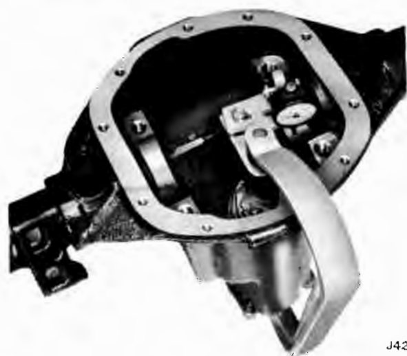
Fig. 10-27 Checking Pinion Adjustment
