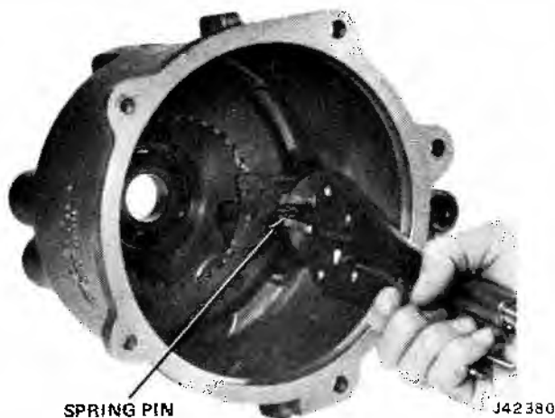
Fig. 8-29 Removing Shift Fork Locating Spring Pin
