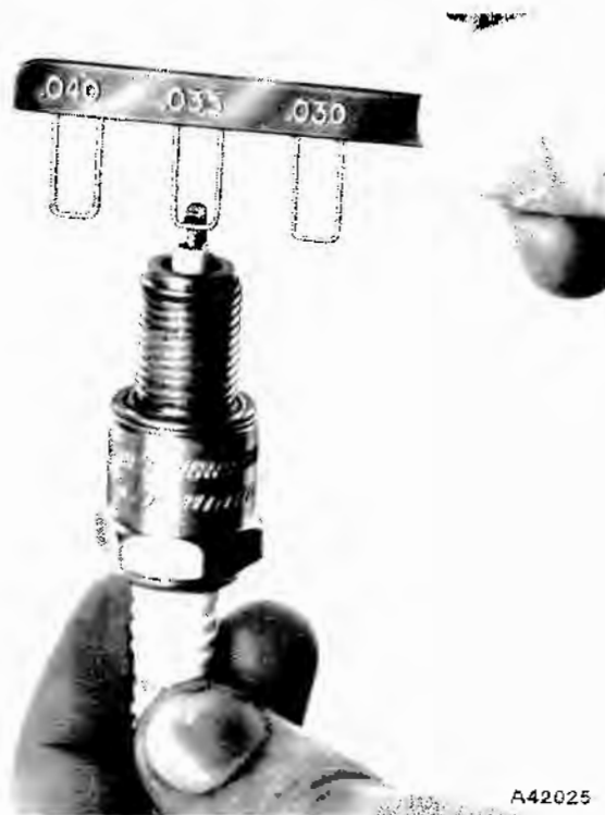
Fig. 4A-35 Spark Plug Gap Check
