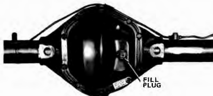
Fig. B-5 Rear Axle Filler Plug Location (Front Axle Similar)
