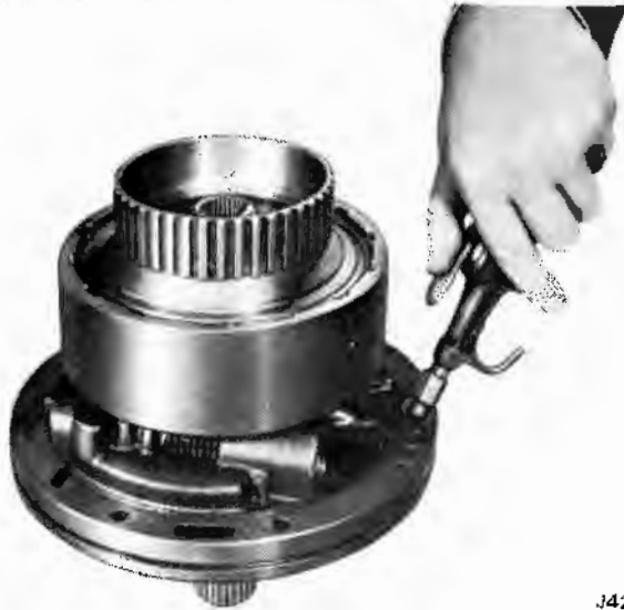
Fig. 7-71 Checking Forward Clutch Operation
