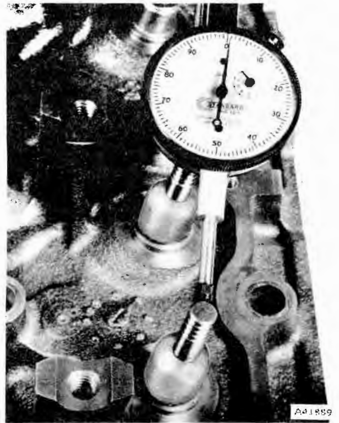
Fig. 1A-17 Checking Stem-to-Guide Clearance
