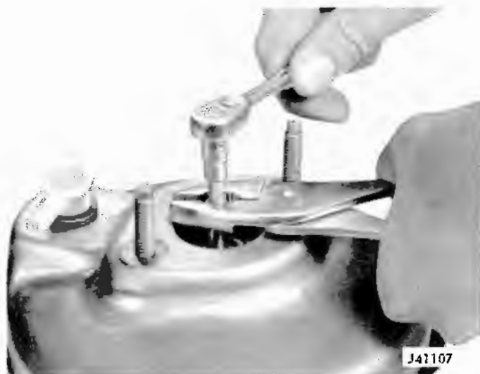
Fig. 9-5 Adjusting Push Rod Length
