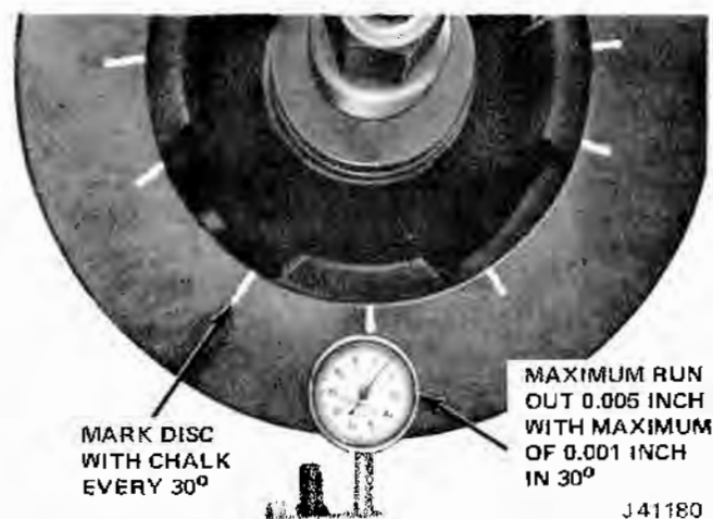
Fig. 9-53 Checking Lateral Runout
