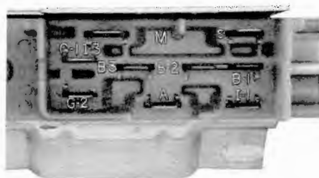
Fig. 3-63 Ignition Switch Terminals
