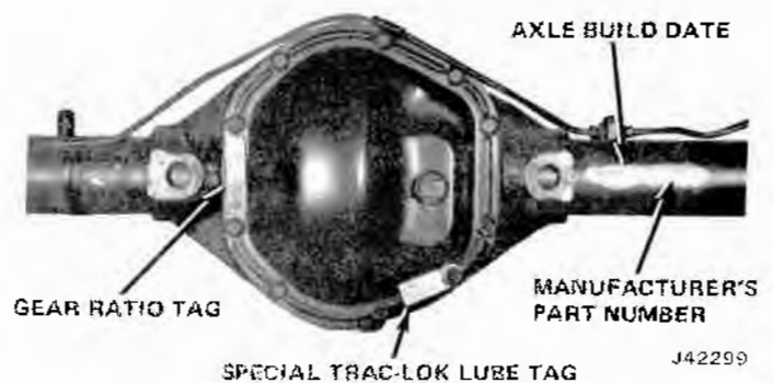
Fig. 10-2 Ratio, Build Date, and Trac-Lok Differential Identification
