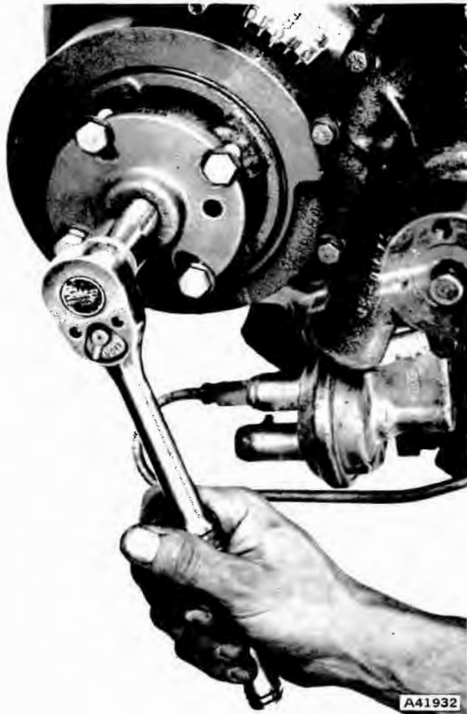
Fig. 1B-19 Vibration Damper Removal
