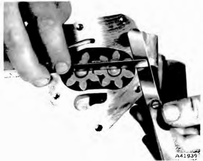
Fig. 1B-26 Gear End Clearance Measurement
