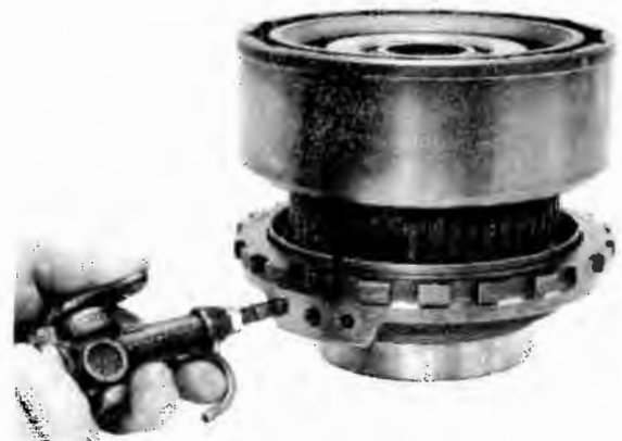
Fig. 7-86 Checking Operation of Direct Clutch Assembly
