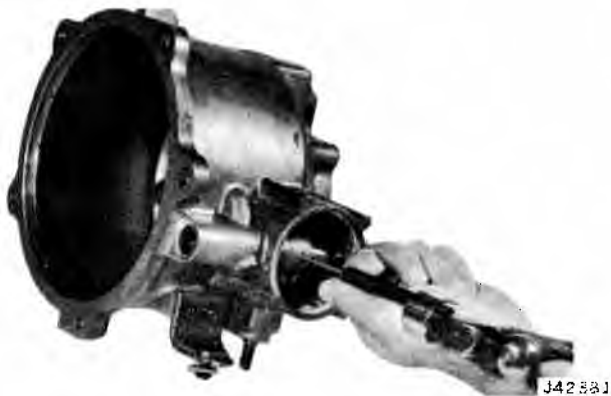
Fig. 8-30 Removing Spring Pin
