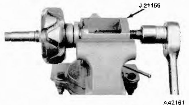
Fig. 3-31 Rear Bearing Removal
