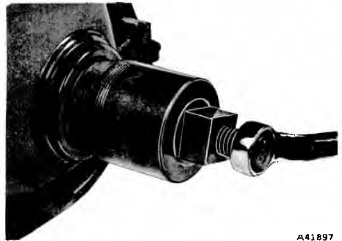
Fig. 1A-27 Timing Chain Cover Oil Seal Removal
