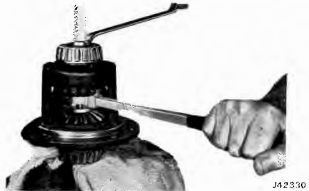
Fig. 10-42 Removing Pinion Mate Gears
