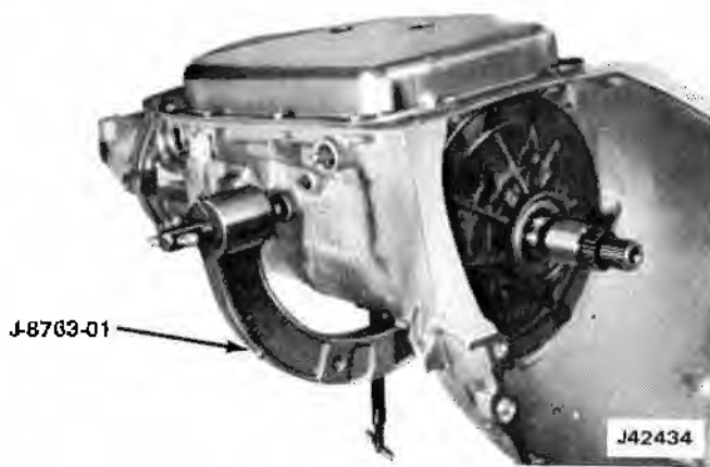
Fig. 7-4 Transmission in Holding Fixture J-8763-01
