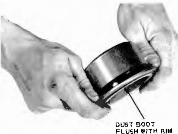
Fig. 9-47 Installing Dust Boot on Piston
