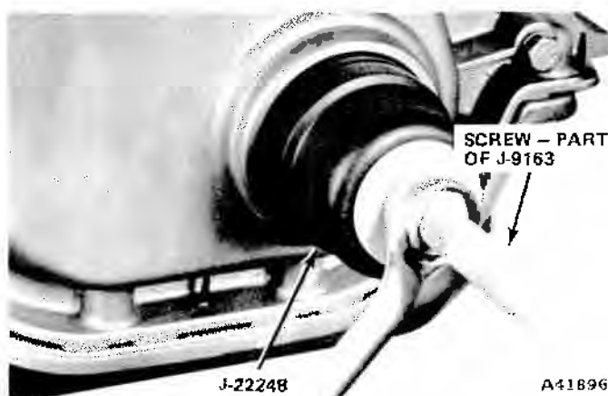
Fig. 1A-26 Timing Chain Cover Oil Seal Installation
