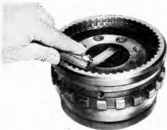
Fig. 7-97 Checking End Play of Pinions in Output Carrier
