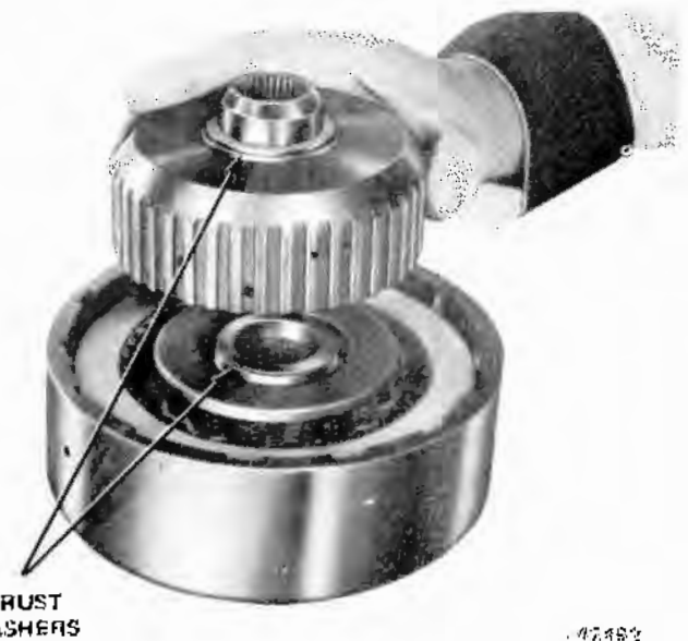
Fig. 7-62 Removing Hub and Thrust Washers From Forward Clutch Assembly
