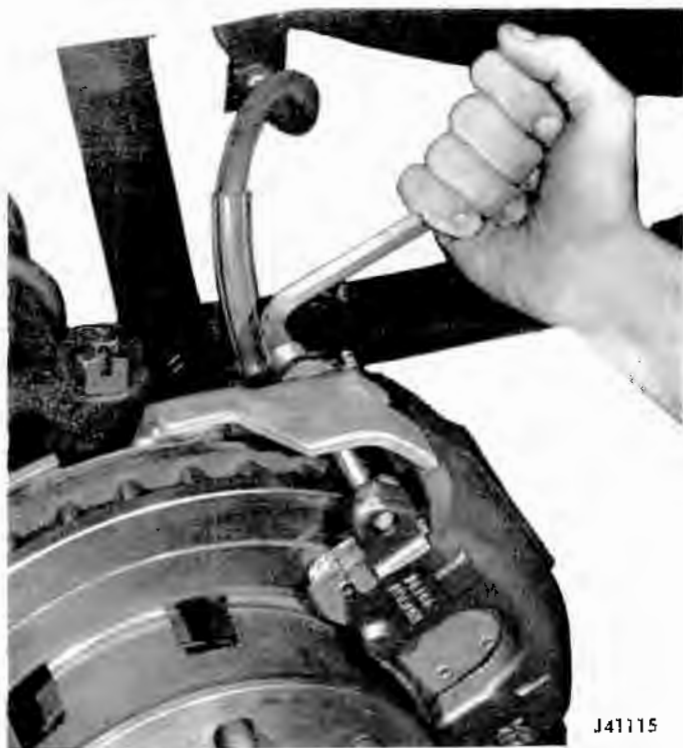
Fig. 9-40 Removal of Caliper Mounting Bolts
