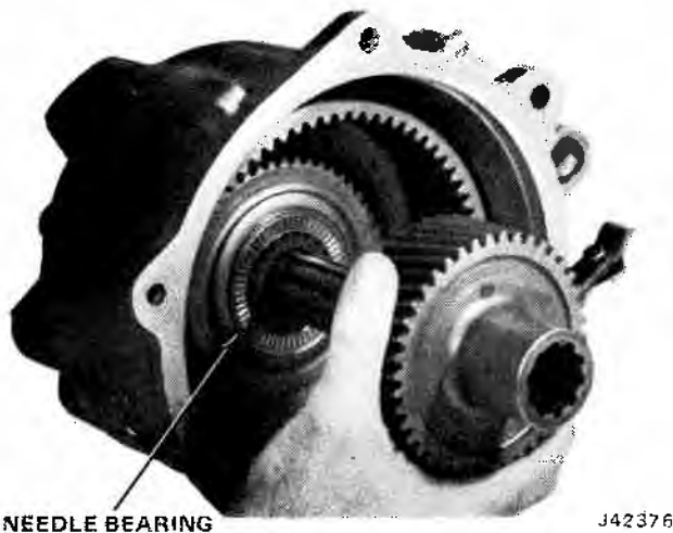
Fig. 8-25 Removing Mainshaft and Sun Gear Assembly
