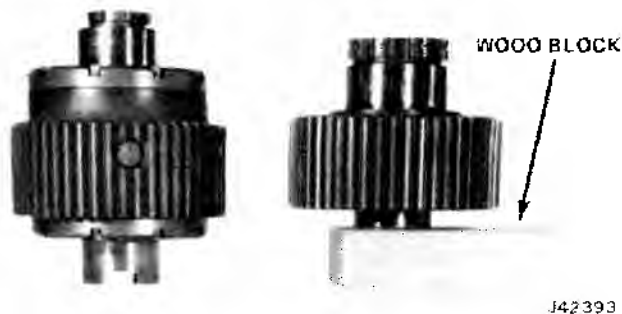
Fig. 8-42 Differential and Drive Sprocket Positioned for Chain Installation
