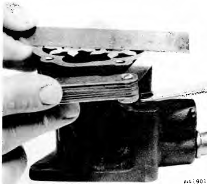
Fig. 1A-32 Oil Pump Gear End Clearance Measurement
