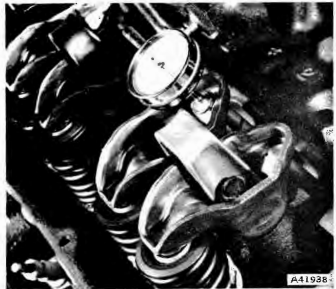
Fig. 1B-25 Cam Lobe Lift Measurement
