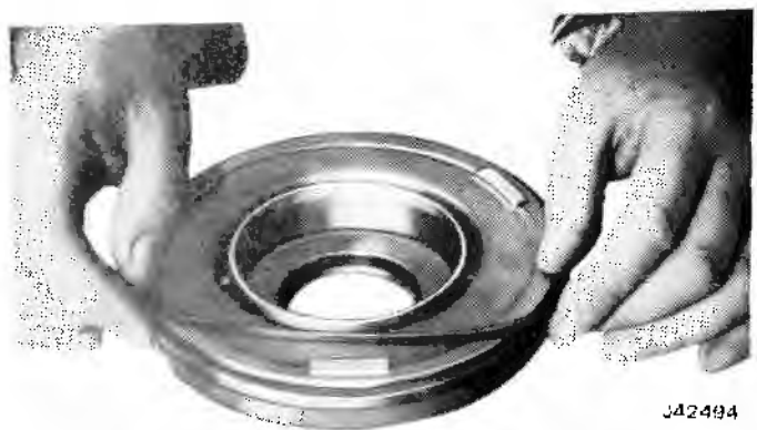
Fig. 7-64 Removing Forward Clutch Piston Outer Seal
