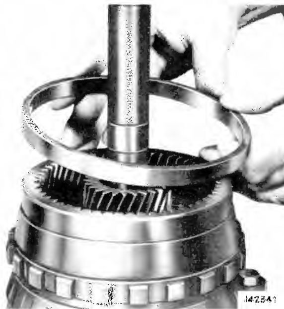
Fig. 7-111 Positioning Front Internal Gear Ring
