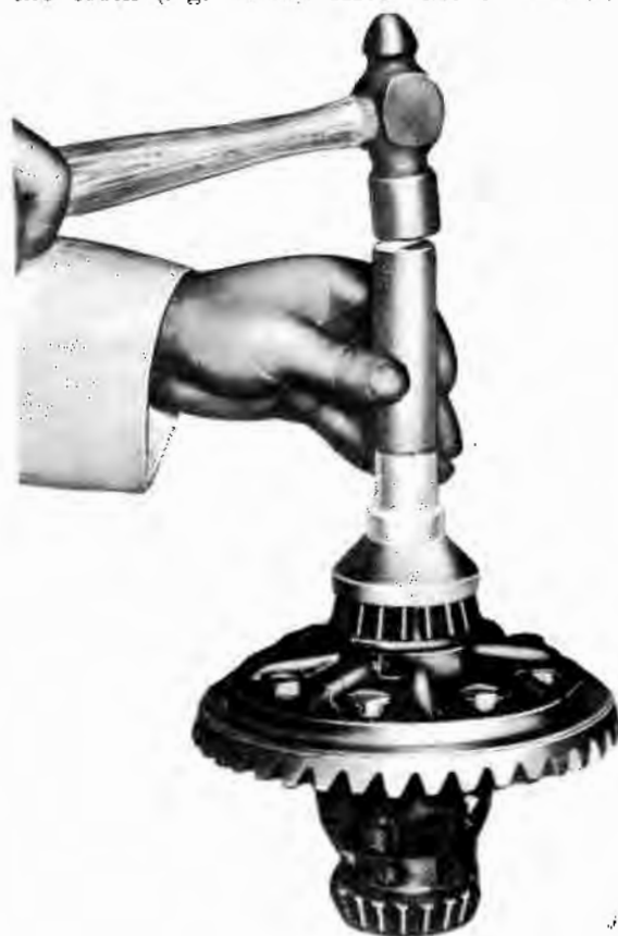
Fig. 10-30 Differential Bearing Driver
