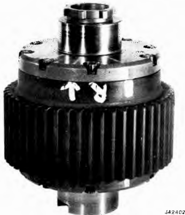
Fig. 8-49 Case Sprocket and End Caps Identified for Orientation
