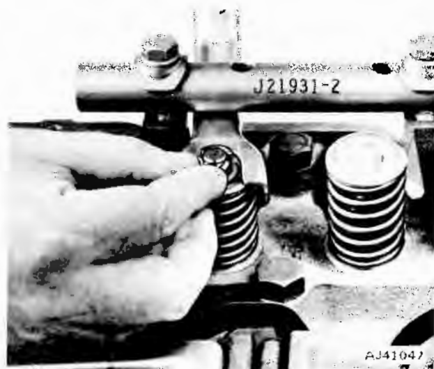
Fig. 1A-10 Valve Spring Removal
