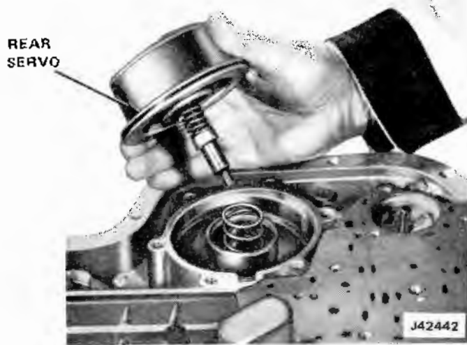
Fig. 7-12 Removing or Installing Rear Servo Assembly
