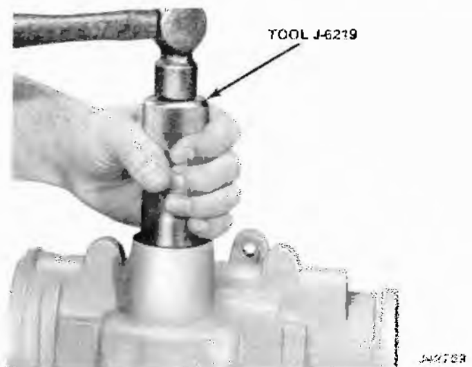
Fig. 11-78 Seating Pitman Shaft Seal in Housing
