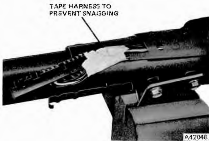
Fig. 11-8 Steering Column Harness Removal
