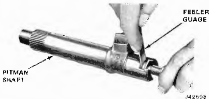
Fig. 11-38 Checking Lash Adjuster End Play
