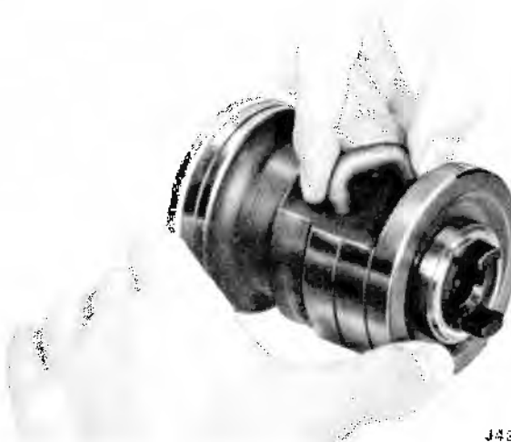
Fig. 11-76 Installing Ball Return Guides in Rack-Piston Nut
