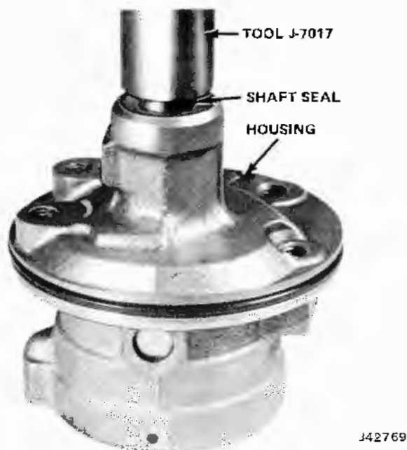
Fig. 11-91 Installing Pump Shaft Seal
