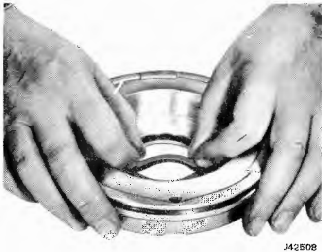
Fig. 7-78 Installing Inner Seal on Direct Clutch Piston
