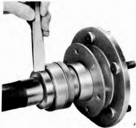
Fig. 10-15 Notching Bearing Retainer Ring
