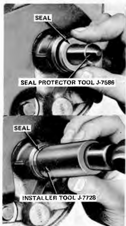
Fig. 11-87 Installing Oil Pump Shaft Seal
