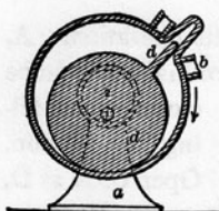
542. "COCHRANE" ROTARY PUMP.—A slide pocket in the outer shell receives the piston wing of the inner eccentric cylinder, which swings in contact with the shell on its centre, 2, carried around by a cam crank.
