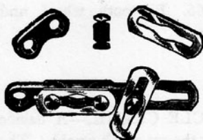
872. DETACHABLE LINK CHAIN for bicycles. The pin can be slipped out by drawing the links together. The grooves in the pins lock in the narrow slot ends of the links.
