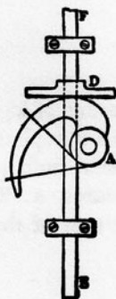
1077. WIPER CAM for stamp mills. A, the wiper; D, flanged chock, allowing the hammer spindle to revolve. Also in use on sewing-machines for throwing the needle bar
