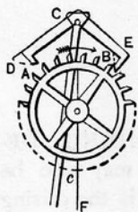
1171. DEAD-BEAT CLOCK ESCAPEMENT.—The face of teeth is slightly pitched forward. The stop-faces of the pallets A, B are concentric with the axis, which gives the dead-beat stop.
