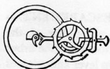
1183. ANCHOR AND LEVER ESCAPEMENT for watches. "Reed's" patent.
