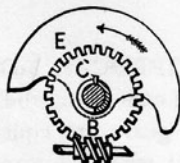
920. RELEASE CAM.—Uniform motion is communicated to the gear wheel, B, fixed on its shaft with a pin at C. The cam is loose on the shaft, with a stop section to meet the pin at C. The lever d has a spring and a roller on the cam. The lever d is raised by the motion of the cam until its straight face reaches the roller, when the lever falls suddenly, throwing the cam forward.
