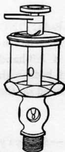
1386. SIGHT-FEED LUBRICATOR.—The amount of feed is seen by the frequency of drops at the sight hole. Adjusted by a needle-point valve with milled head and screw.
