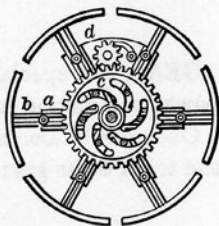
934. EXPANDING PULLEY.—The sectional rim pieces with their arms have a radial sliding joint on the hub arms, and are moved out or in by pins projecting into the spiral slots on the central spur-gear wheel. The movement of the wheel c , by turning the ratchet pinion d , moves all the sections of the pulley equally.
