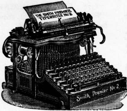
1582. TYPEWRITING MACHINE, "Smith" Premier model. Eighty-four characters.
