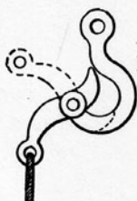
810. BOAT DETACHING HOOK.—The standard is fastened to the boat. A tongue is pivoted to its upper end and passes through the hook of the tackle-block. A lever with an eye to catch the tongue is pivoted to the upright standard, with a lanyard attached at the bottom. A simultaneous pulling of the two lanyards detaches both ends of a boat at once.
