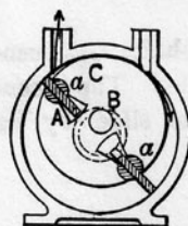
336. "SMITH" ROTARY ENGINE.—Four arms with cylindrical sectors are rotated around an axis central to a perforated cylindrical shell. The driven shaft and head discs are eccentric to the shell. The pressure of steam between the wings tends to push them apart, by which the differential leverage on the disc pins revolves the disc and shaft.
