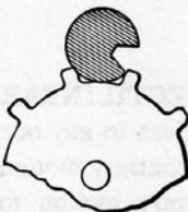
1059. INTERMITTENT MOTION of a toothed wheel by the revolution of a pinion with a single recessed tooth.
