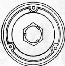
1308. MULTIPLE PLATE FRICTION CLUTCH.—Several plates of iron or steel are fitted loosely on a three-feather shaft, between which plates of wood or other hard material, sometimes steel, are placed and keyed in an iron housing or coupling to move loosely on the keys. The coupling is keyed to the next shaft in
