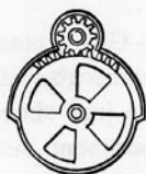
1615. DISC VALVE, for large gas pipes. The disc is revolved by a pinion meshed in a sector gear on the disc.
