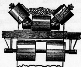
1224. BELT CONVEYOR.—A series of horizontal and inclined rollers serve to turn up the edges of a belt, enabling the material carried to be retained on the belt; the belt returning on the horizontal rollers below.
